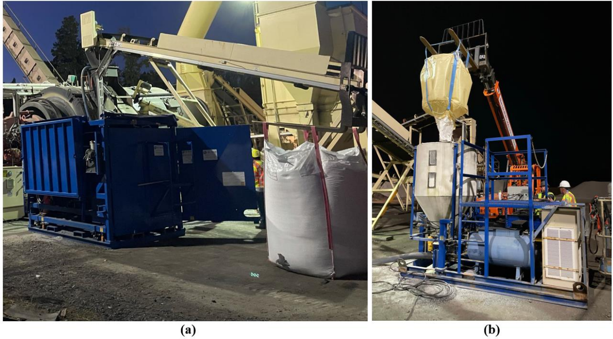
Figure 2. Photographs Taken of Feeder Machines Used for Recycled Plastic Products: (a) P1; (b) P2
