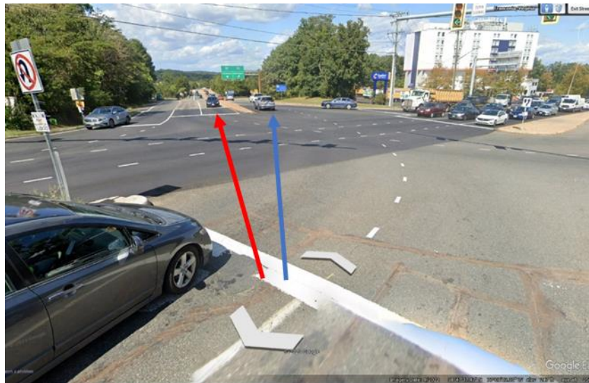
Figure 8. Satellite Image (top) and Google Streetview Image (bottom) of Wrong-Way Driving Rank #1 Ramp I-95S 173A (trumpet) (Google Street View). Blue (right) Arrow Indicates Right Way; Red (left) Arrow Indicates Wrong-Way Driving Maneuvers
