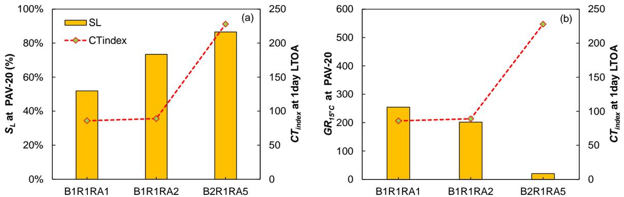
**Figure 48. Comparison of  $CT_{index}$  at 1-day LTOA of Selected Asphalt Mixtures With Parameters of Corresponding Binder Blends Under PAV-20 Aging Conditions: (a)  $S_L$ ; (b)  $GR_{15^\circ C}$ . B = virgin binder; R = reclaimed asphalt pavement (RAP); RA = recycling agent; PAV = pressure aging vessel; PAV-20 = PAV for a duration of 20 hours; CT = cracking tolerance, LTOA = long-term oven aging.**
