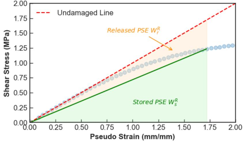
**Figure H12. Linear Amplitude Sweep–Based Pseudo-Strain Energy Definitions.** The undamaged line presents the linear viscoelastic response of the binder to serve as a reference as if no damage took place with increasing loading. The blue dotted line represents the measured response, which shows deviation from the undamaged line as loading progresses, indicating the occurrence of damage.
