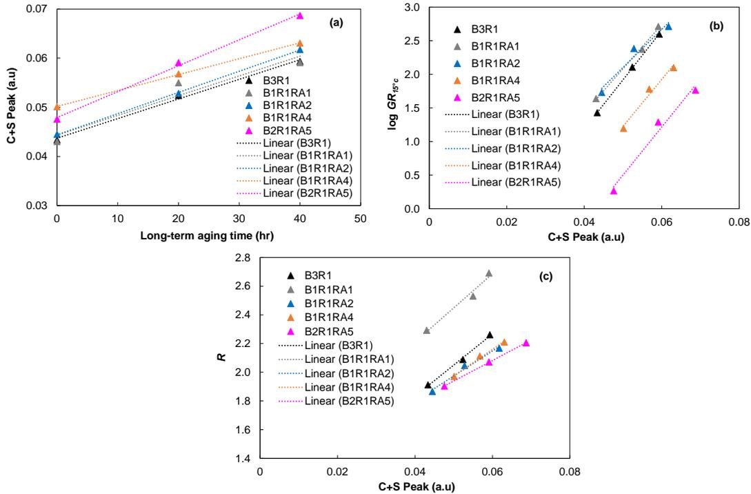
**Figure I9. FTIR Data for a Subset of Source 1 Blends: (a) changes of C+S with respect to aging time; (b) change of log GR<sub>25°C</sub> with respect to C+S; (c) change of R with respect to C+S. FTIR = Fourier transform infrared spectroscopy; B = virgin asphalt binder; R = reclaimed asphalt pavement (RAP) binder; RA = recycling agent; C = carbonyl; S = sulfoxide; GR = Glover-Rowe parameter; R = rheological index.**
