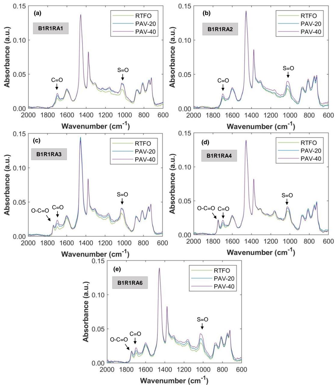
**Figure I2. FTIR Spectra for B1R1 Blends: (a) B1R1RA1; (b) B1R1RA2; (c) B1R1RA3; (d) B1R1RA4; (e) B1R1RA6. FTIR = Fourier transform infrared spectroscopy; B = virgin asphalt binder; R = reclaimed asphalt pavement binder; RA = recycling agent; RTFO = rolling thin film oven (short-term aging); PAV = pressure aging vessel; PAV-20 = aging in PAV for 20 hours; PAV-40 = aging in PAV for 40 hours.**
