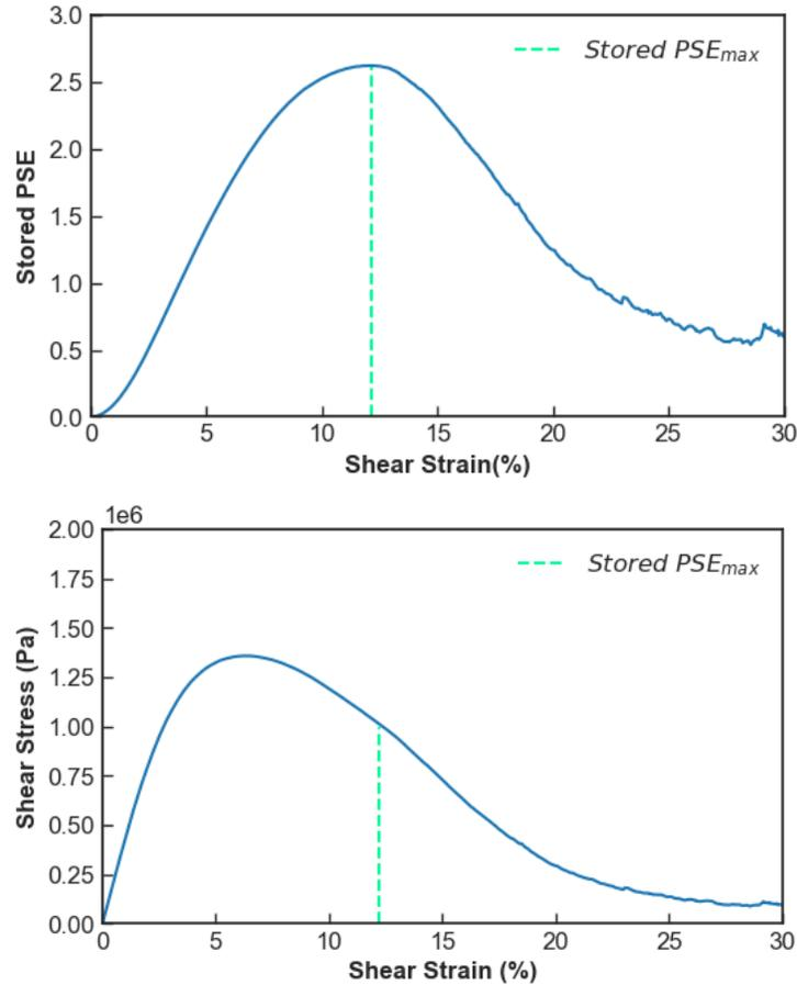
**Figure H13. Schematic for Peak Stored PSE and the Corresponding Shear Stress. PSE = pseud-strain energy.**
