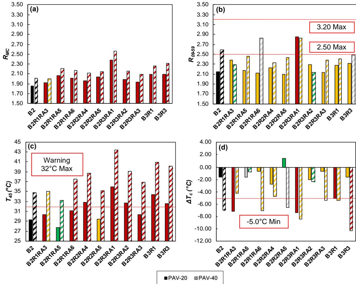
Figure 21. Rheological Balance Parameters (a)  $R_{MC}$ ; (b)  $R_{09-59}$ ; (c)  $T_{45}$ ; (d)  $\Delta T_c$ . Colors correspond to performance; black is target, green is better performance, yellow is equal performance, red is worse performance, and gray is removed. B = virgin asphalt binder; R = reclaimed asphalt pavement (RAP); RA = recycling agent.
