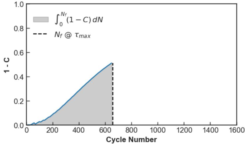
Figure H3. Schematic for the Calculation of  $I^R$
