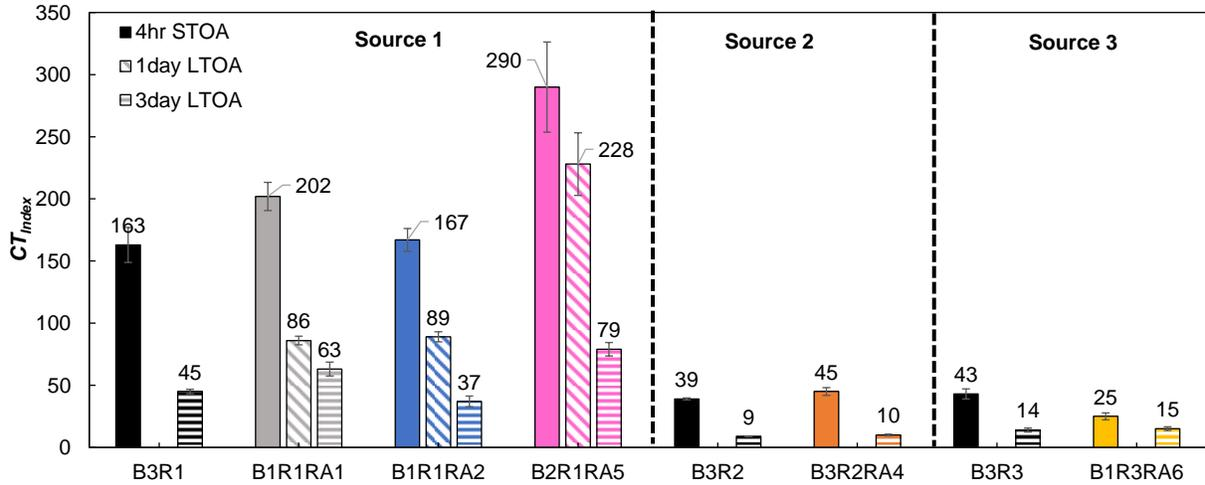
**Figure 45. Performance Test Data for IDT-CT of Source 1, 2, and 3 Mixtures Under Different Aging Conditions.** I-bars indicate CT index variability  $\pm 1$  standard deviation. IDT-CT = indirect tensile cracking test; CT = cracking tolerance; STOA = short-term oven aging; LTOA = long-term oven aging; B = virgin binder; R = reclaimed asphalt pavement (RAP); RA = recycling agent.
