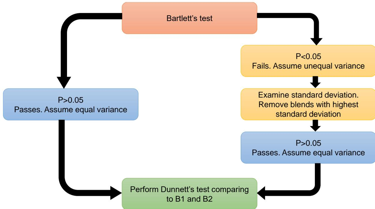
Figure 3. Flowchart of the Statistical Grouping Analysis. P = p-value; B = virgin asphalt binder.
