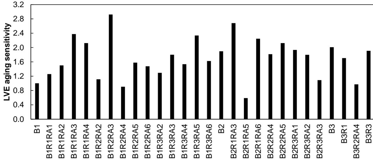
Figure H2. LVE Aging Sensitivity for All Evaluated Binder Blends. LVE = linear viscoelastic; B = virgin asphalt binder; R = reclaimed asphalt pavement (RAP) binder; RA = recycling agent.
