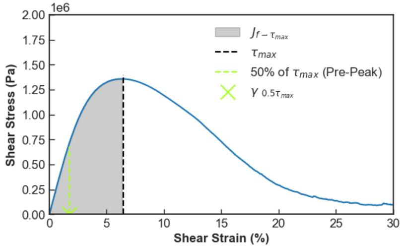
Figure H8. Schematic for the Calculation of FREI. FREI = fatigue resistance energy index.
