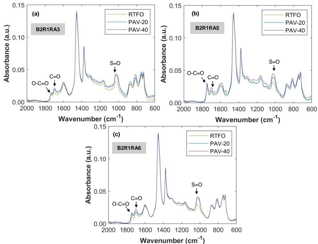
Figure I5. FTIR Spectra for B2R1 Blends: (a) B2R1RA3; (b) B2R1RA5; (c) B2R1RA6. FTIR = Fourier transform infrared spectroscopy; B = virgin asphalt binder; R = reclaimed asphalt pavement (RAP) binder; RA = recycling agent; RTFO = rolling thin film oven (short-term aging); PAV = pressure aging vessel; PAV-20 = aging in PAV for 20 hours; PAV-40 = aging in PAV for 40 hours.
