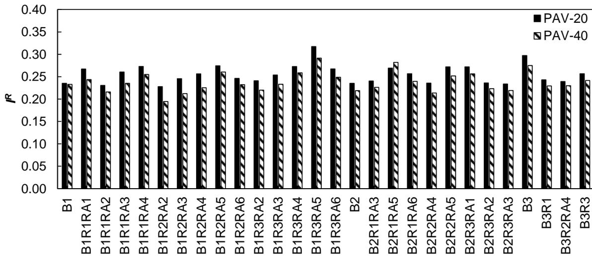
Figure H4. Average Reduction in Integrity Up to Failure ( $I^R$ ) for All Evaluated Binder Blends Under PAV-20 and PAV-40 Aging Conditions. B = virgin asphalt binder; R = reclaimed asphalt pavement (RAP) binder; RA = recycling agent; PAV = pressure aging vessel; PAV-20 = PAV for a duration of 20 hours; PAV-40 = PAV for a duration of 40 hours.
