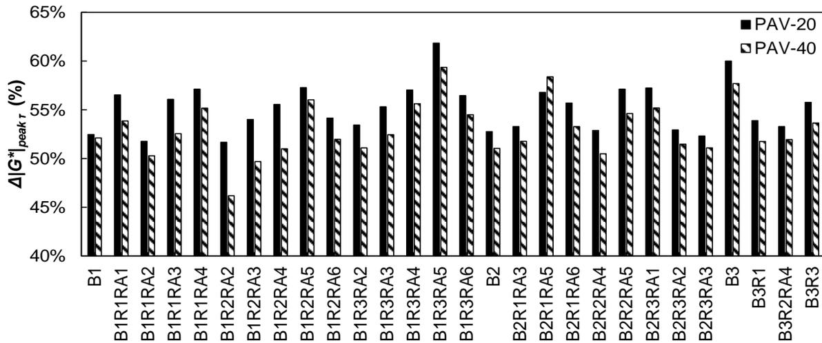
**Figure H11.  $\Delta|G^*|_{peak \tau}$  for All Evaluated Binder Blends Under PAV-20 and PAV-40 Aging Conditions.** PAV = pressure aging vessel; PAV-20 = PAV for a duration of 20 hours; PAV-40 = PAV for a duration of 40 hours; B = virgin asphalt binder; R = reclaimed asphalt pavement (RAP) binder; RA = recycling agent.
