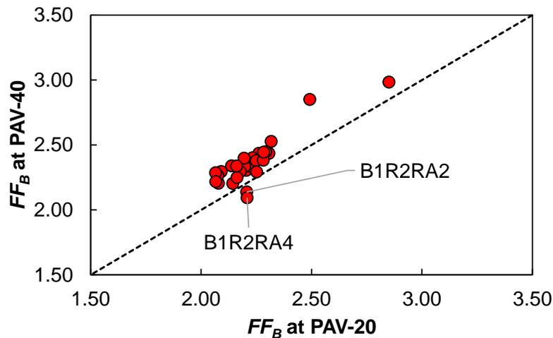
**Figure H10. Comparison of FF<sub>B</sub> for All Evaluated Binder Blends Under PAV-20 and PAV-40 Aging Conditions.** PAV = pressure aging vessel; PAV-20 = PAV for a duration of 20 hours; PAV-40 = PAV for a duration of 40 hours; B = virgin asphalt binder; R = reclaimed asphalt pavement (RAP) binder; RA = recycling agent.
