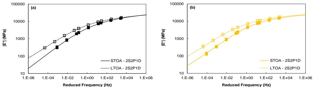
**Figure 43. Dynamic Modulus  $|E^*|$  Master Curves for Two Source 3 Mixtures at STOA and LTOA Conditions: (a) B3R3; (b) B1R3RA6. STOA = short-term oven aging; LTOA = long-term oven aging;  $|E^*|$  = dynamic modulus; B = virgin binder; R = reclaimed asphalt pavement (RAP); RA = recycling agent.**
