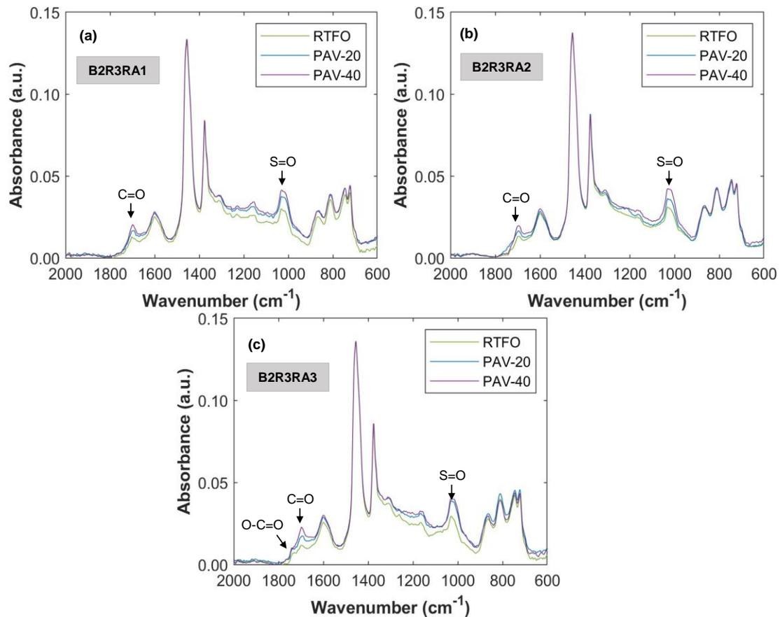
**Figure 17. FTIR Spectra for B2R3 Blends: (a) B2R3RA1; (b) B2R3RA2; (c) B2R3RA3. FTIR = Fourier transform infrared spectroscopy; B = virgin asphalt binder; R = reclaimed asphalt pavement (RAP) binder; RA = recycling agent; RTFO = rolling thin film oven (short-term aging); PAV = pressure aging vessel; PAV-20 = aging in PAV for 20 hours; PAV-40 = aging in PAV for 40 hours.**
