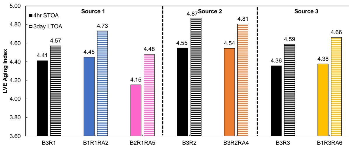
**Figure 44. LVE Aging Index for Source 1, 2, and 3 Mixtures at STOA and LTOA Conditions.** STOA = short-term oven aging; LTOA = long-term oven aging; LVE = linear viscoelastic; B = virgin binder; R = reclaimed asphalt pavement (RAP); RA = recycling agent.
