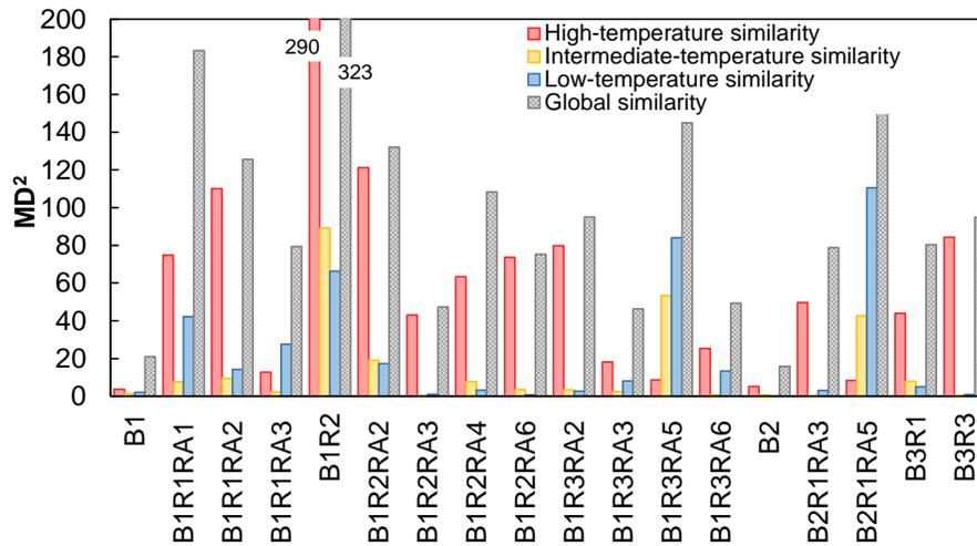
Figure 14. Similarity Analysis Results for Virginia’s Binder Blends. MD = Mahalanobis distance; B = virgin asphalt binder; R = reclaimed asphalt pavement (RAP) binder; RA = recycling agent.
