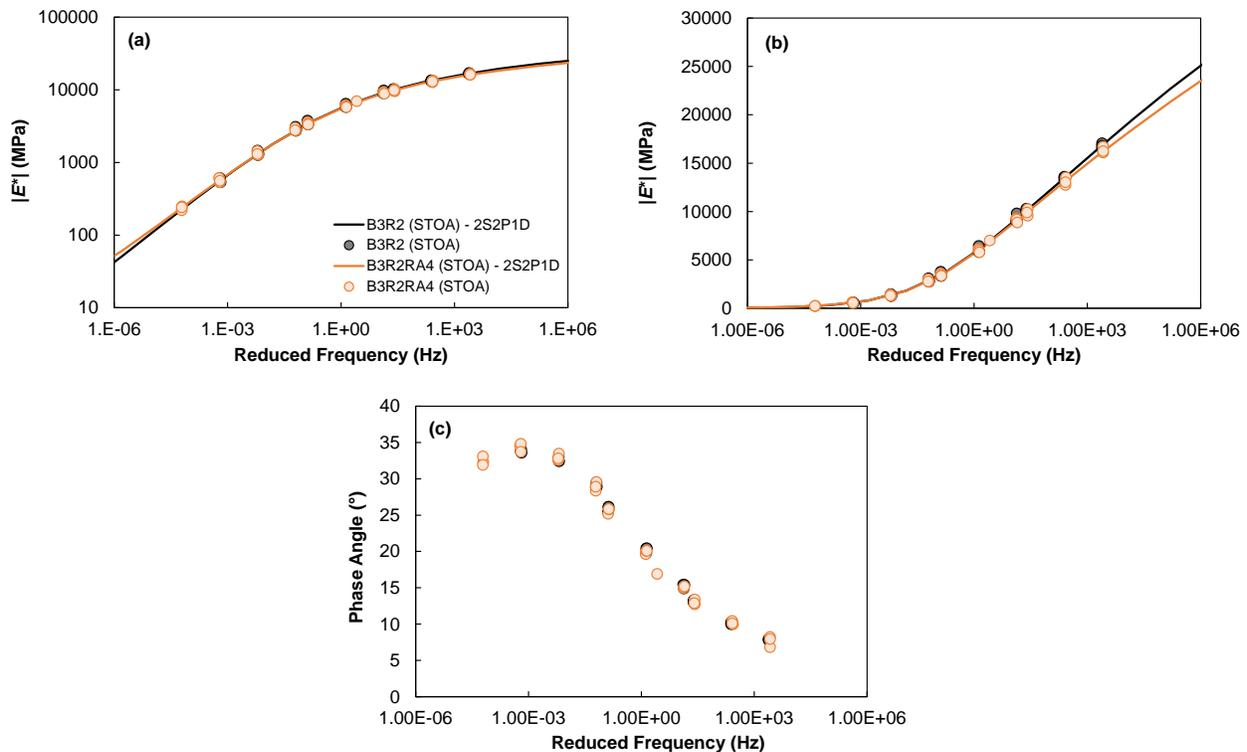
Figure 33. Linear Viscoelastic Characterization of Source 2 Mixtures: (a) dynamic modulus in logarithmic space; (b) dynamic modulus in semi-logarithmic space; (c) phase angle.  $|E^*|$  = dynamic modulus; B = virgin binder; R = reclaimed asphalt pavement (RAP); RA = recycling agent.
