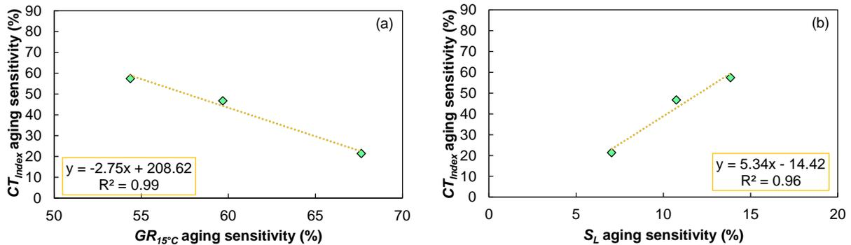
**Figure 50. Cross-Scale Correlation Between 1-day  $CT_{index}$  Aging Sensitivity and Binder Aging Sensitives: (a)  $GR_{15^\circ C}$ ; (b)  $S_L$ .  $CT$  = cracking tolerance,  $GR$  = Glover-Rowe;  $S_L$  = stress level at peak stored pseudo-strain energy.**
