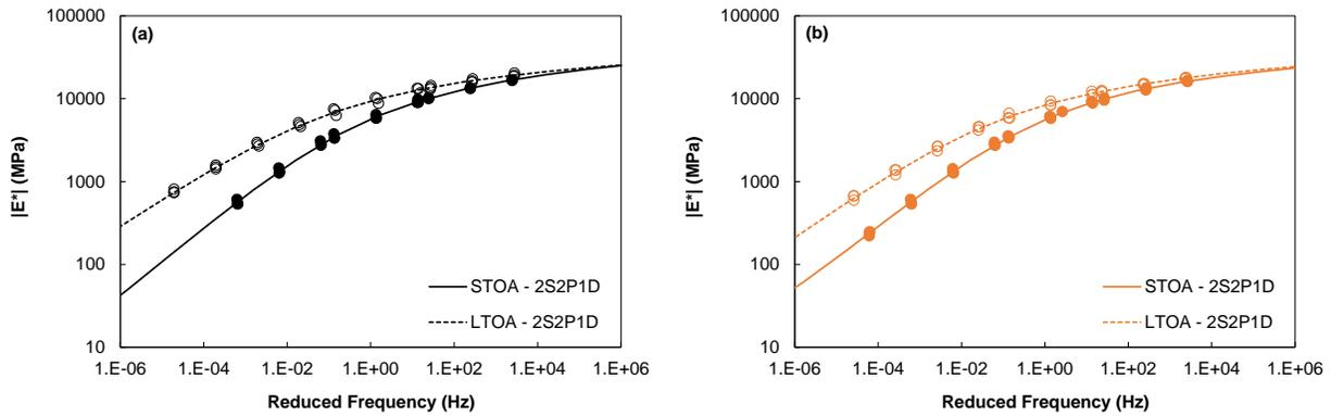
**Figure 42. Dynamic Modulus  $|E^*|$  Master Curves for Two Source 2 Mixtures at STOA and LTOA Conditions: (a) B3R2; (b) B3R2RA4. STOA = short-term oven aging; LTOA = long-term oven aging;  $|E^*|$  = dynamic modulus; B = virgin binder; R = reclaimed asphalt pavement (RAP); RA = recycling agent.**
