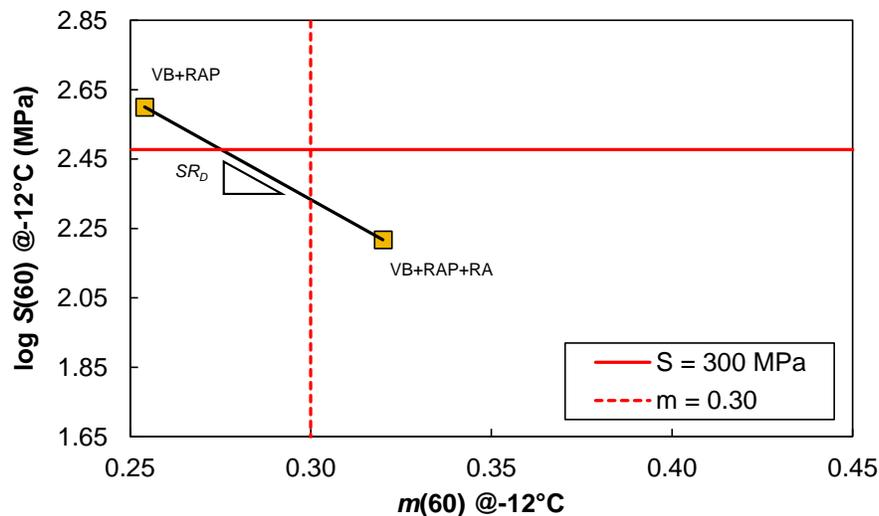
Figure 16. Graphical Representation of the  $SR_D$  Parameter. VB = virgin binder; RAP = reclaimed asphalt pavement; RA = recycling agent.
