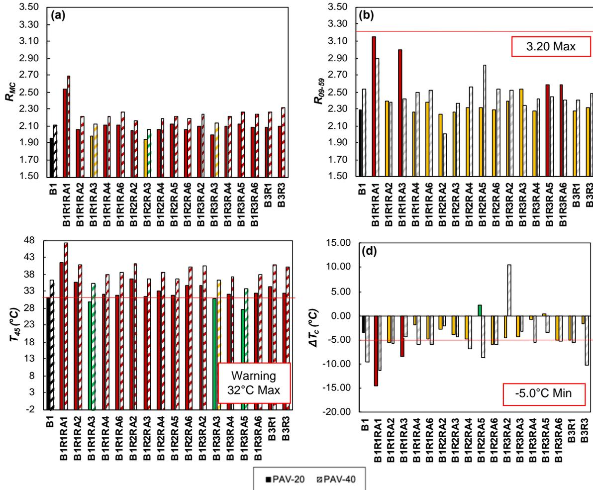
Figure G3. Rheological Balance Parameters: (a)  $R_{MC}$ ; (b)  $R_{09-59}$ ; (c)  $T_{45}$ ; (d)  $\Delta T_c$ . Colors correspond to performance; black is target, green is better performance, yellow is equal performance, red is worse performance, gray is removed. B = virgin asphalt binder; R = reclaimed asphalt pavement (RAP); RA = recycling agent.
