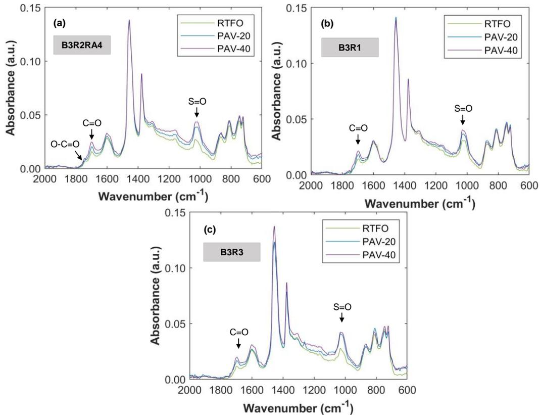
**Figure 28. FTIR Spectra for B3 Blends: (a) B3R2RA4; (b) B3R1; (c) B3R3. FTIR = Fourier transform infrared spectroscopy; B = virgin asphalt binder; R = reclaimed asphalt pavement (RAP) binder; RA = recycling agent; RTFO = rolling thin film oven (short-term aging); PAV = pressure aging vessel; PAV-20 = aging in PAV for 20 hours; PAV-40 = aging in PAV for 40 hours.**
