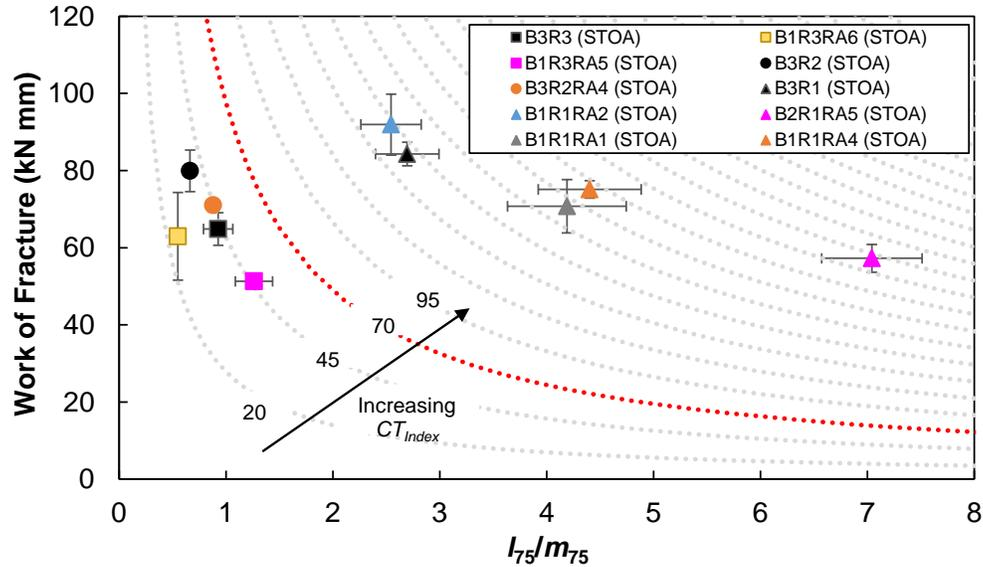
Figure 36. IDT-CT Interaction Diagram of Source 1, 2, and 3 Mixtures. I-bars indicate parameter variability  $\pm 1$  standard deviation. IDT-CT = indirect tensile cracking test; CT = cracking tolerance; B = virgin binder; R = reclaimed asphalt pavement (RAP); RA = recycling agent. Red dashed line = balanced mix design special provision limit for surface asphalt mixtures with A and D designations.
