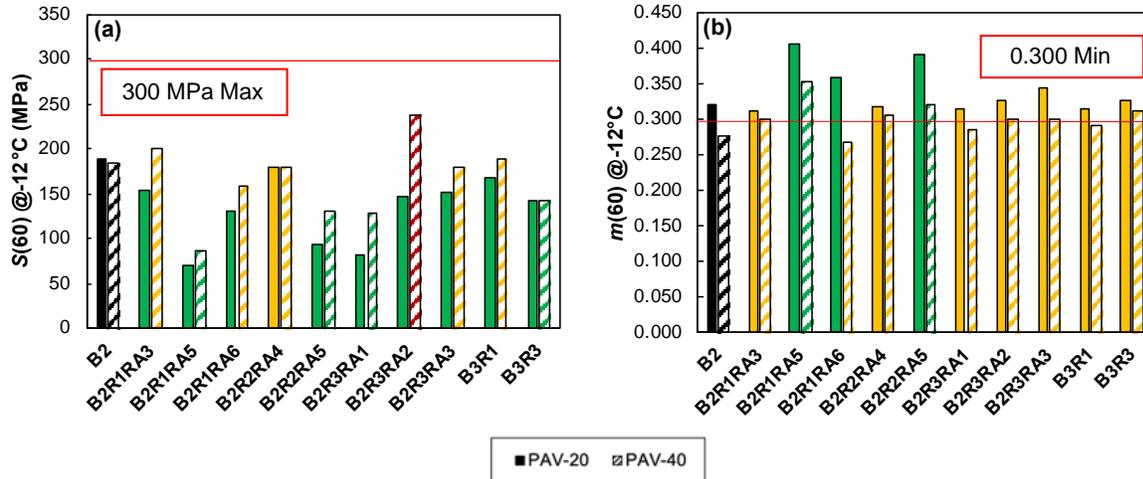
Figure 19. Low-Temperature Point Parameters: (a) stiffness  $S(60)$ ; (b) coefficient of relaxation  $m(60)$ . Colors convey Dunnett's test results: green, yellow, and red indicate better, equal, and worse results relative to B2, respectively. Gray indicates that the blend could not be compared statistically to B2 using Dunnett's test because its variance differed from B2 and thus failed. B = virgin asphalt binder; R = reclaimed asphalt pavement (RAP); RA = recycling agent.
