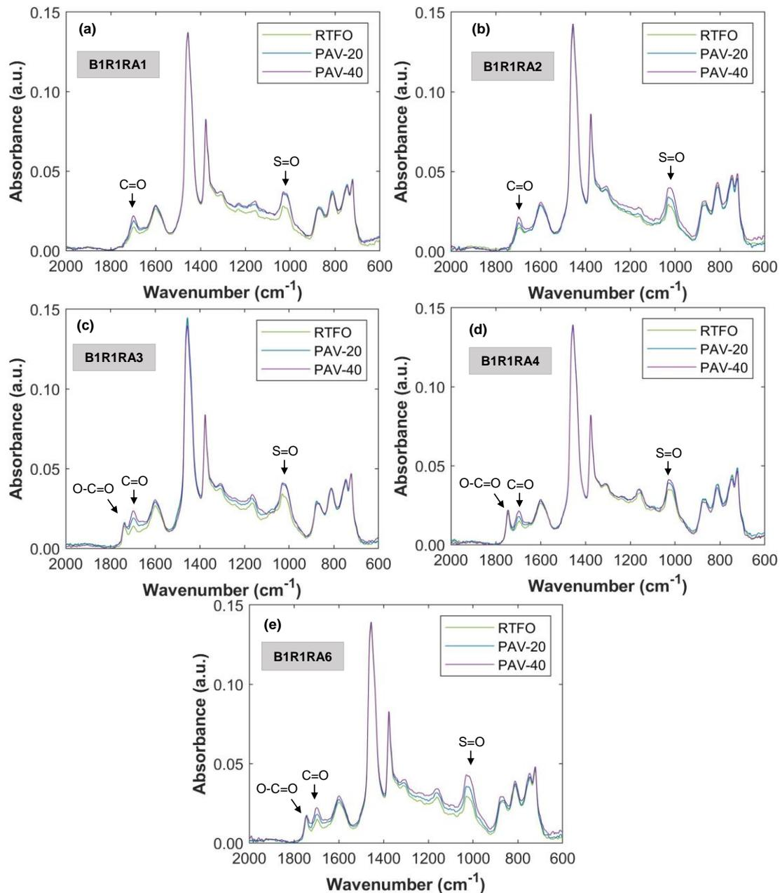
**Figure 26. FTIR Spectra for B1R1 Blends: (a) B1R1RA1; (b) B1R1RA2; (c) B1R1RA3; (d) B1R1RA4; (e) B1R1RA6. FTIR = Fourier transform infrared spectroscopy; B = virgin asphalt binder; R = reclaimed asphalt pavement (RAP) binder; RA = recycling agent; RTFO = rolling thin film oven (short-term aging); PAV = pressure aging vessel; PAV-20 = aging in PAV for 20 hours; PAV-40 = aging in PAV for 40 hours.**
