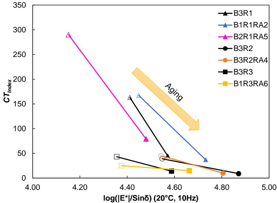
Figure 47. Relationship Between  $CT_{index}$  and LVE Aging Index for Source 1, 2, and 3 Mixtures Under Different Aging Conditions. Open shapes indicate 4-hour short-term oven aging; filled shapes indicate 3-day long-term oven aging at 95°C in addition to short-term oven aging. CT = cracking tolerance;  $|E^*|$  = dynamic modulus; B = virgin binder; R = reclaimed asphalt pavement (RAP); RA = recycling agent.
