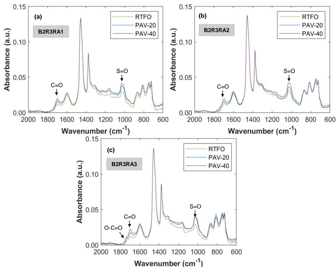
**Figure 27. FTIR Spectra for B2R3 Blends: (a) B2R3RA1; (b) B2R3RA2; (c) B2R3RA3. FTIR = Fourier transform infrared spectroscopy; B = virgin asphalt binder; R = reclaimed asphalt pavement (RAP) binder; RA = recycling agent; RTFO = rolling thin film oven (short-term aging); PAV = pressure aging vessel; PAV-20 = aging in PAV for 20 hours; PAV-40 = aging in PAV for 40 hours.**
