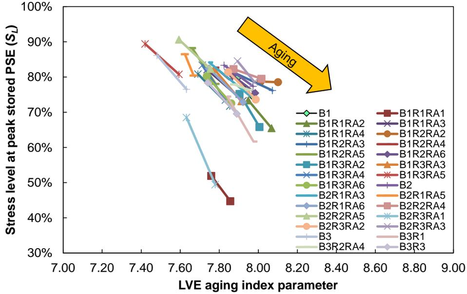
Figure H15. Comparison of  $S_L$  With LVE Aging Index Parameter for All Evaluated Binder Blends Under PAV-20 and PAV-40 Aging Conditions. LVE = linear viscoelastic; PAV = pressure aging vessel; PAV-20 = PAV for a duration of 20 hours; PAV-40 = PAV for a duration of 40 hours; B = virgin asphalt binder; R = reclaimed asphalt pavement (RAP) binder; RA = recycling agent.
