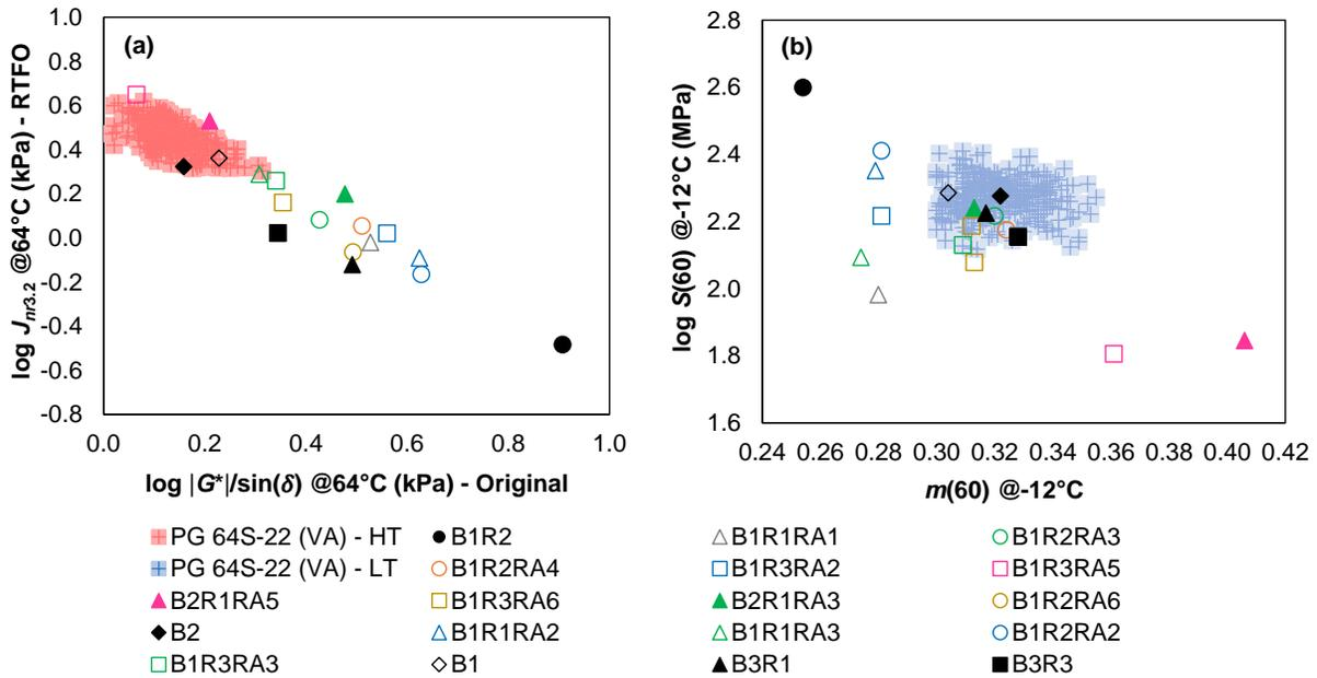
**Figure 11. Bivariate Distribution of High- and Low-Temperature Rheological Properties of Virginia's Materials: (a) AASHTO M 322 high-temperature rheological space; (b) AASHTO M 332 low-temperature rheological space. B = virgin asphalt binder; R = reclaimed asphalt pavement (RAP) binder; RA = recycling agent; PG = performance grade; S = standard traffic.**
