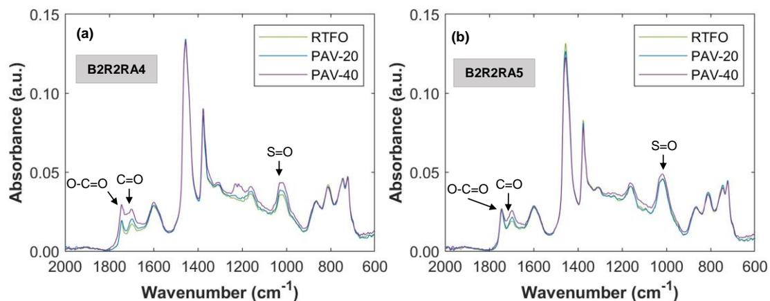
Figure I6. FTIR Spectra for B2R2 Blends: (a) B2R2RA4; (b) B2R2RA5. FTIR = Fourier transform infrared spectroscopy; B = virgin asphalt binder; R = reclaimed asphalt pavement (RAP) binder; RA = recycling agent; RTFO = rolling thin film oven (short-term aging); PAV = pressure aging vessel; PAV-20 = aging in PAV for 20 hours; PAV-40 = aging in PAV for 40 hours.
