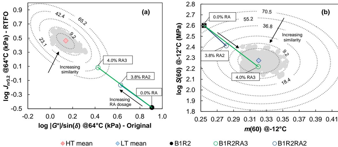
**Figure 12. Relationship Between RA Dosage and Similarity for B1R2RA3 and B1R2RA2: (a) high-temperature rheological space; (b) low-temperature rheological space. B = virgin asphalt binder; R = reclaimed asphalt pavement (RAP) binder; RA = recycling agent; RTFO = rolling thin film oven; HT = high temperature; LT = low temperature.**
