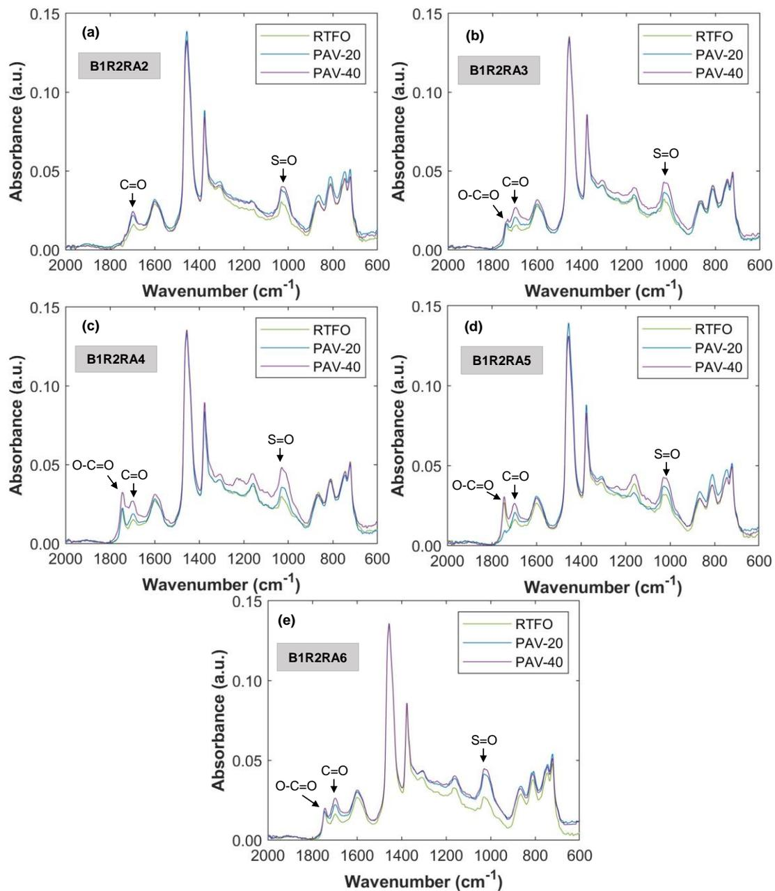
Figure I3. FTIR Spectra for B1R2 Blends: (a) B1R2RA2; (b) B1R2RA3; (c) B1R2RA4; (d) B1R2RA5; (e) B1R2RA6. FTIR = Fourier transform infrared spectroscopy; B = virgin asphalt binder; R = reclaimed asphalt pavement (RAP) binder; RA = recycling agent; RTFO = rolling thin film oven (short-term aging); PAV = pressure aging vessel; PAV-20 = aging in PAV for 20 hours; PAV-40 = aging in PAV for 40 hours.
