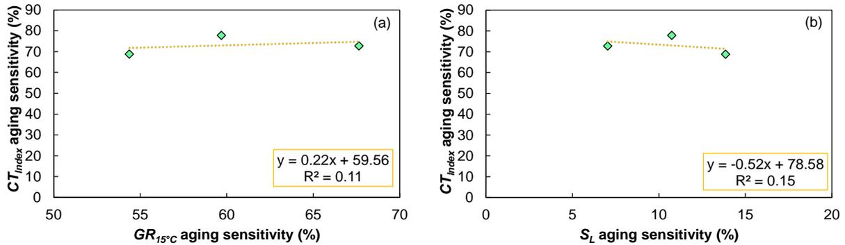
Figure 51. Cross-Scale Correlation Between 3-day  $CT_{index}$  Aging Sensitivity and Binder Aging Sensitives: (a)  $GR_{15^\circ C}$ ; (b)  $S_L$ .  $CT$  = cracking tolerance,  $GR$  = Glover-Rowe;  $S_L$  = stress level at peak stored pseudo-strain energy.
