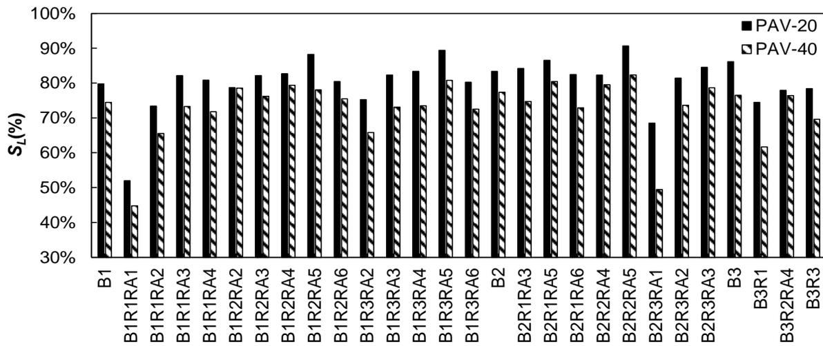
Figure 25.  $S_L$  for All Evaluated Binder Blends Under PAV-20 and PAV-40 Aging Conditions. B = virgin asphalt binder; R = reclaimed asphalt pavement (RAP) binder; RA = recycling agent; PAV = pressure aging vessel; PAV-20 = PAV for a duration of 20 hours; PAV-40 = PAV for a duration of 40 hours.
