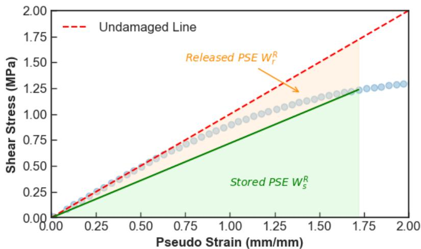
**Figure 23. Liner Amplitude Sweep-Based Pseudo-Strain Energy Definitions.** The undamaged line presents the LVE response of the binder to serve as a reference as if no damage took place with increasing loading. The blue dotted line represents the measured response, which shows deviation from the undamaged line as loading progresses, indicating the occurrence of damage. LVE = linear viscoelastic.
