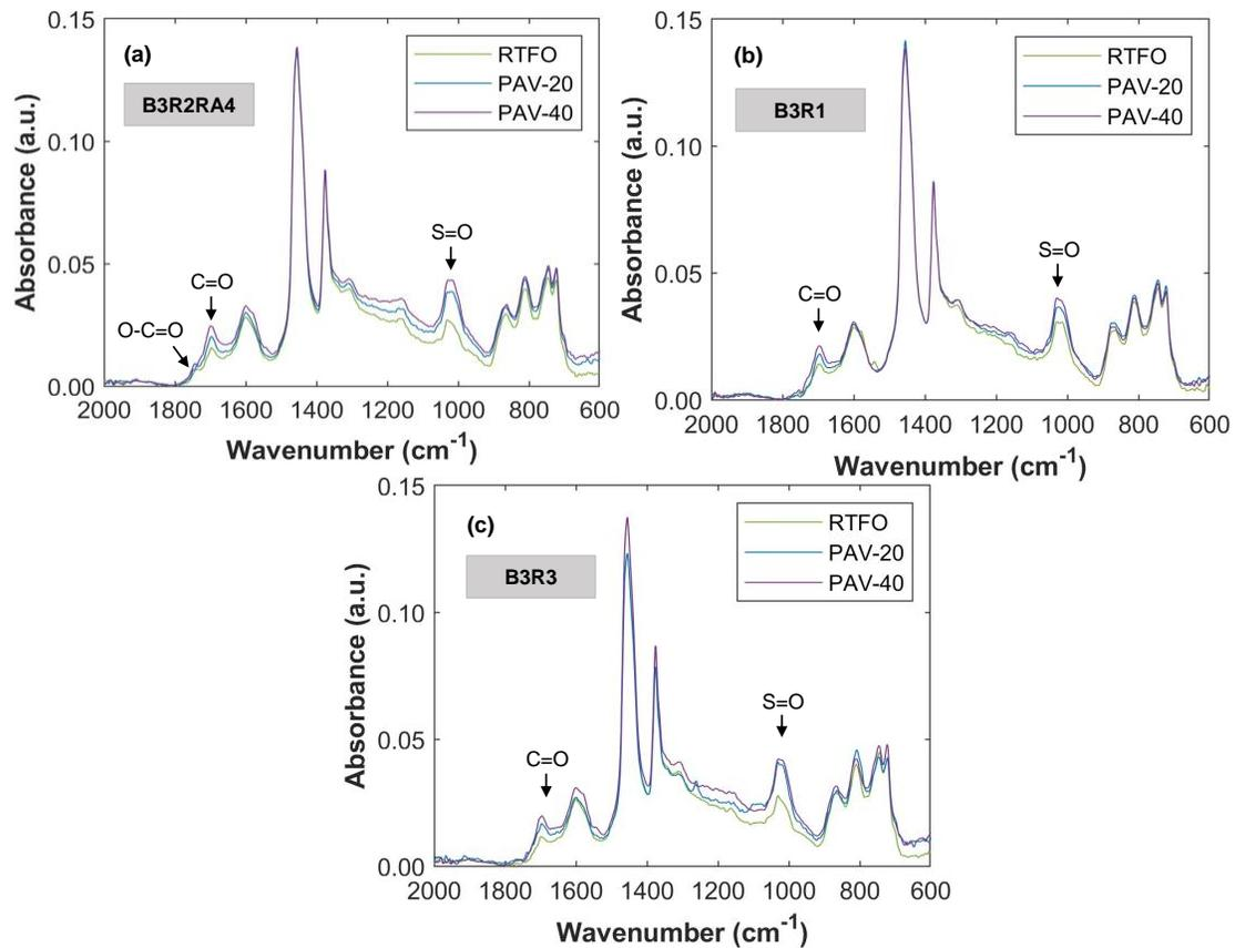
**Figure I8. FTIR Spectra for B3 Blends: (a) B3R2RA4; (b) B3R1; (c) B3R3. FTIR = Fourier transform infrared spectroscopy; B = virgin asphalt binder; R = reclaimed asphalt pavement (RAP) binder; RA = recycling agent; RTFO = rolling thin film oven (short-term aging); PAV = pressure aging vessel; PAV-20 = aging in PAV for 20 hours; PAV-40 = aging in PAV for 40 hours.**
