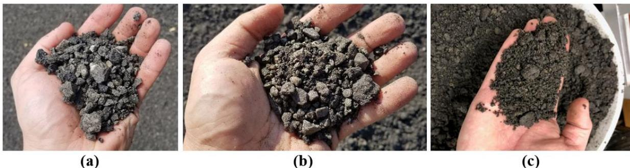
Figure 9. RAP Materials Sampled for This Study: (a) R1 from Salem; (b) R2 from Burkeville; (c) R3 from Chesapeake. RAP = reclaimed asphalt pavement.
