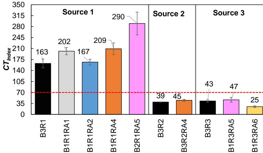
Figure 35. Performance Test Data for the IDT-CT for Source 1, 2, and 3 Mixtures. I-bars indicate CT index variability  $\pm 1$  standard deviation. IDT-CT = indirect tensile cracking test; CT = cracking tolerance; B = virgin binder; R = reclaimed asphalt pavement (RAP); RA = recycling agent. Red dashed line = balanced mix design special provision limit for surface asphalt mixtures with A and D designations.
