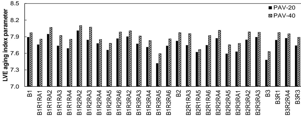
**Figure H1. LVE Aging Index Parameter for All Evaluated Binders Under PAV-20 and PAV-40 Aging Conditions.** LVE = linear viscoelastic; B = virgin asphalt binder; R = reclaimed asphalt pavement (RAP) binder; RA = recycling agent; PAV = pressure aging vessel; PAV-20 = PAV for a duration of 20 hours; PAV-40 = PAV for a duration of 40 hours.
