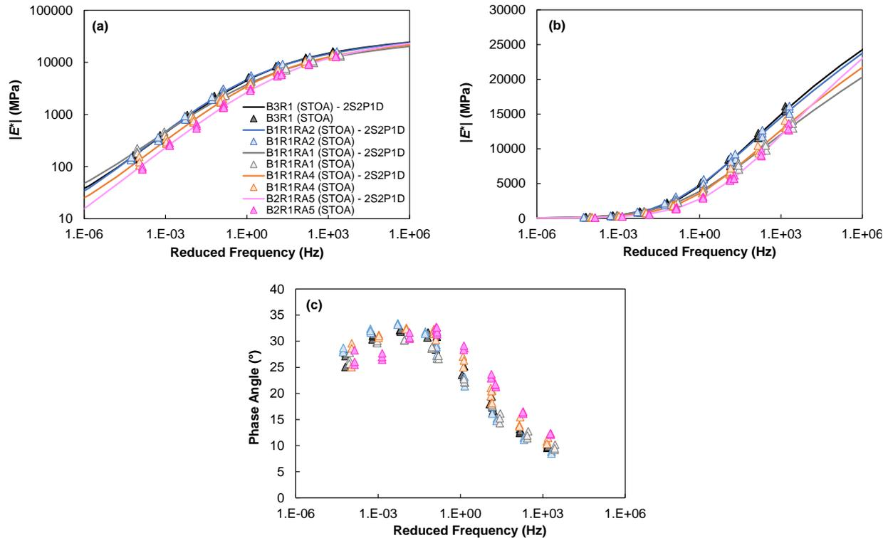
**Figure 32. Linear Viscoelastic Characterization of Source 1 Mixtures: (a) dynamic modulus in logarithmic space; (b) dynamic modulus in semi-logarithmic space; (c) phase angle.  $|E^*|$  = dynamic modulus; B = virgin binder; R = reclaimed asphalt pavement (RAP); RA = recycling agent.**
