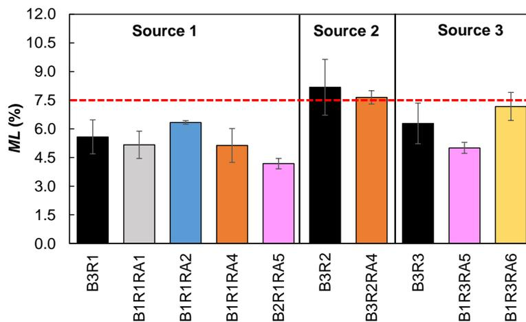
Figure 31. Performance Test Data for Cantabro Mass Loss of Source 1, 2, and 3 Mixtures. I-bars indicate mass loss variability  $\pm 1$  standard deviation. ML = mass loss; B = virgin binder; R = reclaimed asphalt pavement (RAP); RA = recycling agent. Red dashed line = balanced mix design special provision limit for surface asphalt mixtures with A and D designations.
