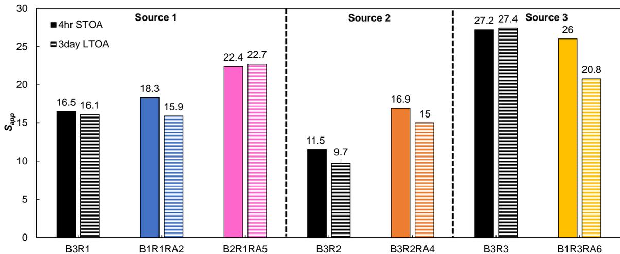
**Figure 46. Cyclic Fatigue Test Data in Terms of  $S_{app}$  Values for Source 1, 2, and 3 Mixtures Under Different Aging Conditions.**  $S_{app}$  = apparent damage capacity; STOA = short-term oven aging; LTOA = long-term oven aging; B = virgin binder; R = reclaimed asphalt pavement (RAP); RA = recycling agent.
