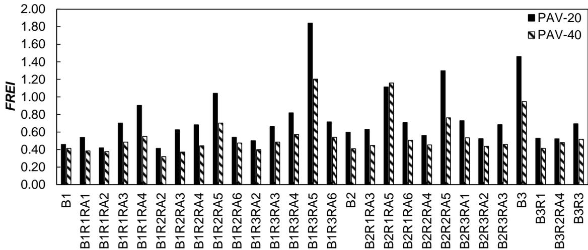
Figure H9. Fatigue Energy Resistance Index (FREI) for All evaluated Binder Blends Under PAV-20 and PAV-40 Aging Conditions. PAV = pressure aging vessel; PAV-20 = PAV for a duration of 20 hours; PAV-40 = PAV for a duration of 40 hours; B = virgin asphalt binder; R = reclaimed asphalt pavement (RAP) binder; RA = recycling agent.
