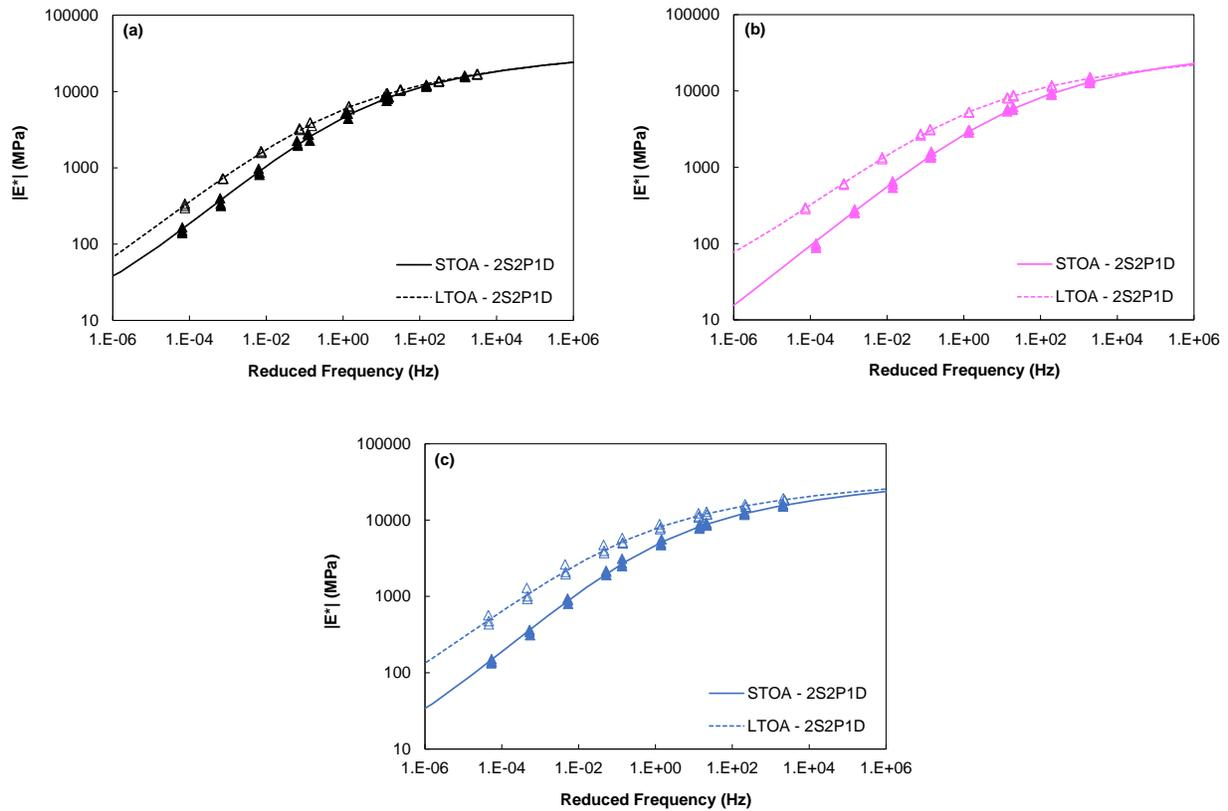
**Figure 41. Dynamic Modulus  $|E^*|$  Master Curves for Three Source 1 Mixtures at STOA and LTOA Conditions: (a) B3R1; (b) B2R1RA5; (c) B1R1R2. STOA = short-term oven aging; LTOA = long-term oven aging;  $|E^*|$  = dynamic modulus; B = virgin binder; R = reclaimed asphalt pavement (RAP); RA = recycling agent.**
