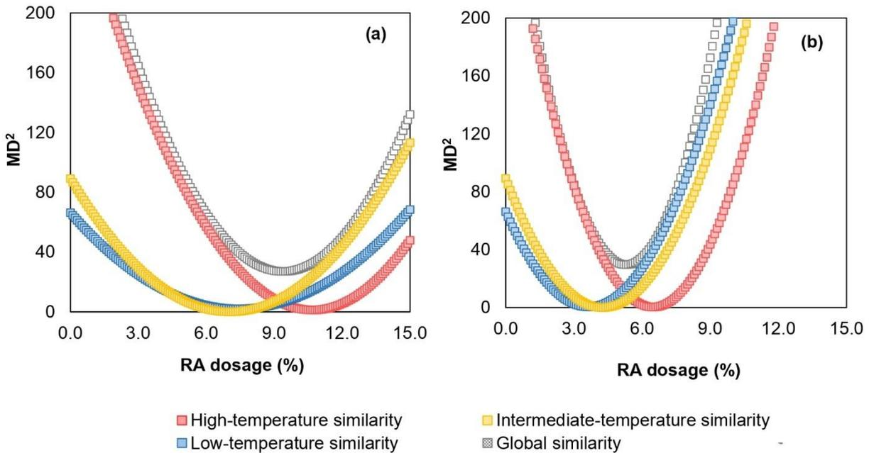
**Figure 13. Statistical Similarity of Recycled Asphalt Blends With RAs to Virginia PG 64S-22 Binders: (a) B1R2RA2; (b) B1R2RA3. MD = Mahalanobis distance; B = virgin asphalt binder; R = reclaimed asphalt pavement (RAP) binder; RA = recycling agent.**
