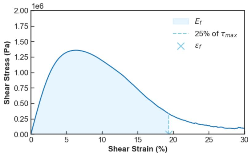
Figure H5. Schematic for the Calculation of  $\epsilon_T$  and  $E_f$
