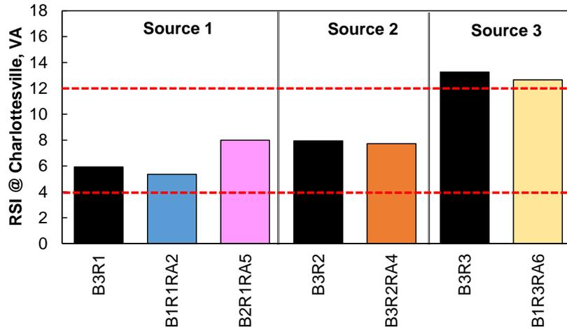
**Figure 40. Performance Test Data for SSR Test of Source 1, 2, and 3 Mixtures Determined Using Charlottesville Climatic Data.** SSR = stress sweep rutting; RSI = rutting strain index; B = virgin binder; R = reclaimed asphalt pavement (RAP); RA = recycling agent. Red dashed lines represent the corresponding range for standard traffic.
