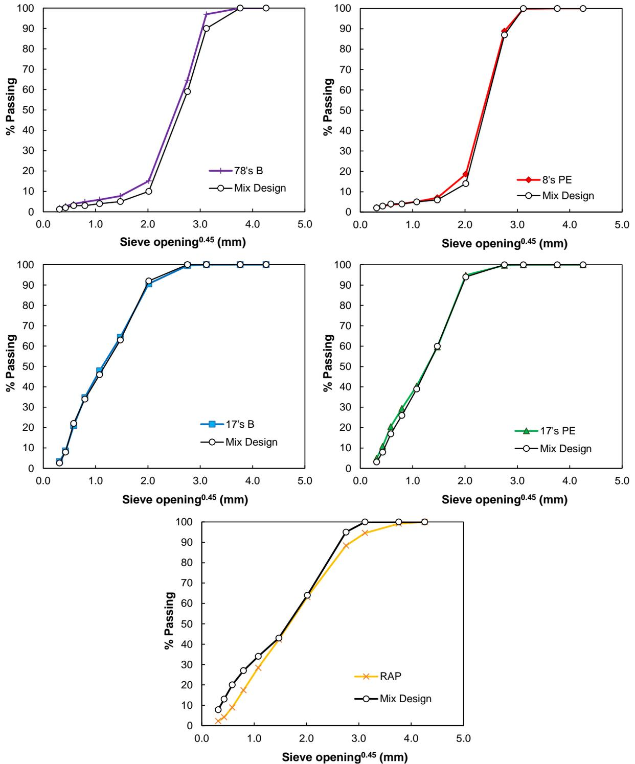
Figure E2. Source 2 Aggregate and RAP Stockpile Gradations. RAP = reclaimed asphalt pavement.
