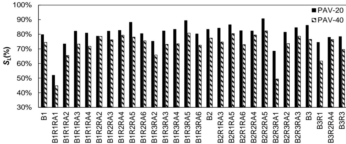
**Figure H14.  $S_L$  for All Evaluated Binder Blends Under PAV-20 and PAV-40 Aging Conditions.** PAV = pressure aging vessel; PAV-20 = PAV for a duration of 20 hours; PAV-40 = PAV for a duration of 40 hours; B = virgin asphalt binder; R = reclaimed asphalt pavement (RAP) binder; RA = recycling agent.
