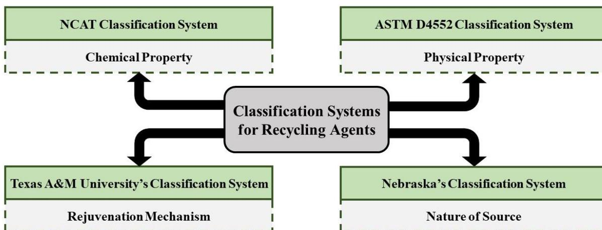
**Figure 5. Basis of Different Classification Systems for Recycling Agents.** NCAT = National Center for Asphalt Technology; ASTM = American Society for Testing and Materials.
