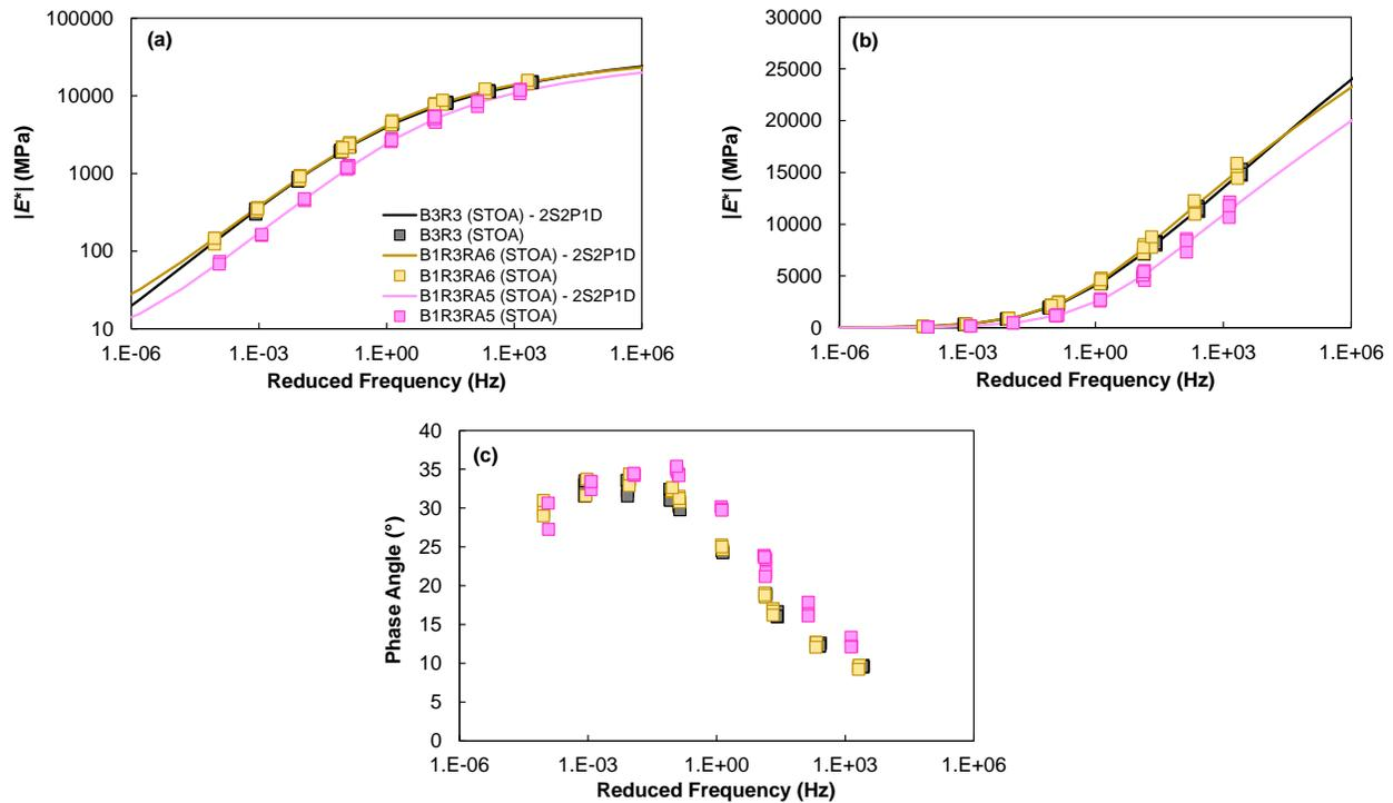
**Figure 34. Linear Viscoelastic Characterization of Source 3 Mixtures: (a) dynamic modulus in logarithmic space; (b) dynamic modulus in semi-logarithmic space; (c) phase angle.  $|E^*|$  = dynamic modulus; B = virgin binder; R = reclaimed asphalt pavement (RAP); RA = recycling agent.**
