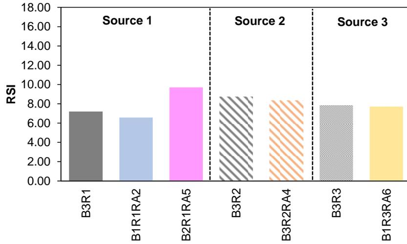
**Figure L2. RSI Results for Source 1, 2, and 3 Mixtures Calculated Using the Specific Climatic Data (Source 1 = Blacksburg, Virginia; Source 2 = Mecklenburg, Virginia; and Source 3= Chesapeake, Virginia). RSI = rutting strain index; B = virgin binder; R = reclaimed asphalt pavement (RAP); RA = recycling agent.**
