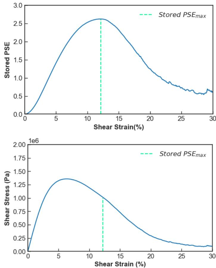
**Figure 24. Schematic for Peak Stored Pseudo-Strain Energy (PSE) and the Corresponding Shear Stress**
