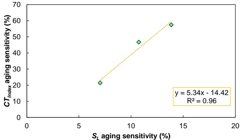
**Figure H16. Aging Sensitivity Across Binder and Mixture Scales for B1R1RA1, B1R1RA2, and B2R1RA5. B = virgin asphalt binder; R = reclaimed asphalt pavement (RAP) binder; RA = recycling agent.**
