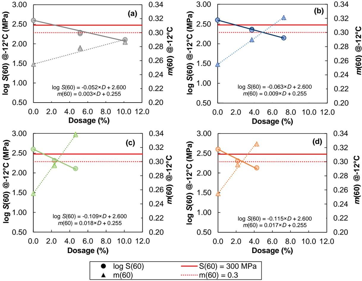
Figure 15. Relationship Between  $\log S(60)$  and  $m(6)$  With RA Dosage: (a) B1R2RA1; (b) B1R2RA2; (c) B1R2RA3; (d) B1R2RA4. B = virgin asphalt binder; R = reclaimed asphalt pavement (RAP) binder; RA = recycling agent.
