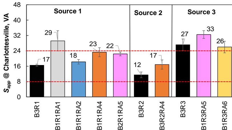
Figure 38. Cyclic Fatigue Test Data in Terms of  $S_{app}$  Values for Source 1, 2, and 3 Mixtures Determined Using Charlottesville Climatic Data.  $S_{app}$  = apparent damage capacity; B = virgin binder; R = reclaimed asphalt pavement (RAP); RA = recycling agent. Red dashed lines represent the corresponding range for standard traffic.
