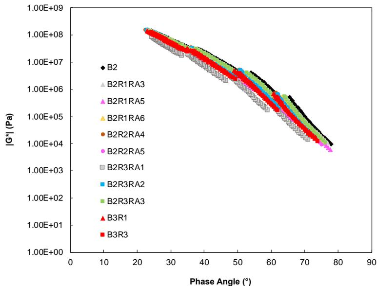
Figure 22. Black Space Graph for B2 Binder Blends and Reference Blends. B = virgin asphalt binder; R = reclaimed asphalt pavement (RAP); RA = recycling agent.
