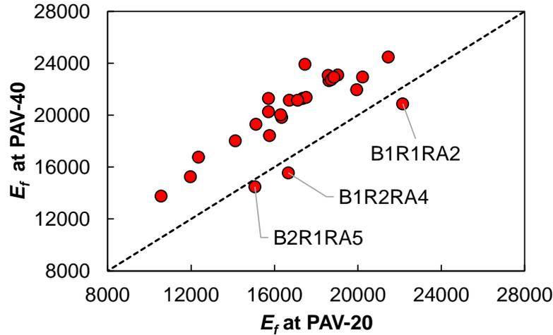
Figure H7. Strain Energy Tolerance for All Evaluated Binder Blends Under PAV-20 and PAV-40 Aging Conditions. PAV = pressure aging vessel; PAV-20 = PAV for a duration of 20 hours; PAV-40 = PAV for a duration of 40 hours; B = virgin asphalt binder; R = reclaimed asphalt pavement (RAP) binder; RA = recycling agent.
