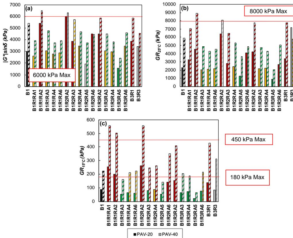
Figure G2. Intermediate-Temperature Point Parameters: (a)  $|G^*| \sin(\delta)$ ; (b)  $GR_{25^\circ C}$ ; (c)  $GR_{15^\circ C}$ . Colors convey Dunnett's test results: green, yellow, and red indicate better, equal, and worse results relative to B1, respectively. Gray indicates Dunnett's test could not be conducted due to unequal variance. B = virgin asphalt binder; R = reclaimed asphalt pavement (RAP); RA = recycling agent.
