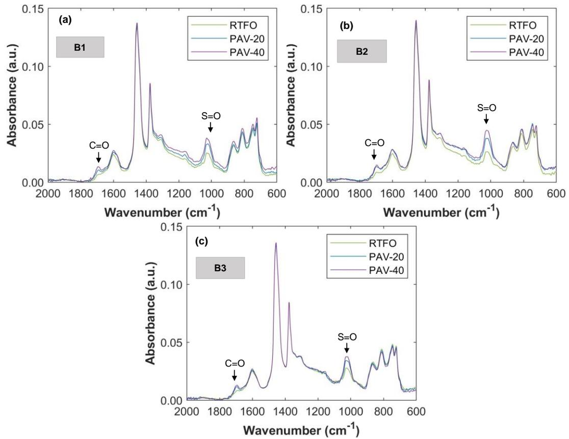
Figure II. FTIR Spectra for Virgin Binders: (a) B1; (b) B2; (c) B3. FTIR = Fourier transform infrared spectroscopy; B = virgin asphalt binder; RTFO = rolling thin film oven (short-term aging); PAV = pressure aging vessel; PAV-20 = aging in PAV for 20 hours; PAV-40 = aging in PAV for 40 hours.
