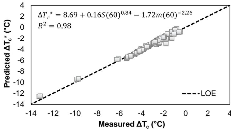
**Figure 17. Regression Model to Predict  $\Delta T_c$  Based on S and m-value at  $-12^\circ\text{C}$ . LOE = line of equality;  $S(60)$  = creep stiffness;  $m(60)$  = coefficient of relaxation;  $\Delta T_c$  = difference between the continuous grade based on  $S(60)$  and  $m(60)$  parameters.**
