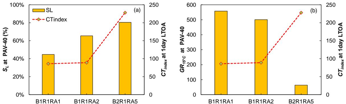
**Figure 49. Comparison of  $CT_{index}$  at 1-day LTOA of Selected Asphalt Mixtures With Parameters of Corresponding Binder Blends Under PAV-40 Aging Conditions: (a)  $S_L$ ; (b)  $GR_{15^\circ C}$ . B = virgin binder; R = reclaimed asphalt pavement (RAP); RA = recycling agent; PAV = pressure aging vessel; PAV-40 = PAV for a duration of 40 hours; CT = cracking tolerance, LTOA = long-term oven aging.**
