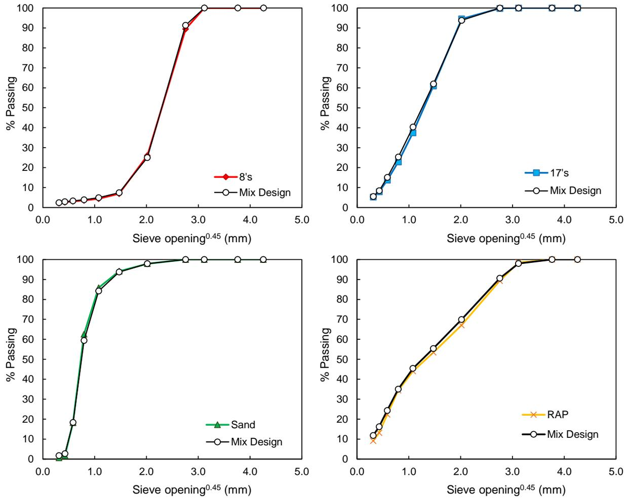
**Figure E3. Source 3 Aggregate and RAP Stockpile Gradations. RAP = reclaimed asphalt pavement.**
