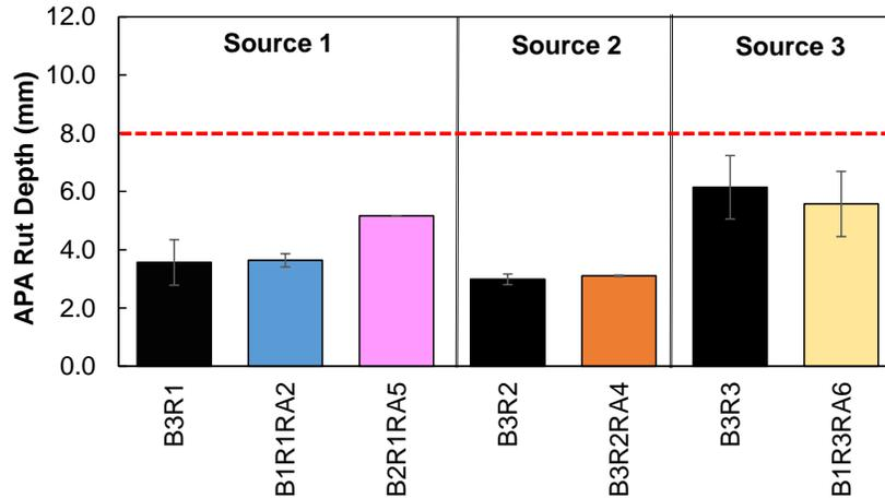
**Figure 39. Performance Test Data for APA Rut Depth of Source 1, 2, and 3 Mixtures. I-bars indicate rut depth variability  $\pm 1$  standard deviation. APA = Asphalt Pavement Analyzer; B = virgin binder; R = reclaimed asphalt pavement (RAP); RA = recycling agent. Red dashed line = balanced mix design special provision limit for surface asphalt mixtures with A and D designations.**
