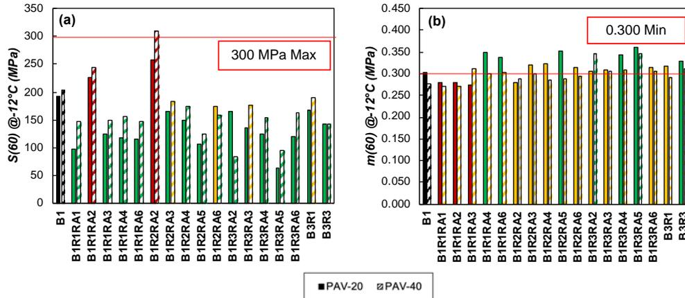
Figure G1. Low-Temperature Point Parameters: (a) stiffness  $S(60)$ ; (b) coefficient of relaxation  $m(60)$ . Colors convey Dunnett's test results: green, yellow, and red indicate better, equal, and worse results relative to B1, respectively. B = virgin asphalt binder; R = reclaimed asphalt pavement (RAP); RA = recycling agent.
