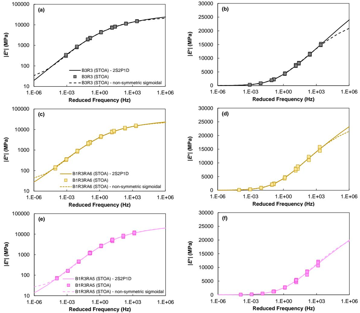
**Figure K1. Dynamic Modulus Master Curves Fitted Using 2S2P1D and Non-Symmetric Sigmoidal Model: (a) B3R3 in logarithmic space; (b) B3R3 in semi-logarithmic space; (c) B1R3RA6 in logarithmic space; (d) B1R3RA6 in semi-logarithmic space; (e) B1R3RA5 in logarithmic space; (f) B1R3RA5 in semi-logarithmic space.  $|E^*|$  = dynamic modulus; B = virgin binder; R = reclaimed asphalt pavement (RAP); RA = recycling agent; S = spring; P = parabola; D = dashpot; STOA = short-term oven aged.**
