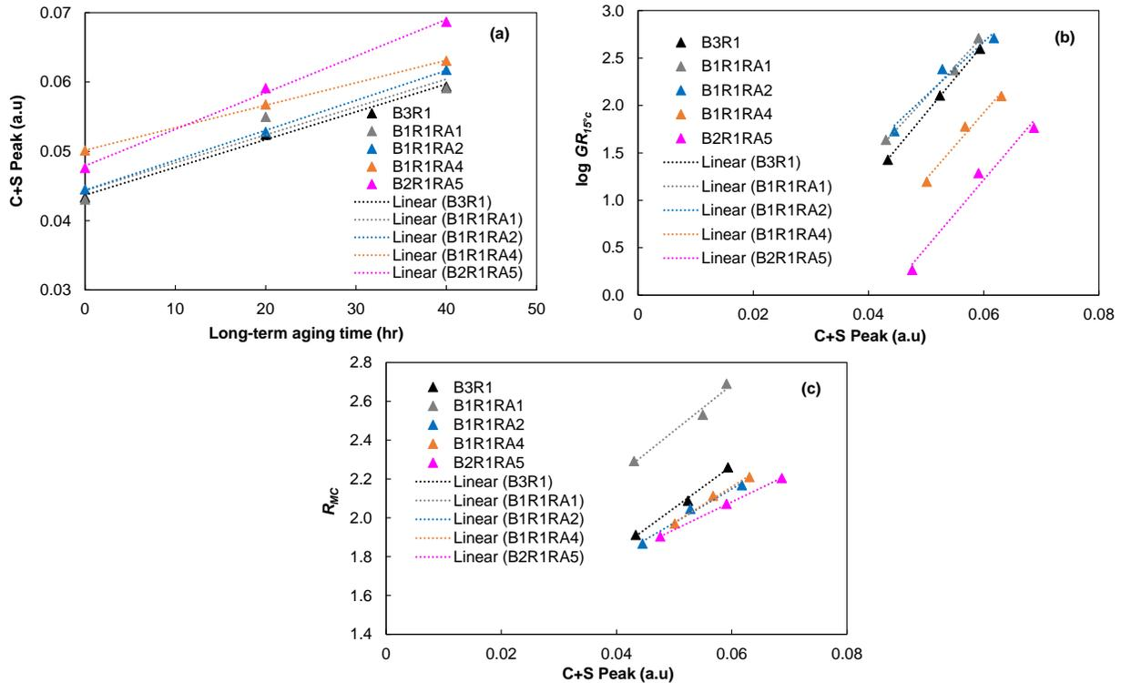
**Figure 29. FTIR for a Subset of Source 1 Blends: (a) changes of C+S with respect to aging time; (b) change of log GR<sub>25°C</sub> with respect to C+S; (c) change of R<sub>MC</sub> with respect to C+S. FTIR = Fourier transform infrared spectroscopy; C = carbonyl; S = sulfoxide; B = virgin asphalt binder; R = reclaimed asphalt pavement (RAP) binder; RA = recycling agent; GR = Glover-Rowe parameter; R = rheological index.**
