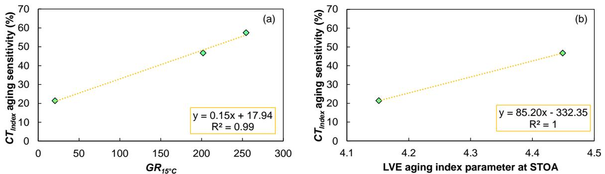
Figure 52. Cross-Scale Correlation Between 1-day  $CT_{index}$  Aging Sensitivity and (a) Binder Parameter  $GR_{15^\circ C}$  and (b) Mixture Parameter LVE.  $CT$  = cracking tolerance,  $GR$  = Glover-Rowe; LVE = linear viscoelastic.
