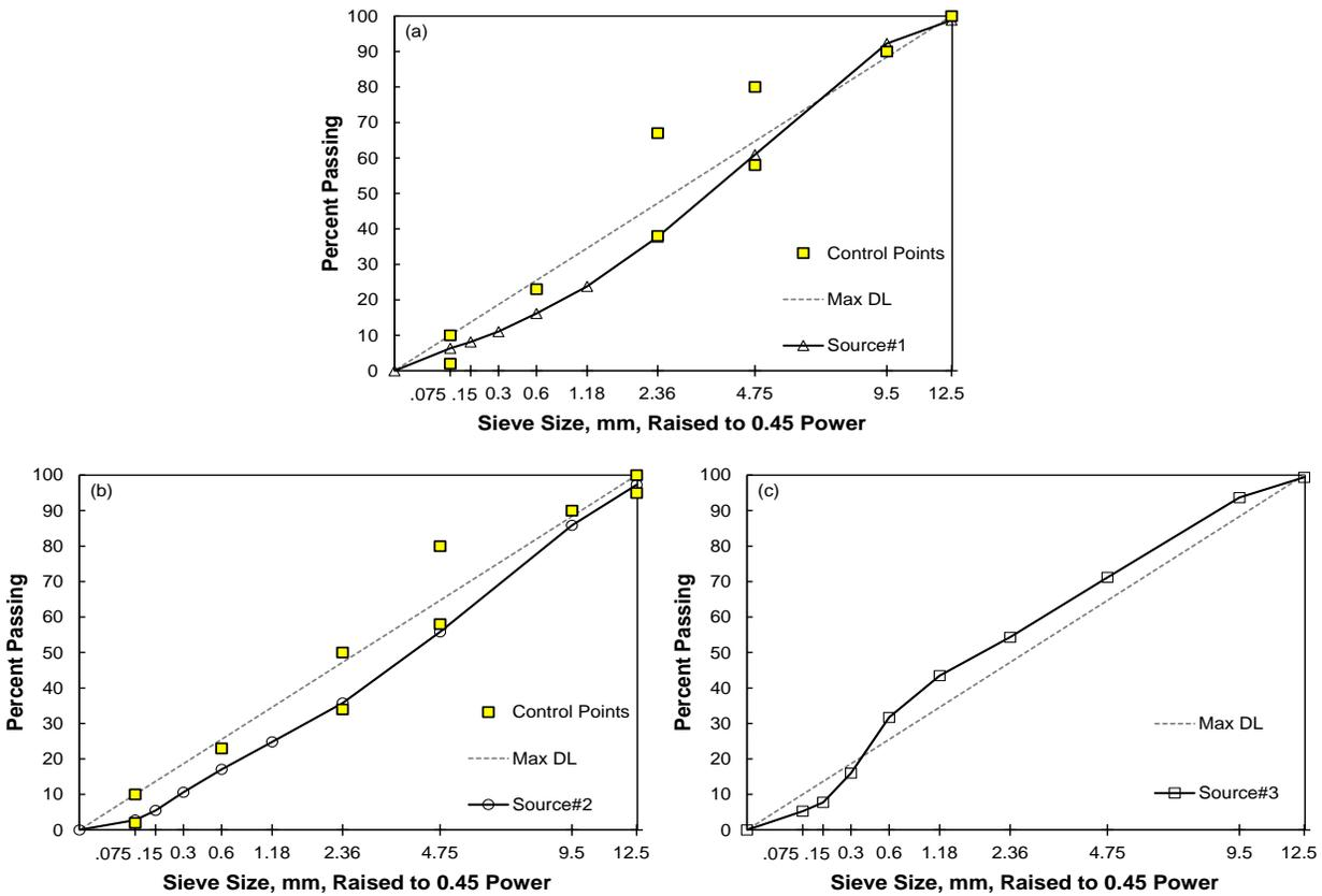
**Figure 30. Combined Gradations for All Three Sources: (a) Source 1 from Salem; (b) Source 2 from Burkeville; (c) Source 3 from Chesapeake. DL = density line.**
