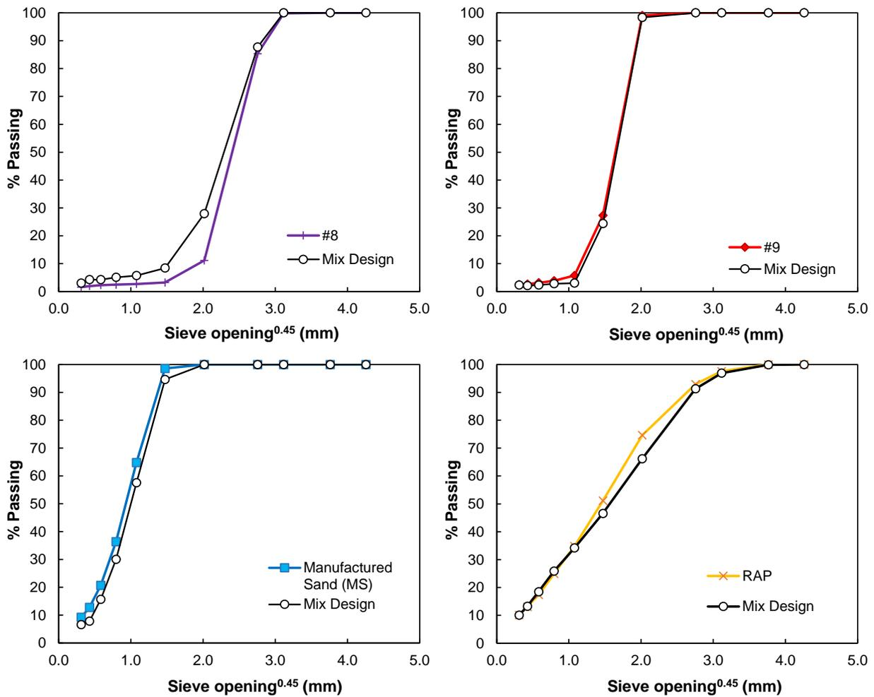
**Figure E1. Source 1 Aggregate and RAP Stockpile Gradations. RAP = reclaimed asphalt pavement.**
