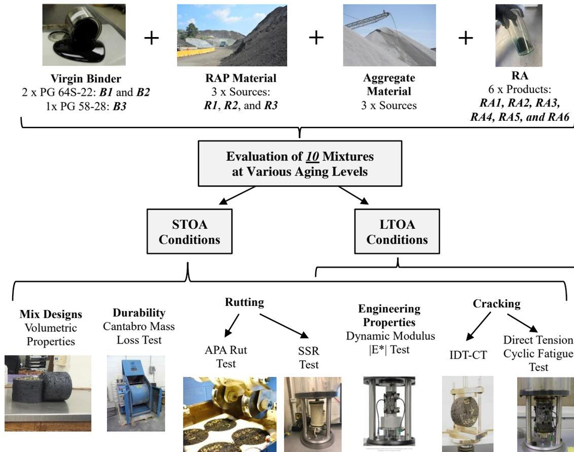
Figure 2. Flowchart of the Laboratory Experimental Program for Phase II of the Study. PG = performance grade; S = standard traffic; B = virgin asphalt binder; RAP = reclaimed asphalt pavement; R = RAP source; RA = recycling agent; STOA = short-term oven aged; LTOA = long-term oven aged; APA = Asphalt Pavement Analyzer; SSR = stress sweep rutting; IDT-CT = indirect tensile cracking test.
