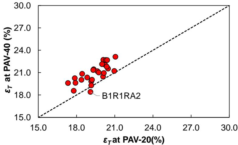
**Figure H6. Strain Tolerance Up to Failure (Post Peak) for All Evaluated Binder Blends Under PAV-20 and PAV-40 Aging Conditions.** PAV = pressure aging vessel; PAV-20 = PAV for a duration of 20 hours; PAV-40 = PAV for a duration of 40 hours; B = virgin asphalt binder; R = reclaimed asphalt pavement (RAP) binder; RA = recycling agent.
