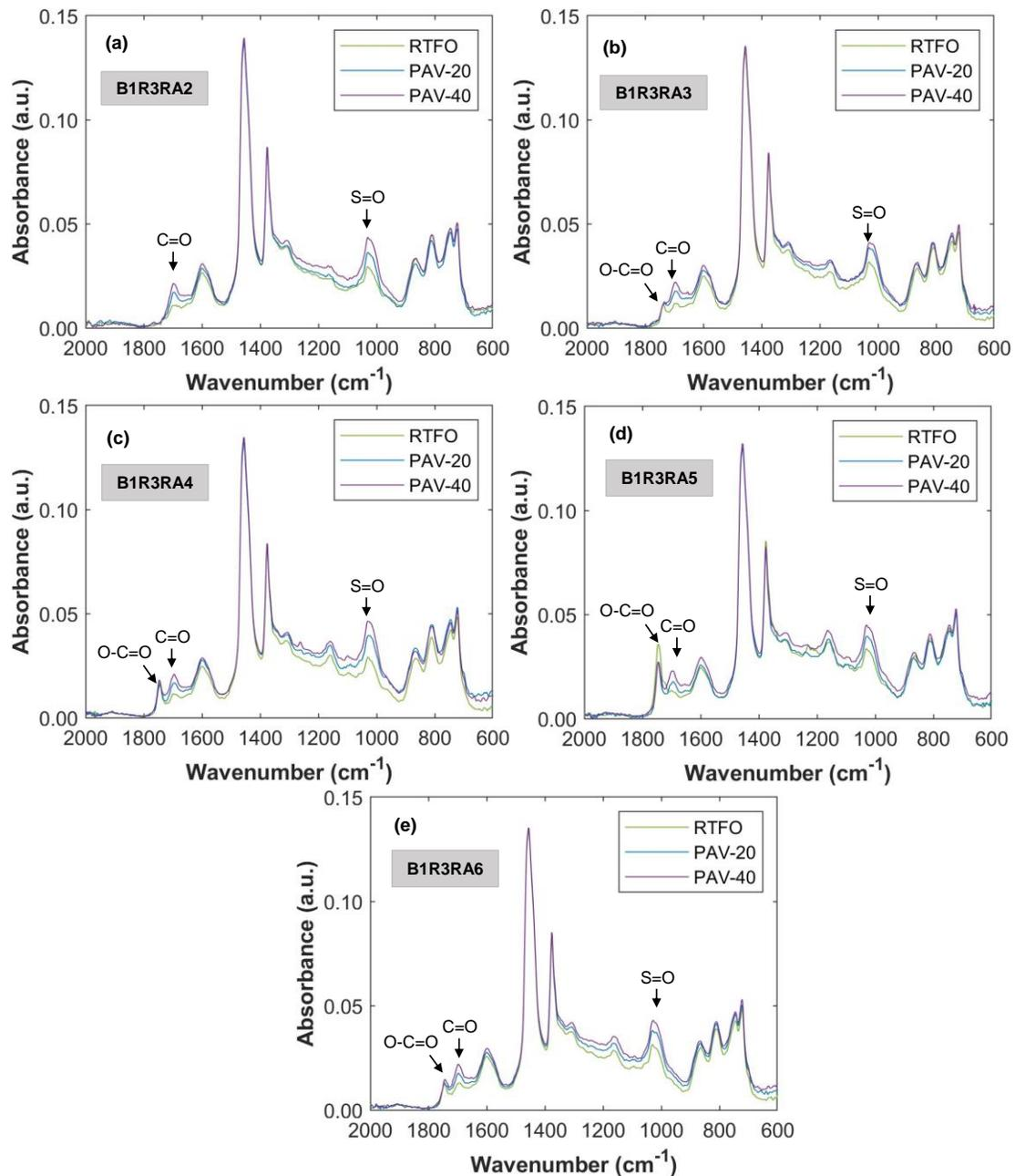
Figure I4. FTIR Spectra for B1R3 Blends: (a) B1R3RA2; (b) B1R3RA3; (c) B1R3RA4; (d) B1R3RA5; (e) B1R3RA6. FTIR = Fourier transform infrared spectroscopy; B = virgin asphalt binder; R = reclaimed asphalt pavement (RAP) binder; RA = recycling agent; RTFO = rolling thin film oven (short-term aging); PAV = pressure aging vessel; PAV-20 = aging in PAV for 20 hours; PAV-40 = aging in PAV for 40 hours.
