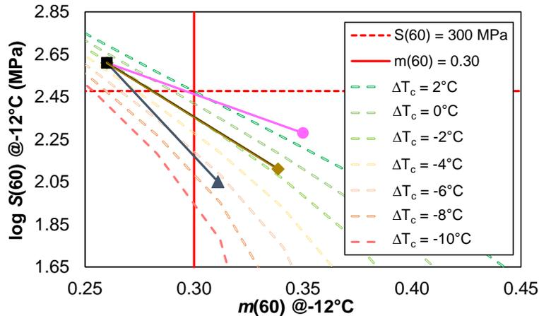
**Figure 18. Black Space Diagram Considering  $\Delta T_c$  Prediction Curves. Filled squares indicate possible rejuvenation paths.  $S(60)$  = creep stiffness;  $m(60)$  = coefficient of relaxation;  $\Delta T_c$  = difference between the continuous grade based on  $S(60)$  and  $m(60)$  parameters.**
