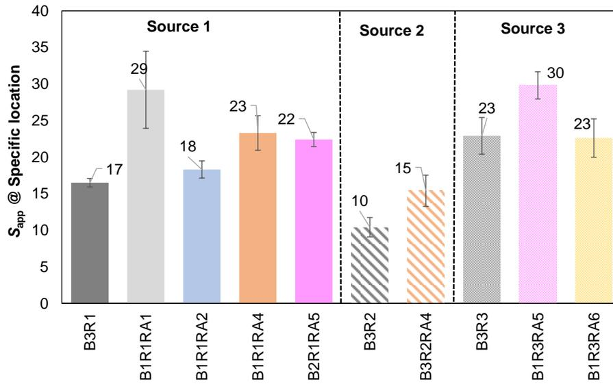
**Figure J1. Cyclic Fatigue Performance Test Data in Terms of  $S_{app}$  Values for Source 1, 2, and 3 Mixtures Determined Using Local Specific Climatic Data: Blacksburg, Virginia, for Source 1 mixtures (15°C); Mecklenburg, Virginia, for Source 2 mixtures (18°C); and Chesapeake, Virginia, for Source 3 mixtures (21°C).  $S_{app}$  = apparent damage capacity. B = virgin binder; R = reclaimed asphalt pavement (RAP); RA = recycling agent.**
