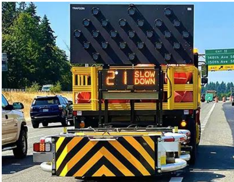
Figure 12. Dynamic message sign activated by operator or approaching vehicle
