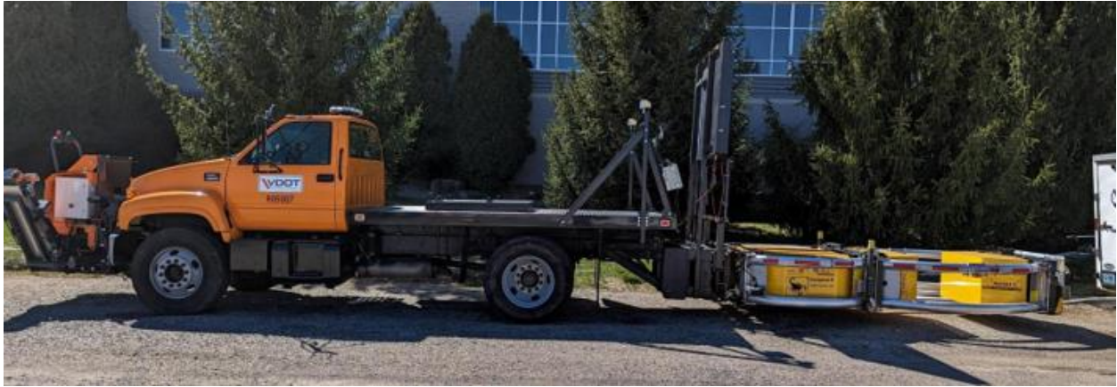
Figure 4. TMA truck with Scorpion attenuator and custom-mounted panels
