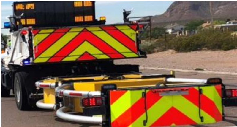
Figure 13. Extra markings placed above the cushion and below the arrow board
