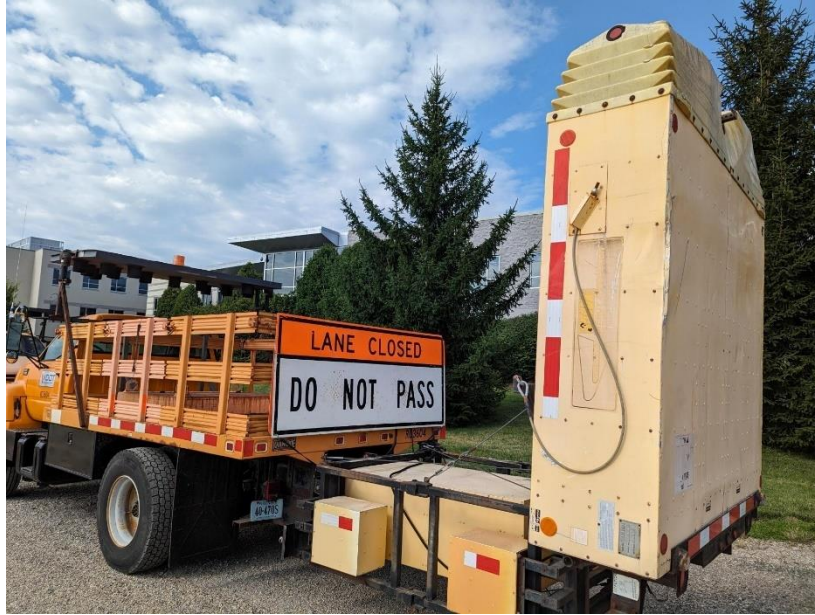
Figure 11. A TMA truck with a static sign
