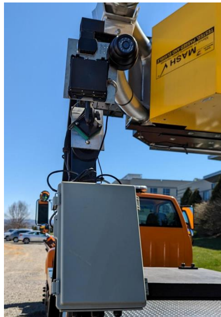
Figure 5. Move-Over Law data collection unit mounted on Stinger support beam
