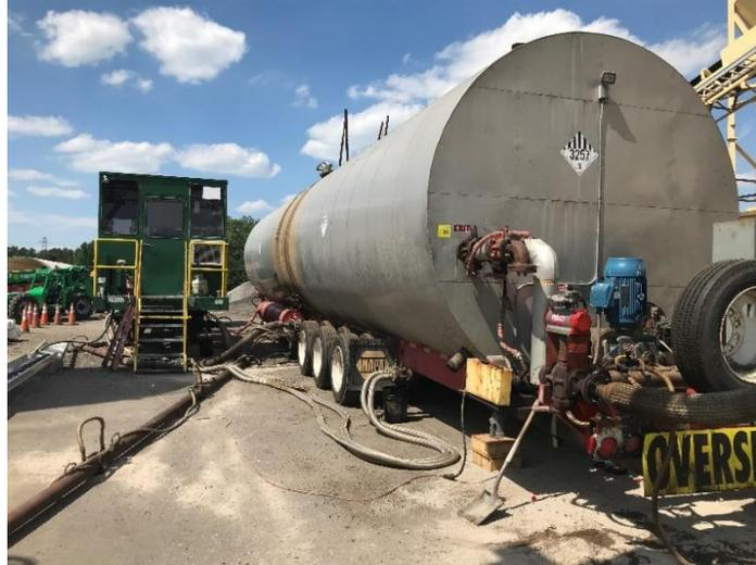
**Figure 7. Asphalt Rubber Binder Holding Tank**
