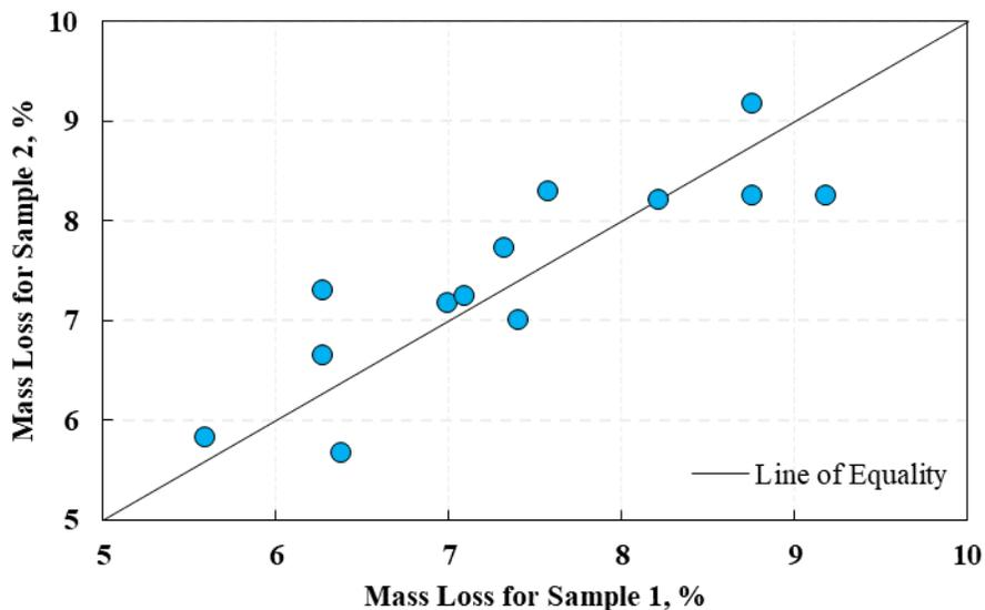
Figure 9. Within-Lot Sample-to-Sample Comparison for Cantabro Test
