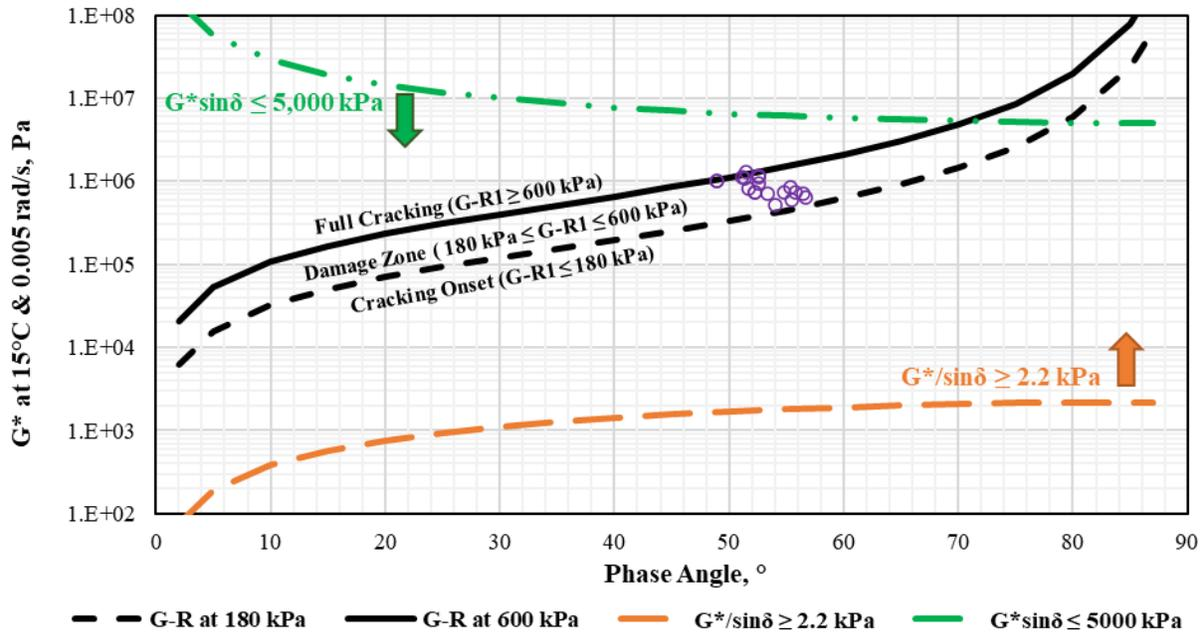
**Figure 14. Black Space Diagram in Terms of Glover-Rowe (G-R1) Values at  $15^\circ\text{C}$  and  $0.005\text{ rad/s}$  for 2021 Binders at 20-Hour PAV Aging Conditions.** PAV = pressure aging vessel;  $G^*$  = complex shear modulus;  $\delta$  = phase angle.
