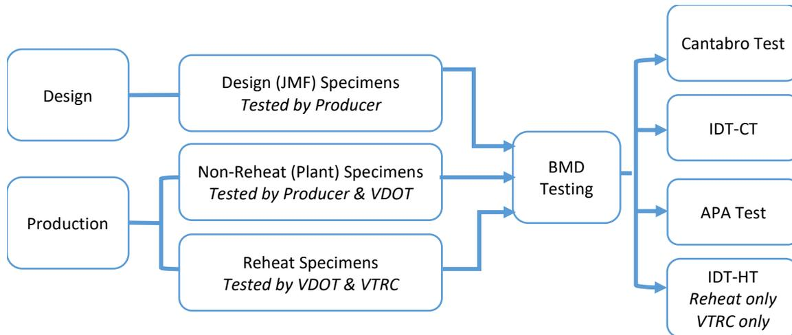
**Figure 1. Testing Performed on Laboratory- and Plant-Produced Mixtures.** JMF = job-mix formula; VDOT = Virginia Department of Transportation; BMD = balanced mix design; IDT-CT = indirect tensile cracking test; APA = Asphalt Pavement Analyzer; IDT-HT = indirect tensile test at high temperature; VTRC = Virginia Transportation Research Council.
