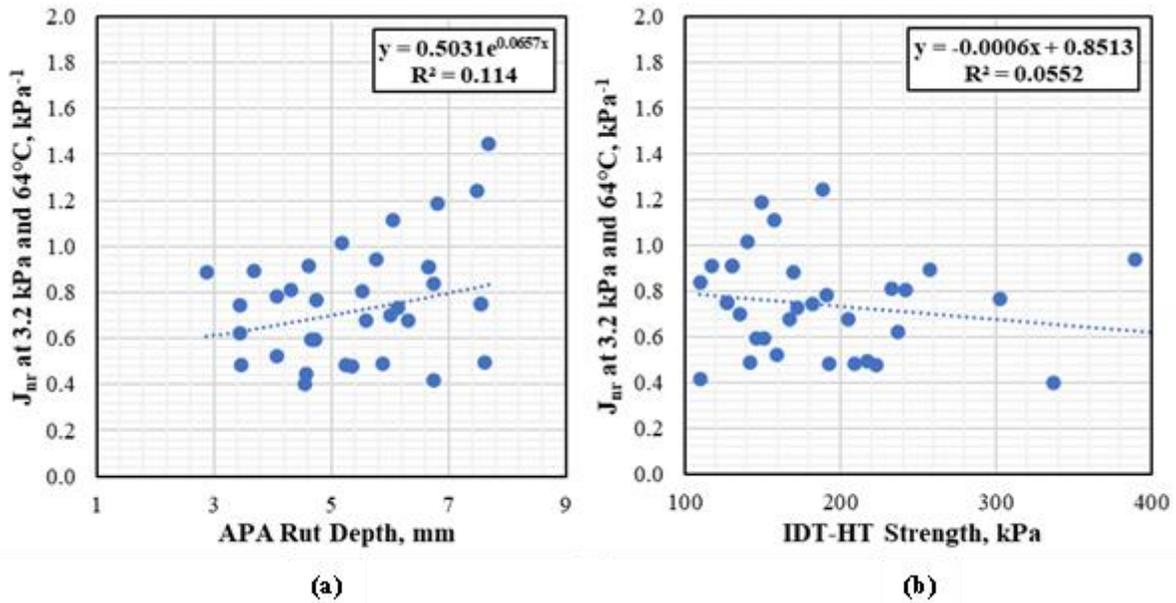
**Figure 19. Correlation Between  $J_{nr, 3.2 \text{ kPa}}$  and (a) APA Rut Depth and (b) IDT-HT Strength.  $J_{nr, 3.2 \text{ kPa}}$  = non-recoverable creep compliance at 3.2 kPa; APA = asphalt pavement analyzer; IDT-HT = indirect tensile test at high temperature.**
