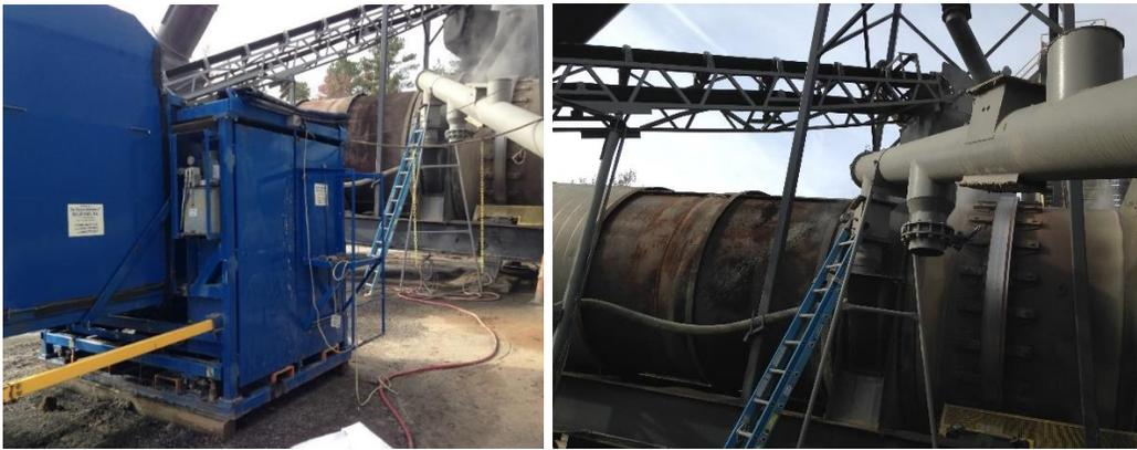
**Figure 4. Adding GTR in the Asphalt Plant (Dry Process): left, GTR feeding machine; right, GTR added through the RAP collar. GTR = ground tire rubber; RAP = reclaimed asphalt pavement.**
