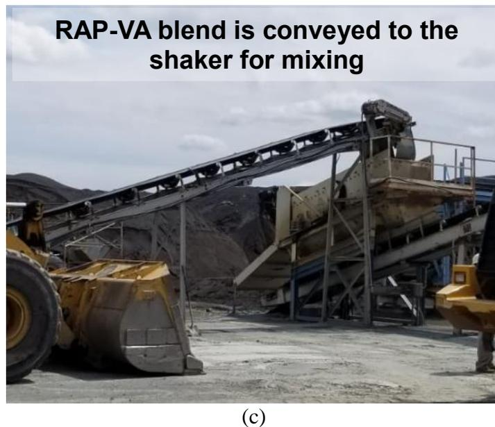
Figure A2: Blending RAP and VA at an asphalt plant
