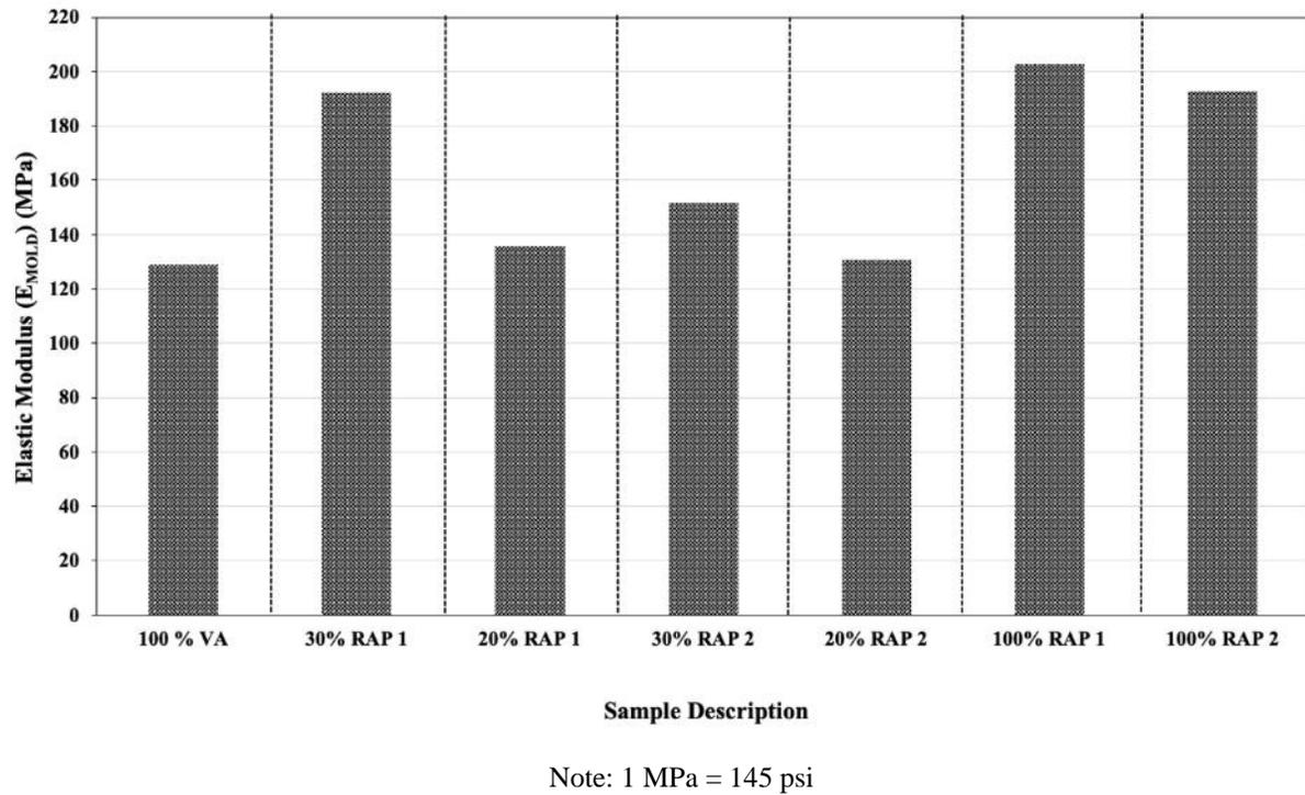
Figure 24: Light Weight Deflectometer (LWD) Test Results Performed on Compaction Mold
