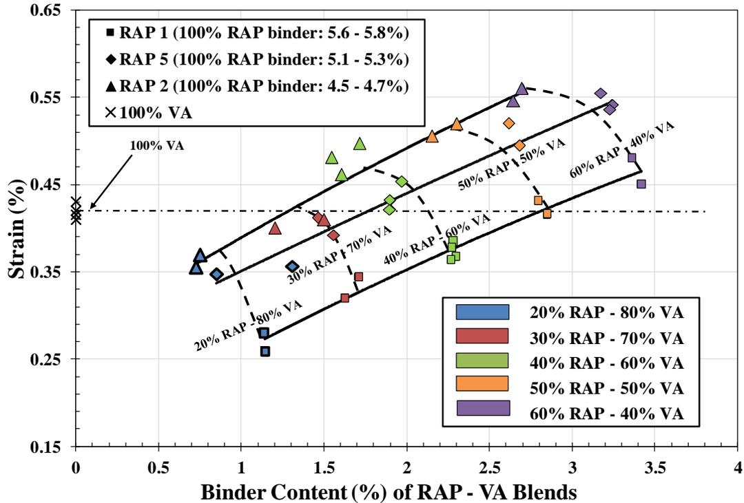
Note: The dashed lines shown as are drawn to indicate theoretical boundaries between the RAP-VA blends that resulted in the presented data.
