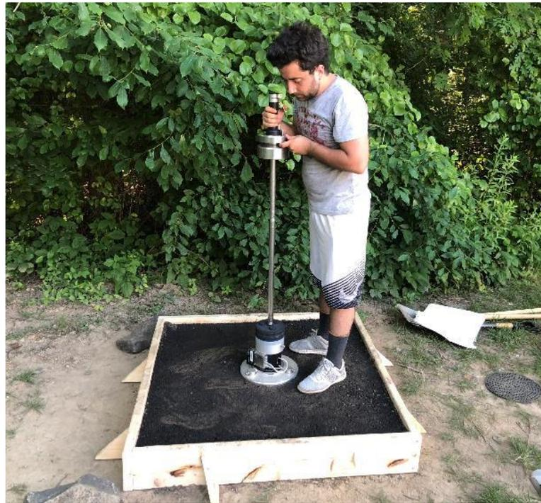
**Figure 4: Field Scale Model Evaluation (FSME) Testing System**
