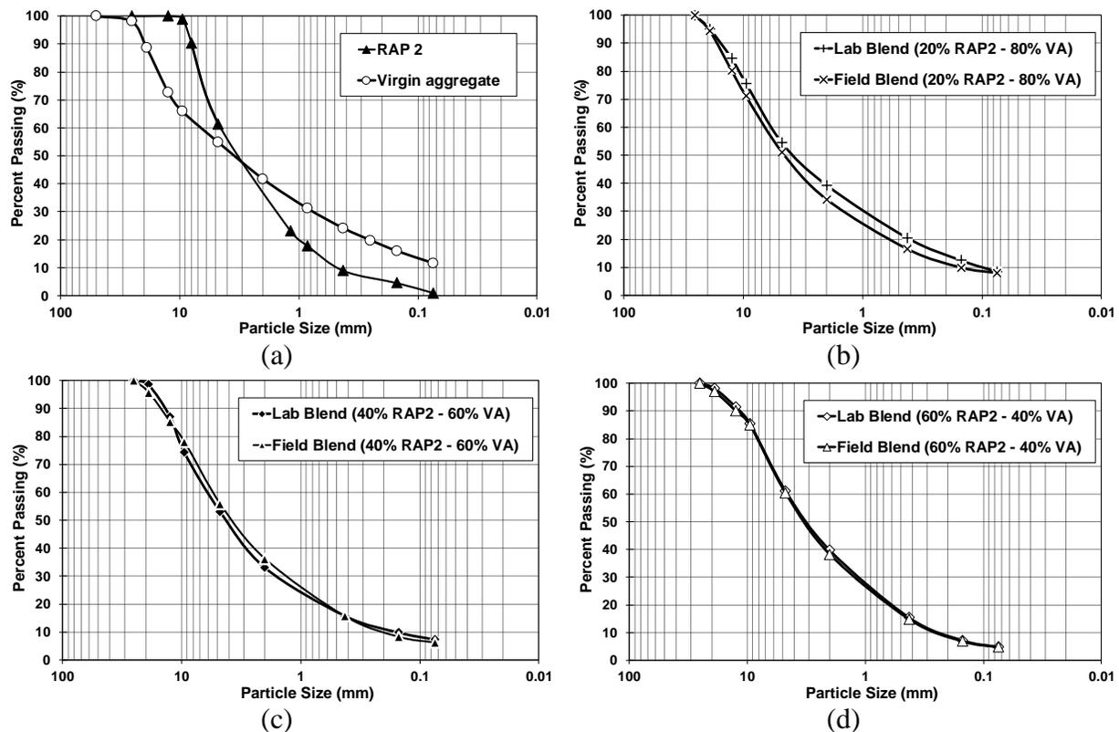
Figure A3: GSD test results for samples prepared after bucket and pugmill mixing in the field.
