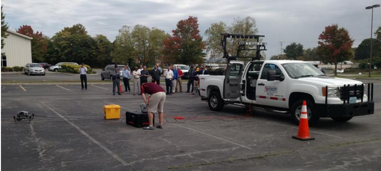
**Figure 3. View of the Safety Services Patrol Truck and Paired, Tethered UAV Prior to Take-off**
