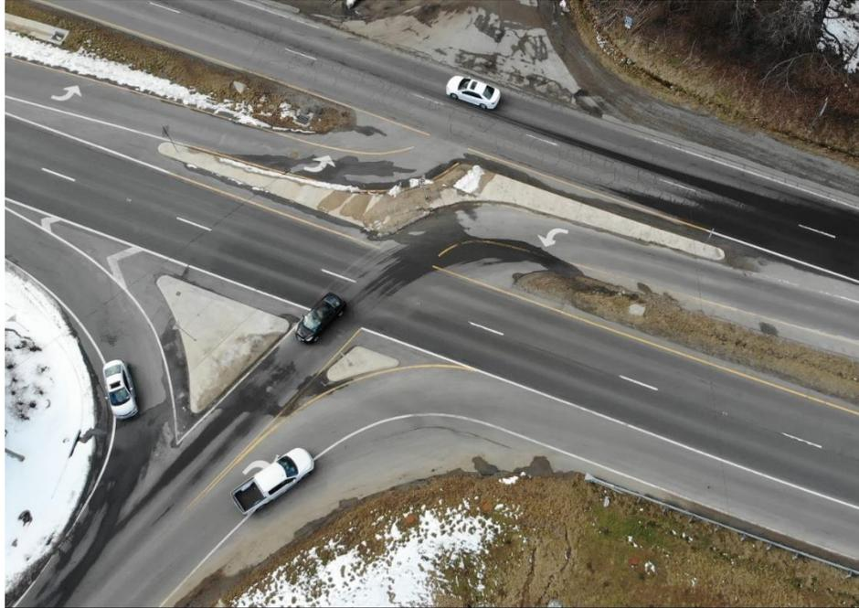
**Figure 7. Travel, Crossing, and Merge Lanes at a Restricted Crossing U-Turn Intersection**
