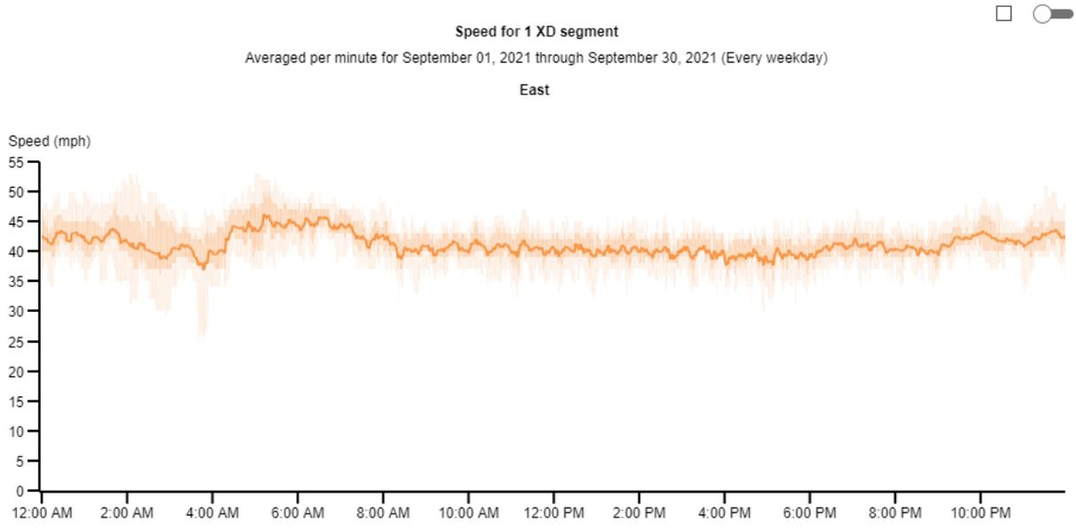
**Figure A5. Speed profile for XD3 segment shown in Figure A2**
