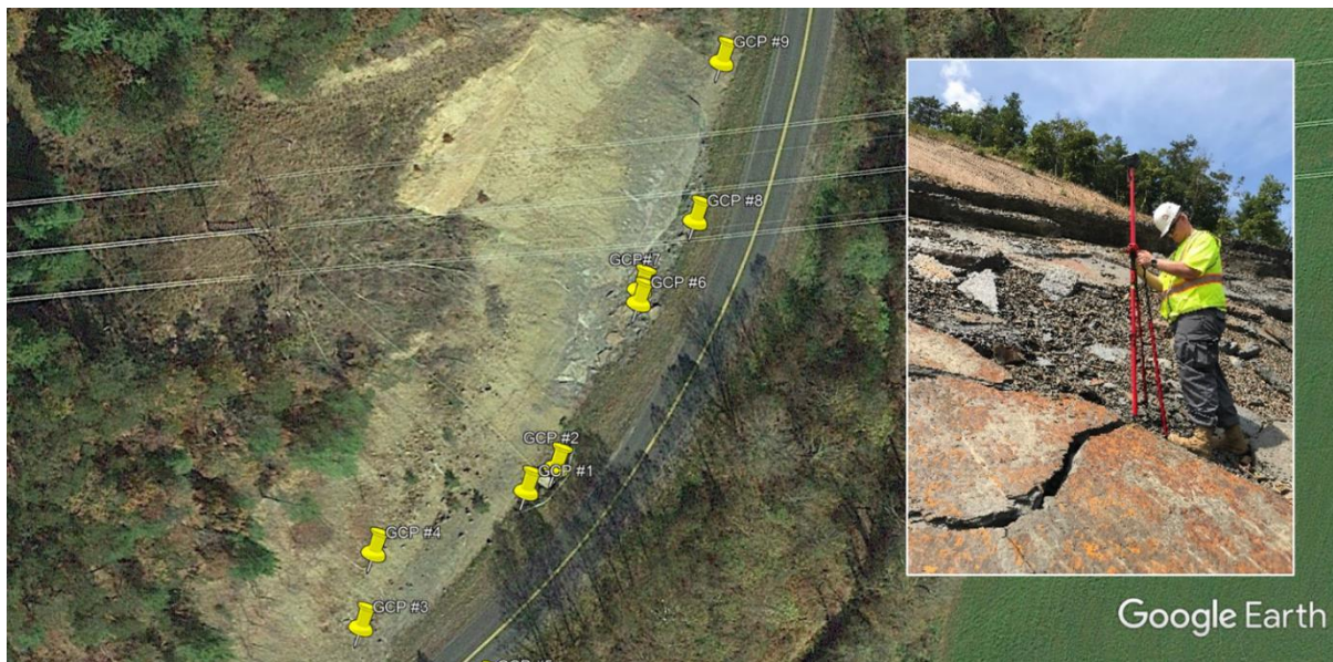
Figure 9. Satellite image of surveyed ground control points (GCPs) at Site #2 Deerfield. The inset shows graduate student James Young obtaining coordinates for GCP #7 using a roving, Emlid RTK GPS receiver, synchronized to a nearby base station in 2019. Base map from Google Earth.
