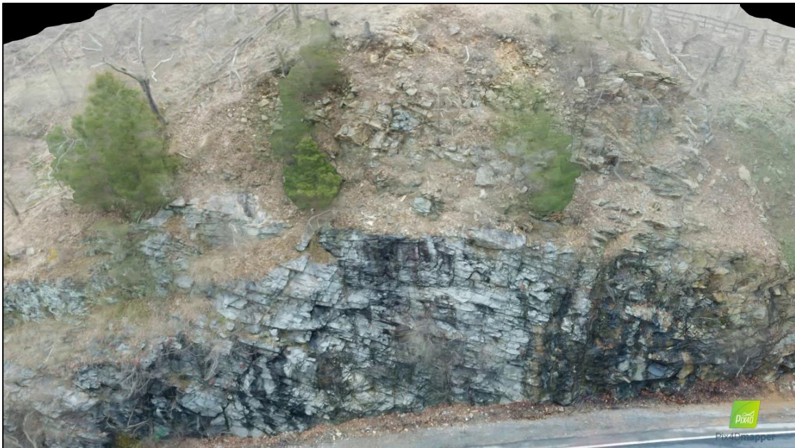
Figure 28. Site #4, Route 340, Harpers Ferry, Virginia. This is not a photograph, rather a portion of the georeferenced densified point cloud from which topographic maps and sections (below) were generated by Pix4D Mapper . Results were then transferred to ArcMap for distribution to HDR for constructability review purposes. This image is a screen capture from a video animation of the dense point cloud.
