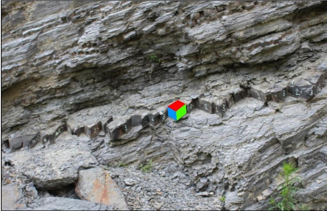
Figure 25. Site #2, Deerfield. Example of extraction of structure data from UAS-based point cloud for plotting on stereonets (Delaney, et al., 2020).
