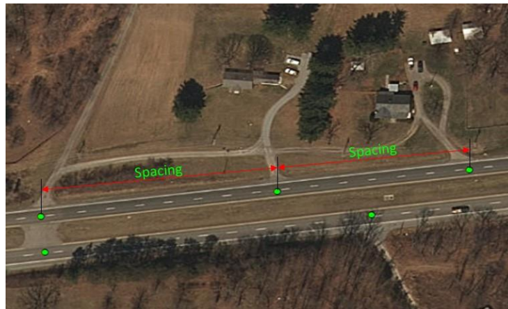
Figure 4. Spacing Calculation Based on ArcMap. Map Data. Sources: ESRI, VITA, West Virginia GIS, Esri, HERE, Garmin, INCREMENT P, Intermap, USGS, METI/NASA, EPA, USDA. (The aforementioned sources are listed in the original basemap created when using ESRI ArcGIS® software in 2019, and as they are not visible in Figure 4 those sources are listed here.)
