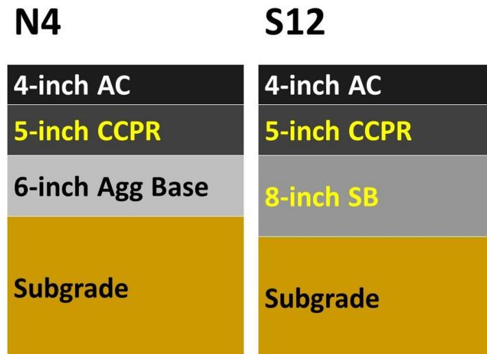
Figure 4. Schematic of NCAT Test Track Sections Including CCPR. NCAT = National Center for Asphalt Technology; CCPR = cold central plant recycling; AC = asphalt concrete; Agg = aggregate; SB = stabilized base.
