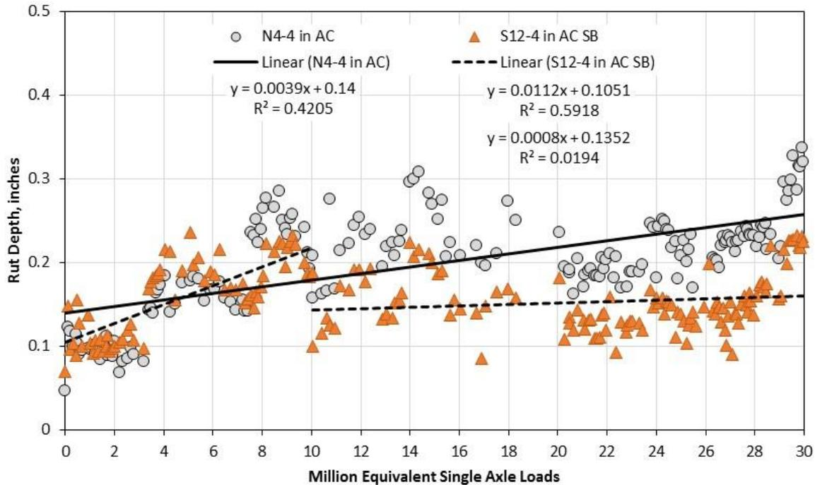
Figure 7. Rut Depth Results. AC = asphalt concrete; SB = stabilized base.
