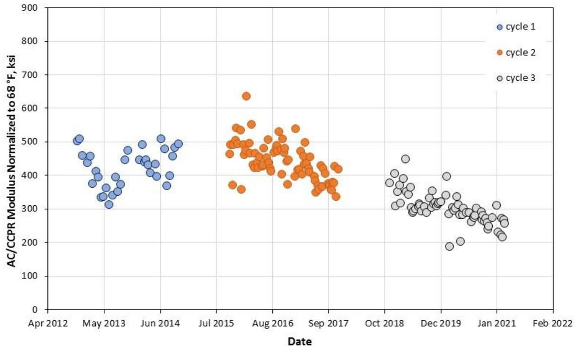
**Figure 9. Section N4 Temperature-Normalized AC/CCPR Modulus. AC = asphalt concrete; CCPR = cold central plant recycling.**
