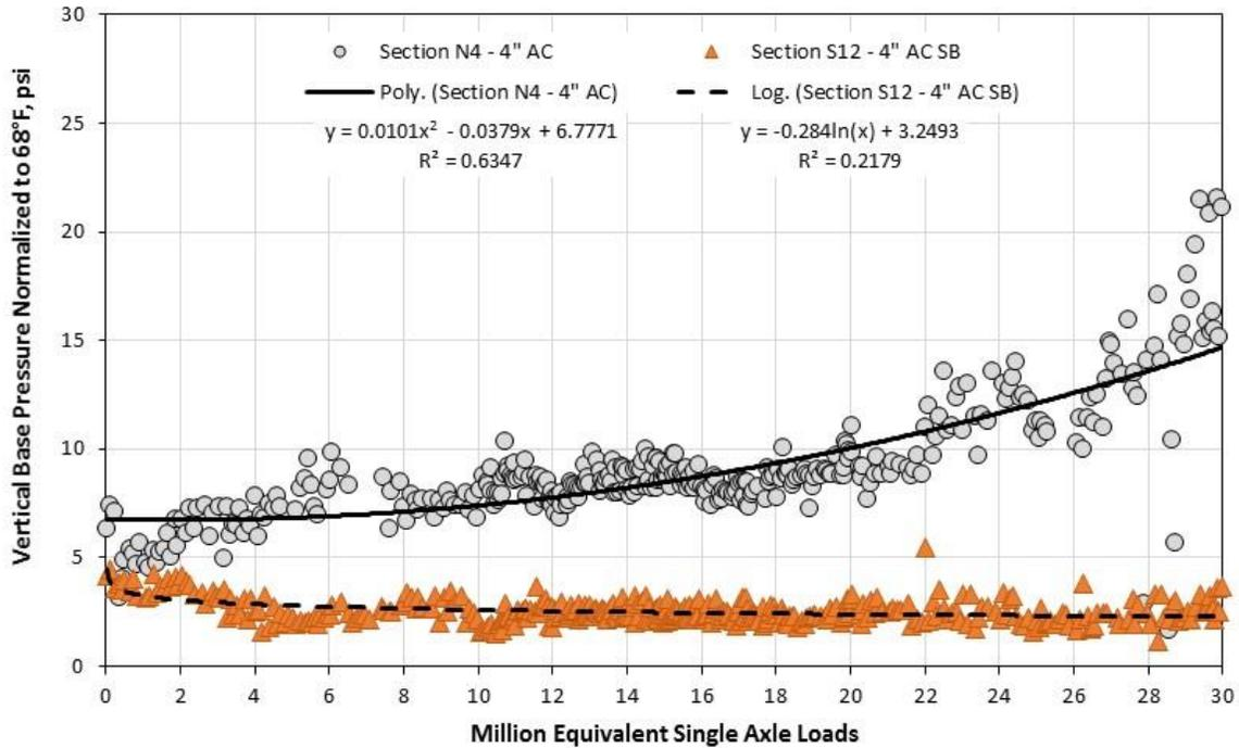
Figure 12. Vertical Base Pressure vs. Million Equivalent Single Axle Loads. AC = asphalt concrete; Poly. = polynomial trendline; SB = stabilized base; Log. = logarithmic trendline.
