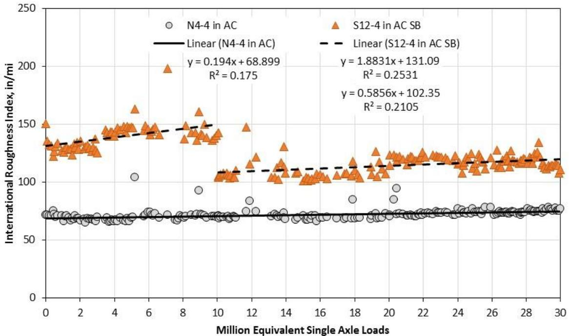
Figure 6. Ride Quality Results. AC = asphalt concrete; SB = stabilized base.
