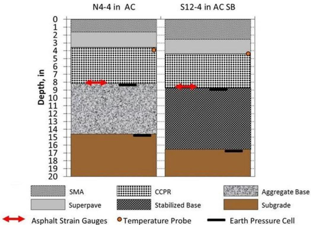
Figure 5. VDOT Sections at NCAT Test Track Showing Average As-Built Thicknesses and Depth of Instrumentation. VDOT = Virginia Department of Transportation; NCAT = National Center for Asphalt Technology; AC = asphalt concrete; SB = stabilized base; SMA = stone matrix asphalt; CCPR = cold central plant recycling.
