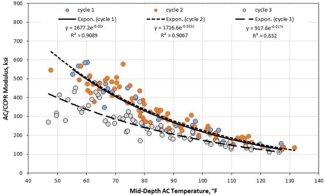
**Figure 8. Section N4 AC/CCPR Modulus. AC = asphalt concrete; CCPR = cold central plant recycling; Expon. = exponential trendline.**
