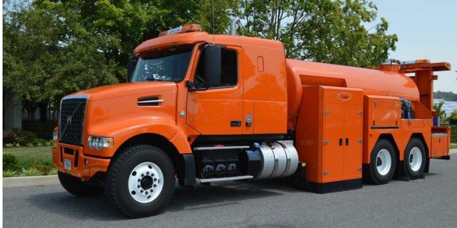
**Figure 2. SCRIM. Instrumentation is housed in the truck.**
