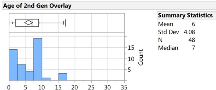
Figure 30. Histogram of Age of Second-Generation Overlays
