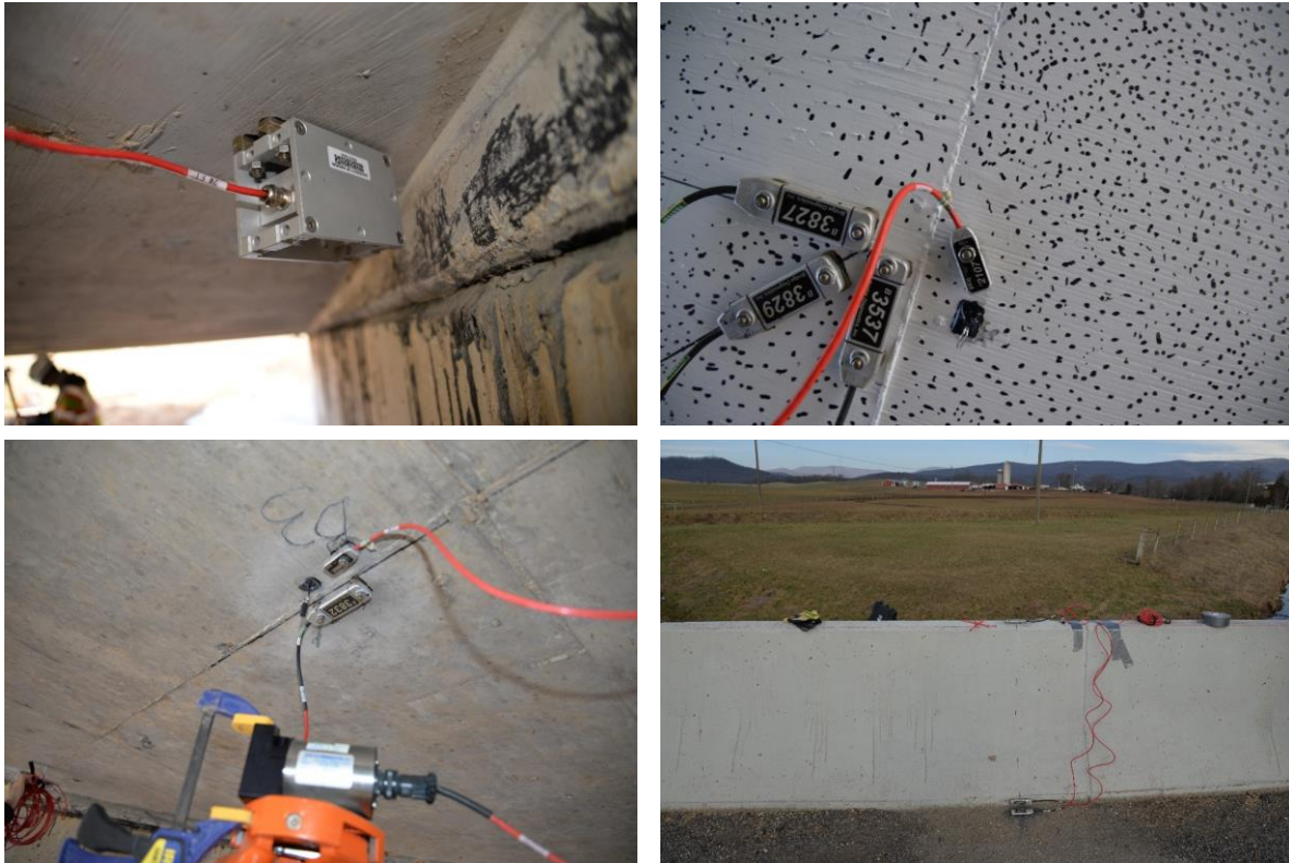
Figure 4 - Representative Images of BDI Instrumentation. Clockwise from top left: tiltmeter, strain gauge rosette and accelerometer, strain gauge and accelerometer, strain gauges)
