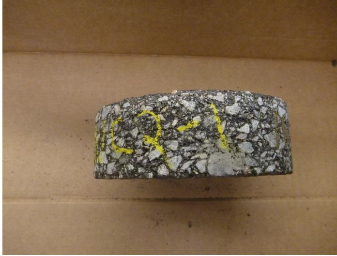
Figure 17. Core Showing Microsurfacing Above Existing Asphalt Top Surface
