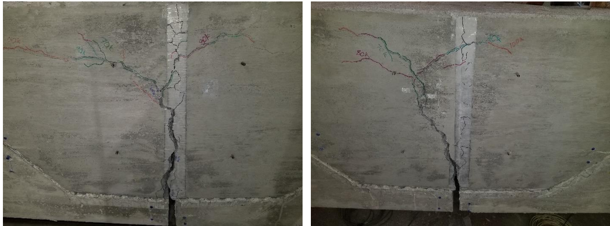
Figure 52. No Connection Specimen with Good Surface Roughening at Failure Load of 130 kips (East Side Left and West Side Right)
