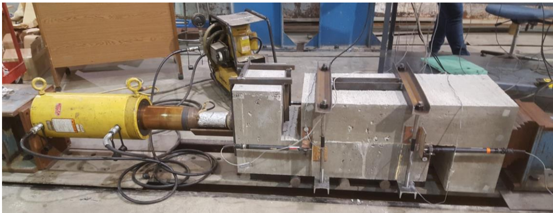
Figure 12. Horizontal Shear Push-off Specimen Testing Apparatus
