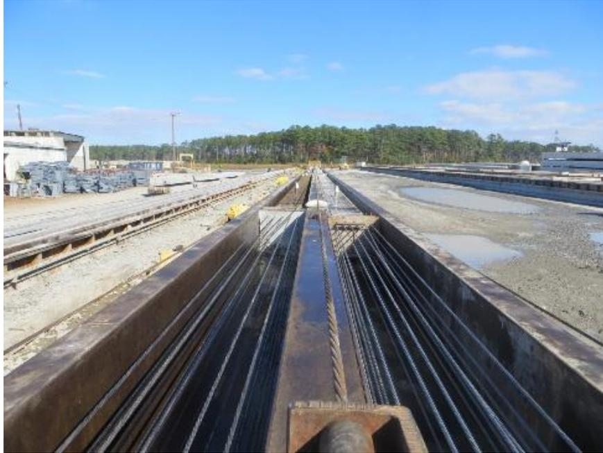
**Figure 19. Preparing to Make 24-in-Square Prestressed Concrete Piles. Conventional steel strand shown on the left and 2205 stainless strand shown on the right in a 400-ft-long bed. Not shown are the steam curing pipes that lay adjacent to the bed near the ground.**
