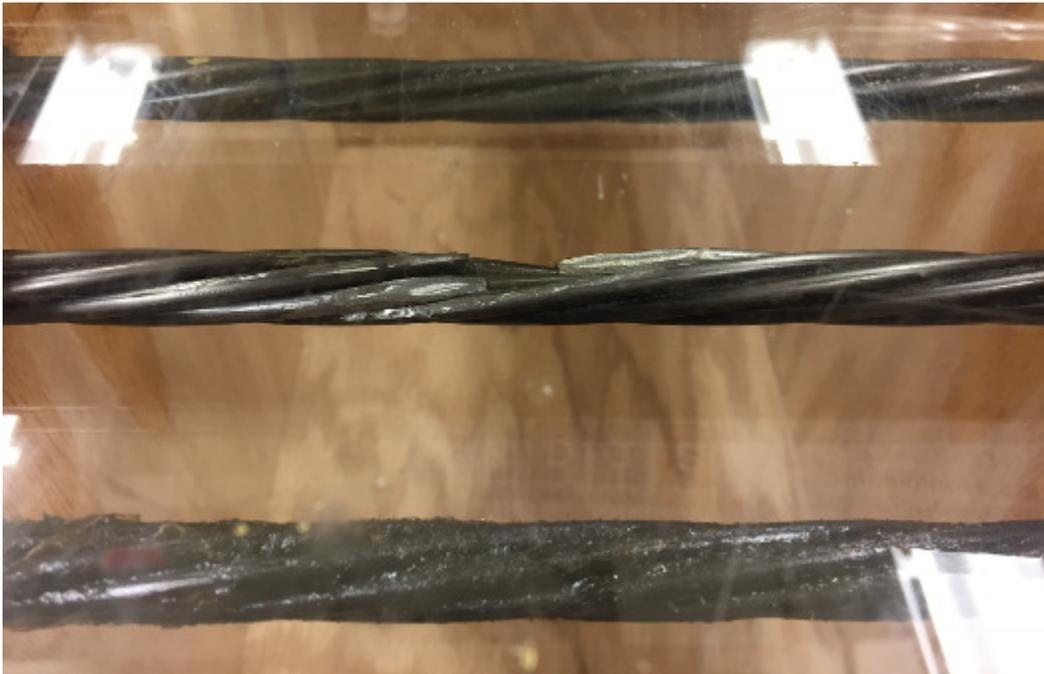
**Figure 11. Strand With Gradual Section Loss**
