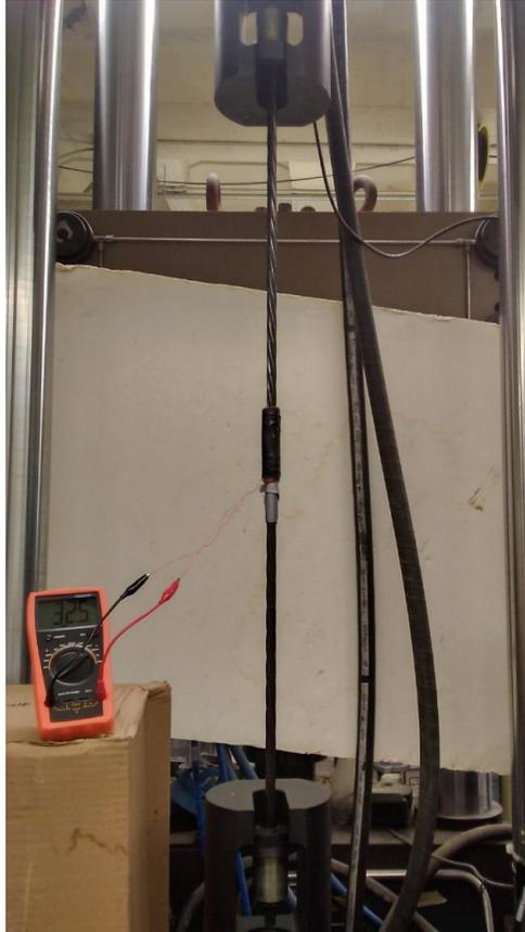
**Figure 22. Tensile Loading and Magnetic Permeability Measurement**
