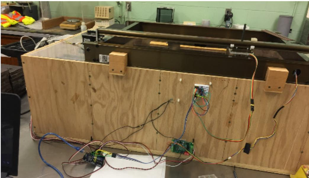
Figure 9. Magnetic Flux Leakage Inspection System Test Fixture
