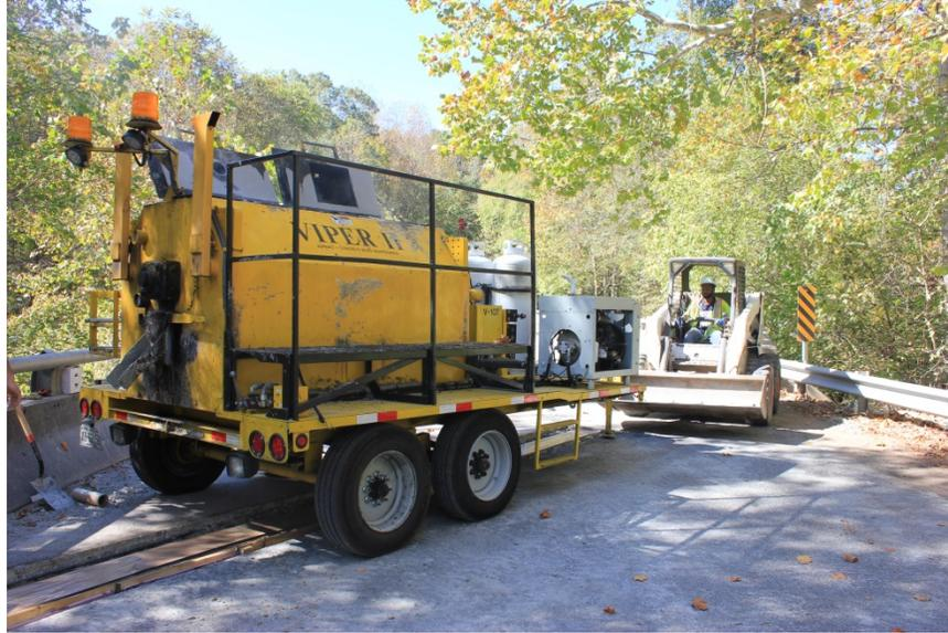
**Figure 22. Equipment for Hot Pours**
