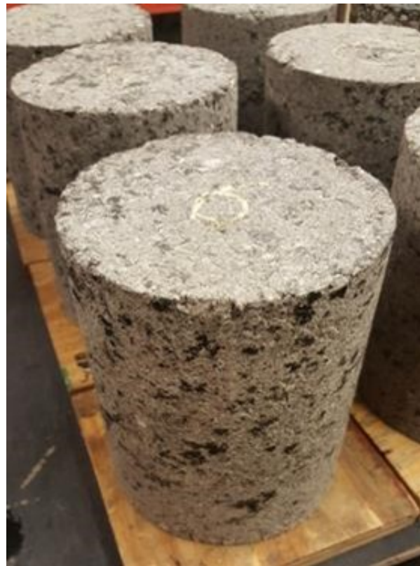
Figure 7. Cured CCPR Specimen for Dynamic Modulus Testing. CCPR = cold central plant recycling.
