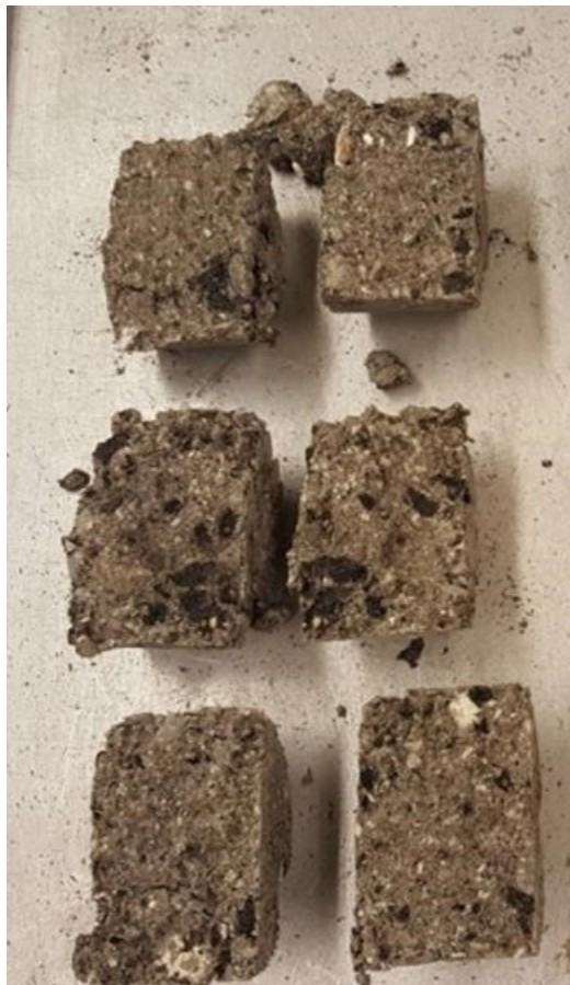
Figure 10. ITS Specimens After Breaking. ITS = indirect tensile strength.
