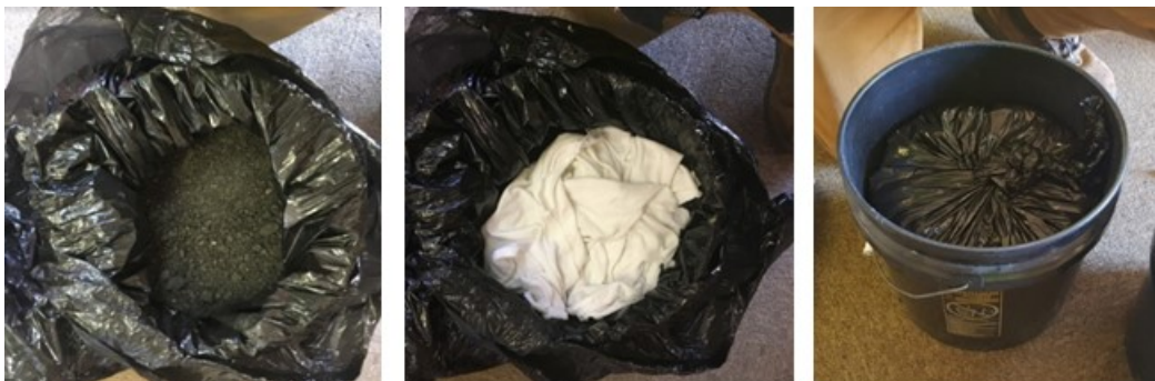
Figure 2. Sampled CCPR Mixture: (Left) mixture placed into plastic bag lining the bucket; (Middle) damp rags placed on top of mixture; (Right) plastic bag tied around mixture. CCPR = cold central plant recycling.
