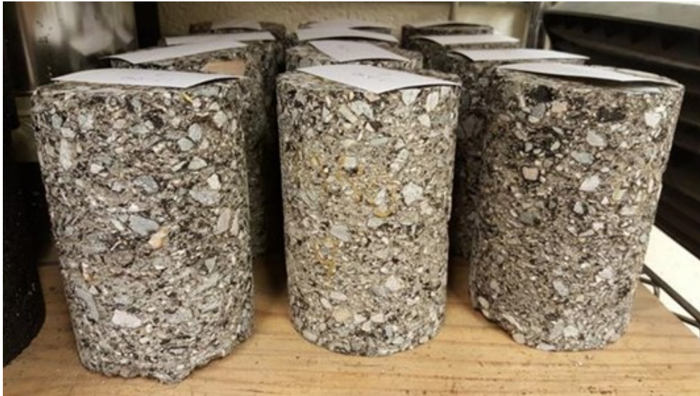
Figure 8. 150-mm Specimen for Dynamic Modulus Test
