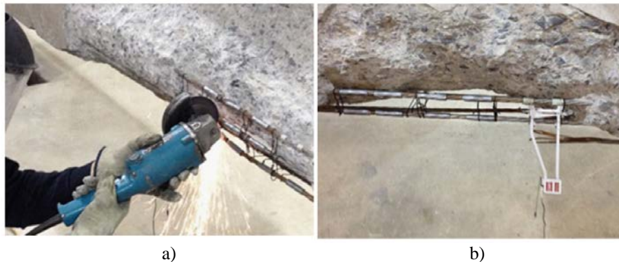
Figure 11. a) Electric Grinder Cutting a Strand and b) Extensometer to Measure Length Change
