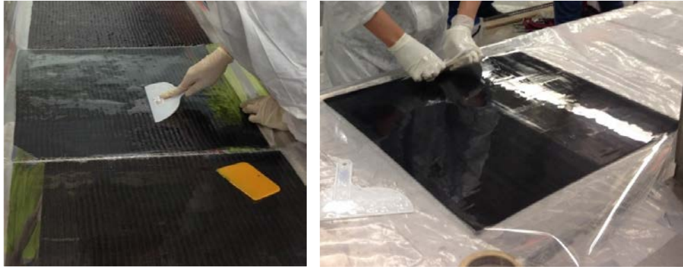
Figure 7. FRP Panel Fabrication
