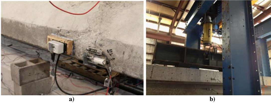
Figure 30. a) MLVDT, Strain Transducer, and Potentiometer, b) Load Cell, Actuator, Spreader Beam, and Rubber Bearing Pads
