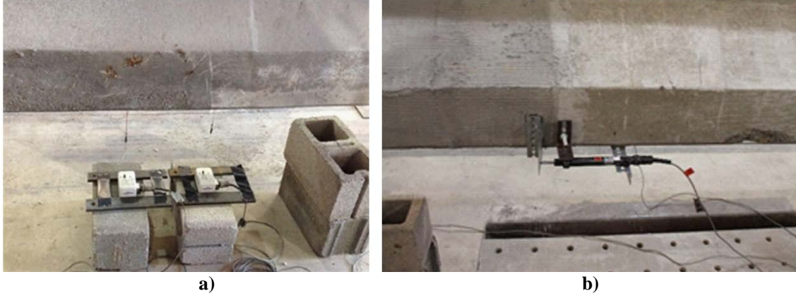
Figure 29. Measurement of a) Displacement Using Wire Potentiometers Below Load Point, b) Slip Between Beam and FRCM Repair Material Using LVDT
