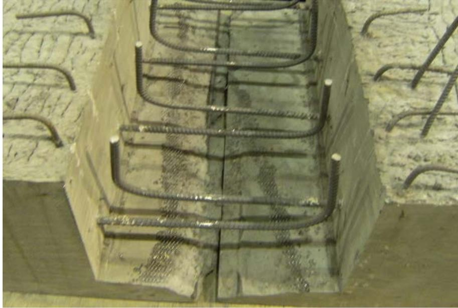
**Figure 16. Trial Specimen With Straight Web, Extended Bars, and Incomplete Flanges**
