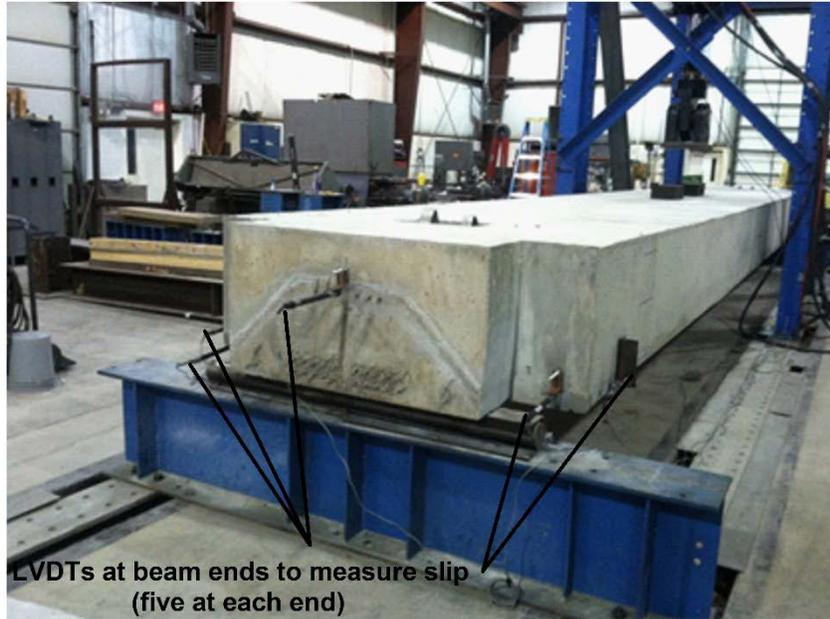
Figure 32. Location of LVDTs at the Ends of the Composite Beam to Measure Slip
