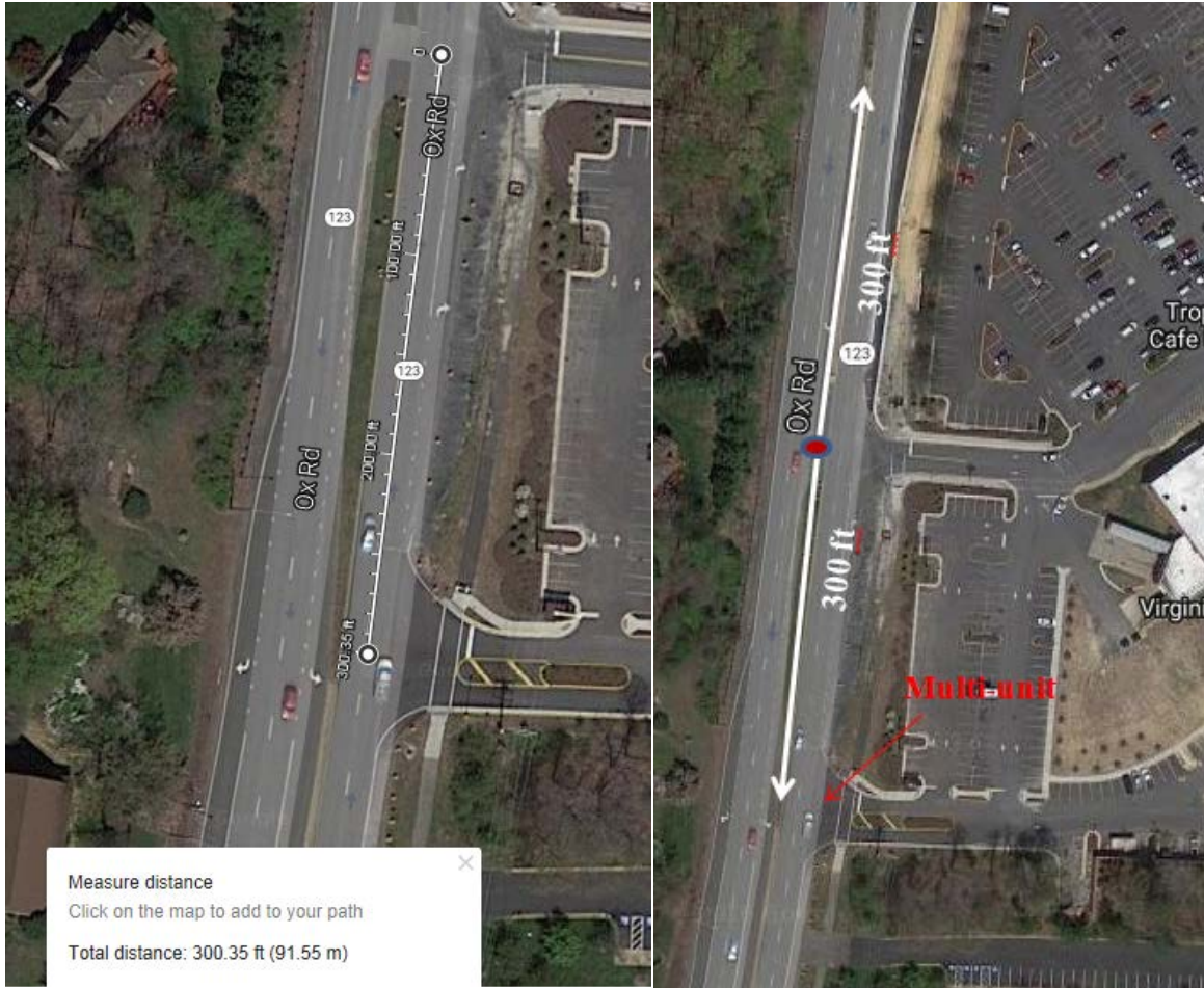
Figure C21. Left: Google Measurement Tool. Right: Single Multi-Unit Entrance Within a 300-Foot Radius of the Commercial Entrance on the Affected Road. Map Data © 2017 Google.
