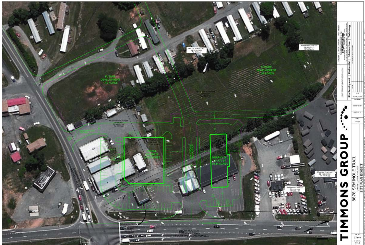
Figure 3. Example of an Exception Site With Proposed Mitigation Measures Near Route 29 (running left to right) and Route 33 (running top to bottom) in Ruckersville (Proctor, 2016). The photograph shows several existing entrances that presently violate spacing standards. The proposed mitigation (green) combines several entrances and moves one farther from the intersection. (In addition to the route names and entrances being labeled, the words within the figure indicate the proposed land uses; for example, the lower left green box indicates that a “retail” development of 14,560 square feet is proposed for that location.) Reprinted with permission of Timmons Group.
