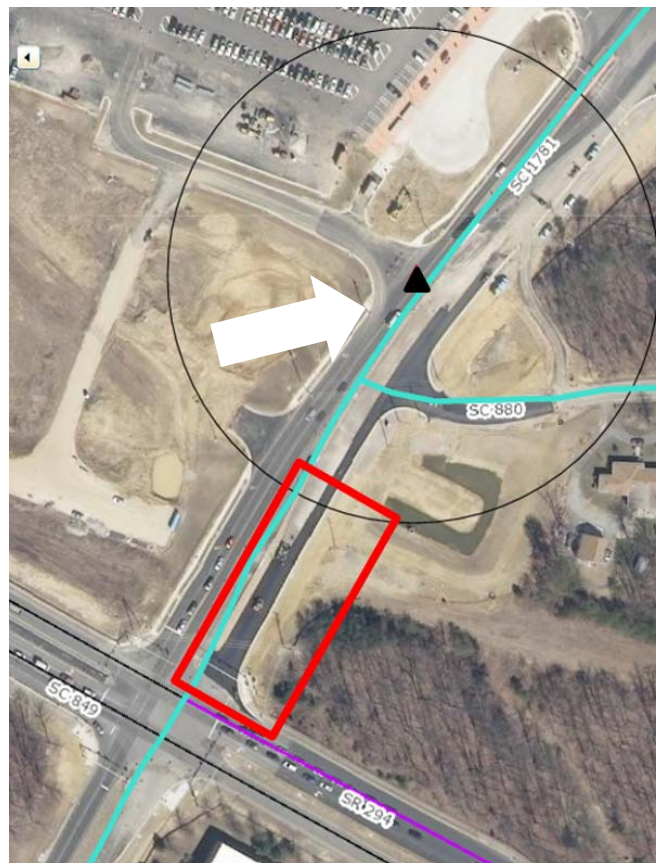
Figure 12. Examples of the Two Methods for Collecting Crashes. The exception site entrance (latitude = 38.65743, longitude = -77.28855) is shown with a black triangle in the upper third of the figure. Method 1 uses a 300-foot buffer (black circle). Method 2 includes Method 1 plus any crashes from that buffer to the center of the existing intersection (red rectangle).
