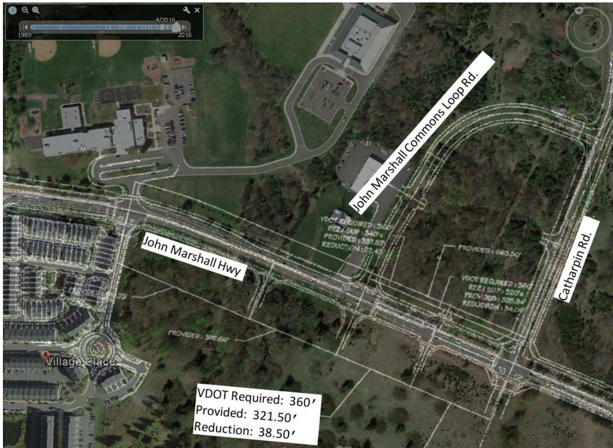
Figure 14. Example of an Exception Request Never Built. Adapted by Nicholas Zugris in 2017 from a 2010 drawing by Barnes and Johnson, LLC, and aerial imagery, © 2017 Google. Because the original text might be illegible, some of this text was manually added by the Virginia Transportation Research Council (in white boxes) in 2018. For example, for two access points, the original text included the 3 lines of information shown in the lowest white box, indicating that those 2 access points had a required spacing distance of 360 ft and a proposed spacing distance of 321.50 ft, which deviates from the standard by 38.50 ft.
