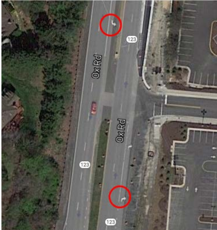
Figure C19. Dedicated Turn Lanes Into the Commercial Entrance From the Affected Road. Map Data © 2017 Google.
