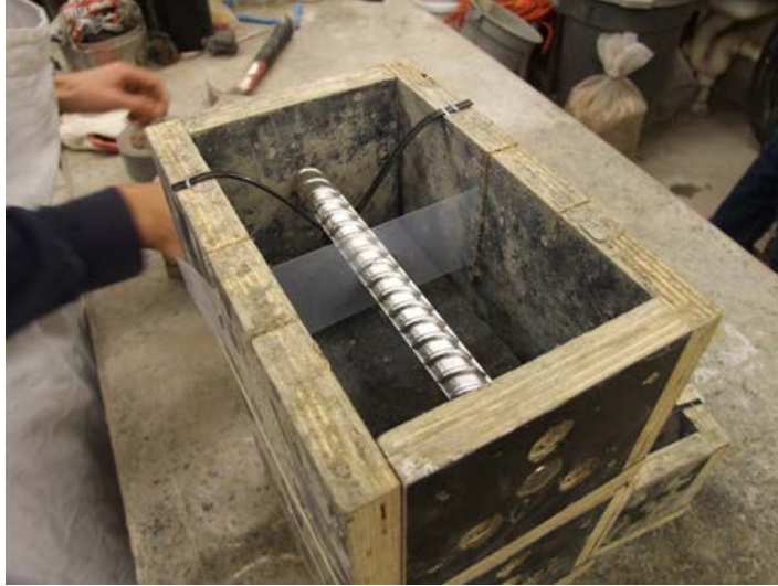
Figure 2. Mold and 1-Ply Shim Construction
