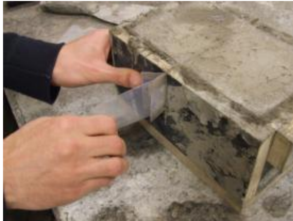
Figure 6. Removing Middle Layer of Multi-Ply Poly Shim First
