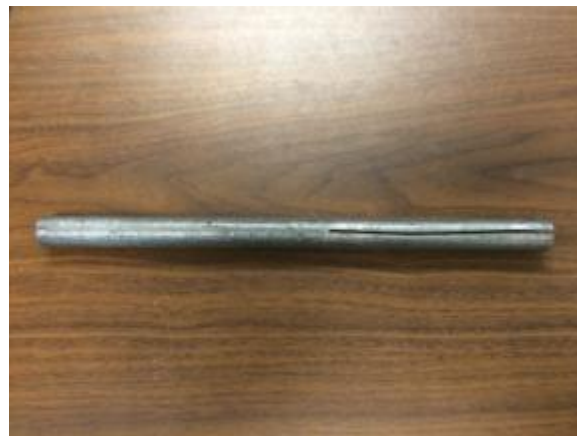
Figure 7. Custom Shim Removal Tool
