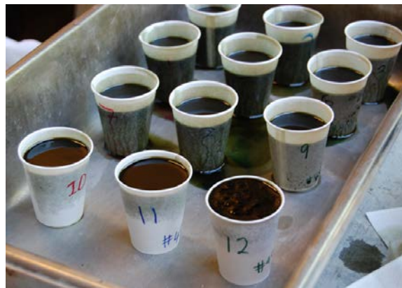
Figure 11. Epoxy Leaking Out of Paper Cups
