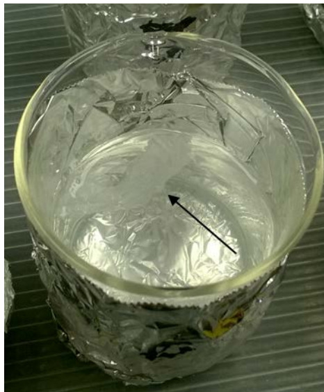
Figure 5. Semisolid Extra Packaging (EP) Specimen (indicated with black arrow). The specimen is still undissolved in water after 24 hours.
