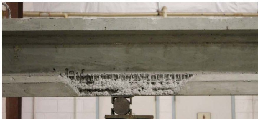
Figure 18. Honeycombing in Three Layers of C-Grid
