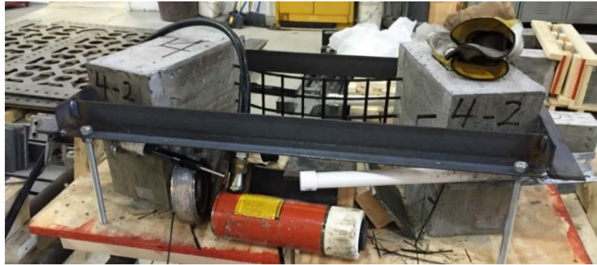
Figure 14. Typical Failure of a Development Length Specimen
