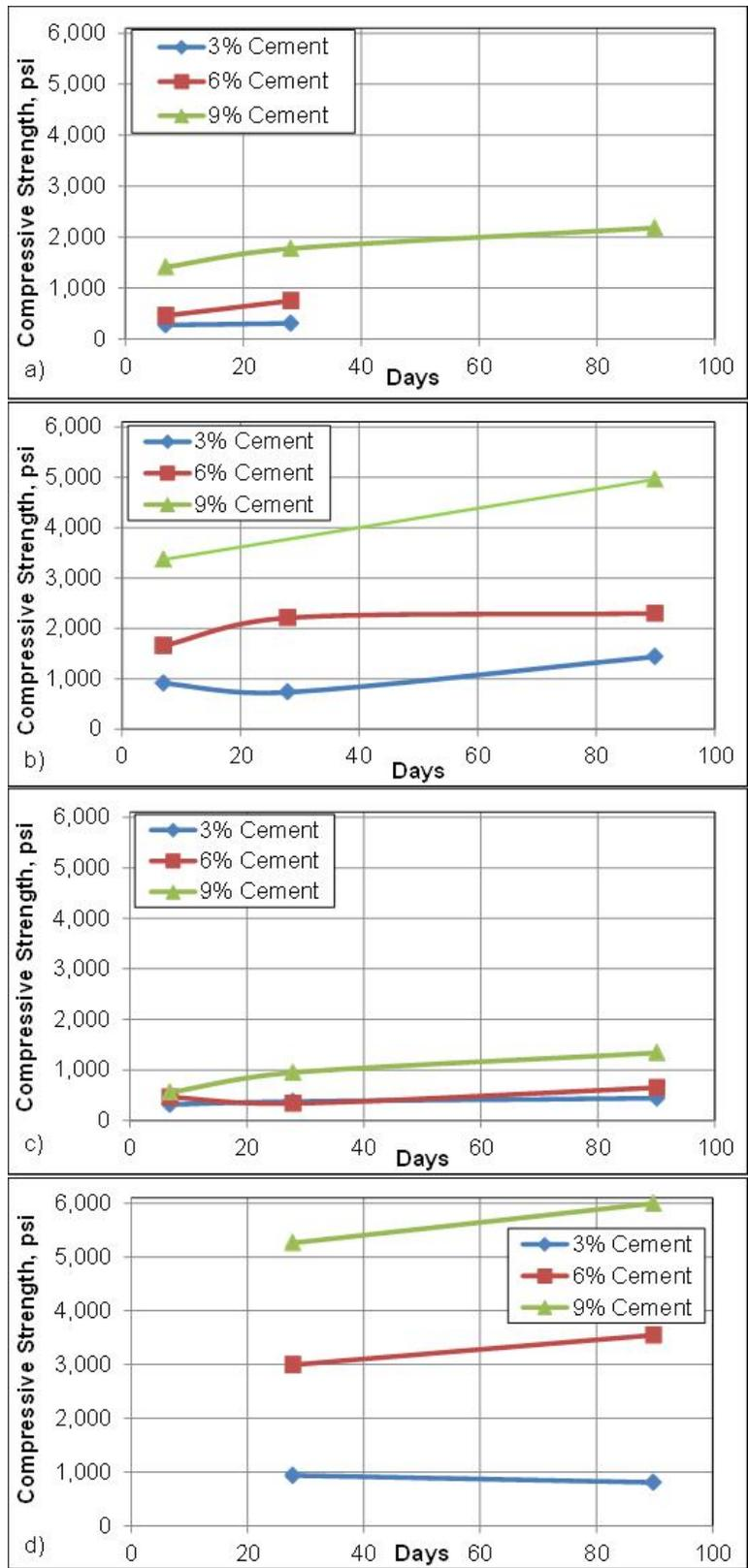
Figure 10. Compressive Strength Gain With Age in Laboratory-Prepared CTA: (a) Middle Ground Boulevard; (b) Nimmo Parkway; (c) Fredericksburg, Route 208; (d) Staunton limestone. CTA = cement-treated aggregate.
