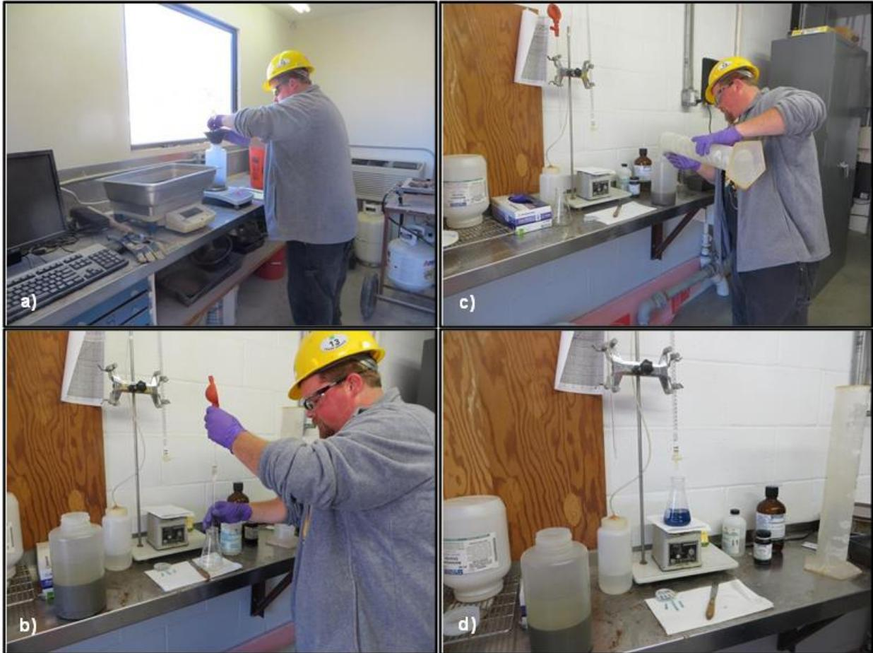
**Figure 2. Titration Test for Cement Content: (a) weighing CTA sample for testing; (b) adding ammonium chloride to sample; (c) transferring solution from sample for titration; (d) titration completed. CTA = cement-treated aggregate.**
