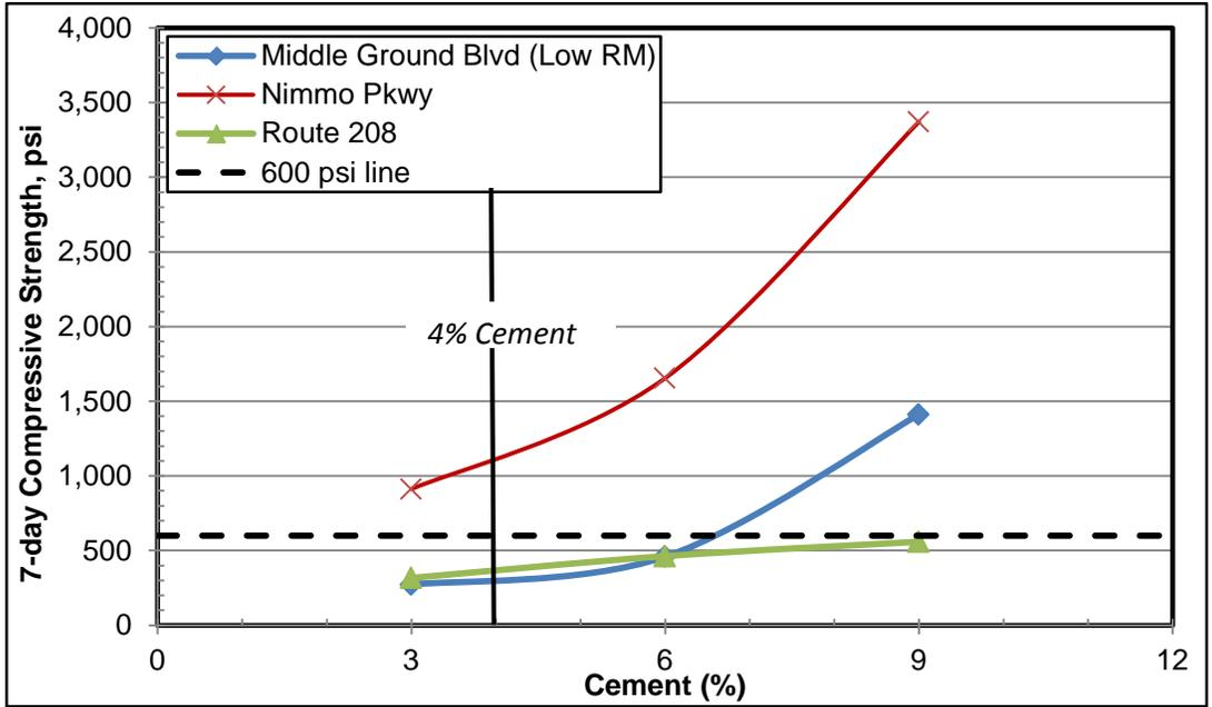
Figure 8. 7-Day Compressive Strength of CTA Produced With Vibratory Hammer. CTA = cement-treated aggregate; RM = resilient modulus.
