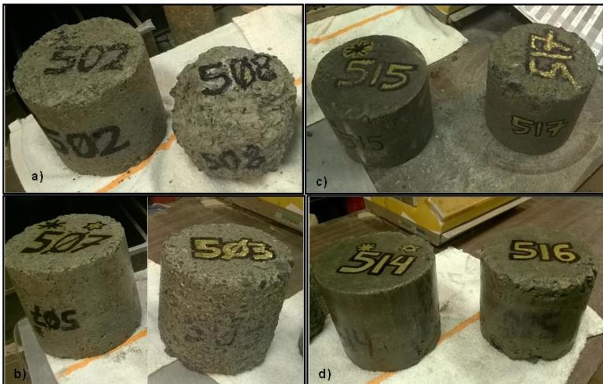
**Figure 18. Freeze-Thaw and Wet-Dry Test Samples After 12 Cycles of Testing: (a) Source A freeze-thaw; (b) Source A wet-dry; (c) Source B freeze-thaw; (d) Source B wet-dry. Source A with 7-day compressive strength of 550 psi, and Source B with 7-day compressive strength of 1,050 psi. CTA = cement-treated aggregate.**
