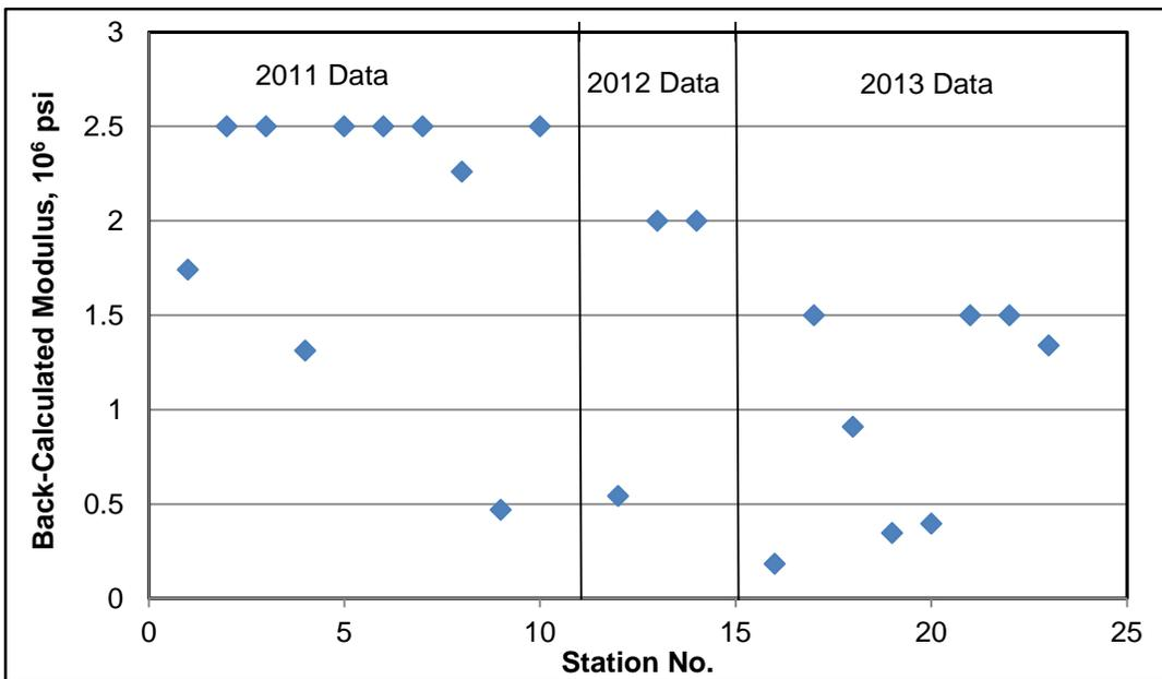
Figure 13. CTA Back-Calculated Layer Modulus (Route 208). CTA = cement-treated aggregate.
