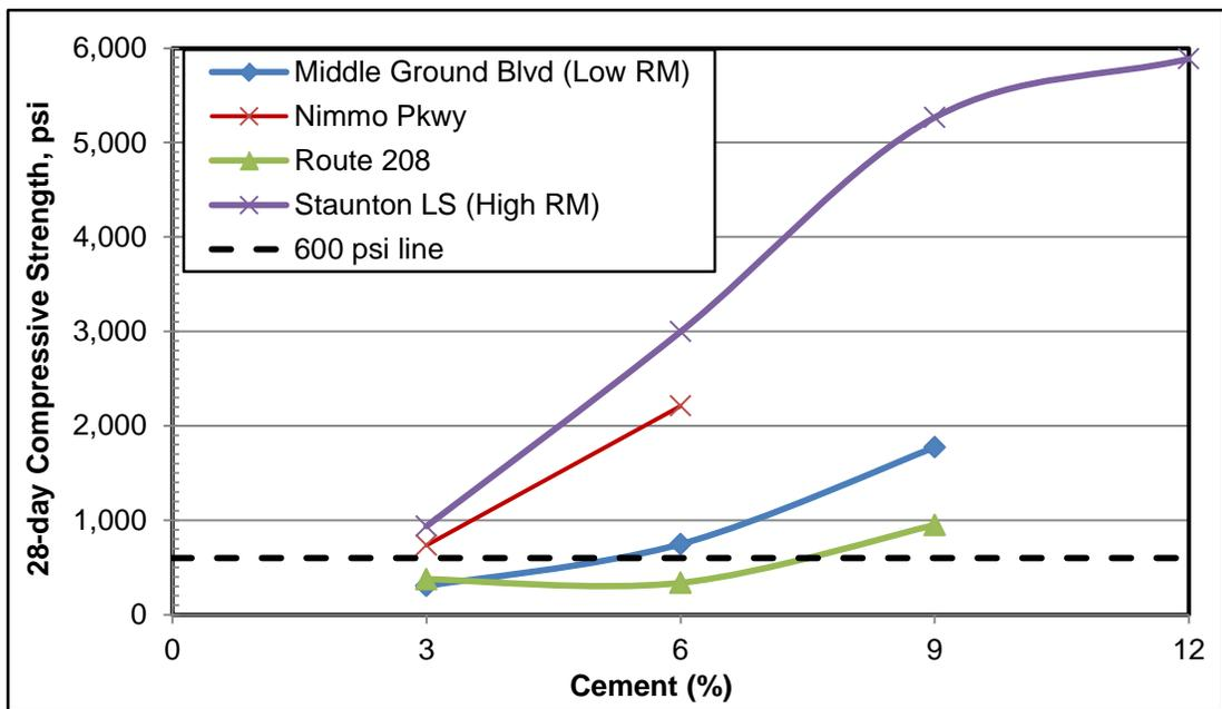
Figure 9. 28-Day Compressive Strength of CTA Produced With Vibratory Hammer. CTA = cement-treated aggregate; RM = resilient modulus.
