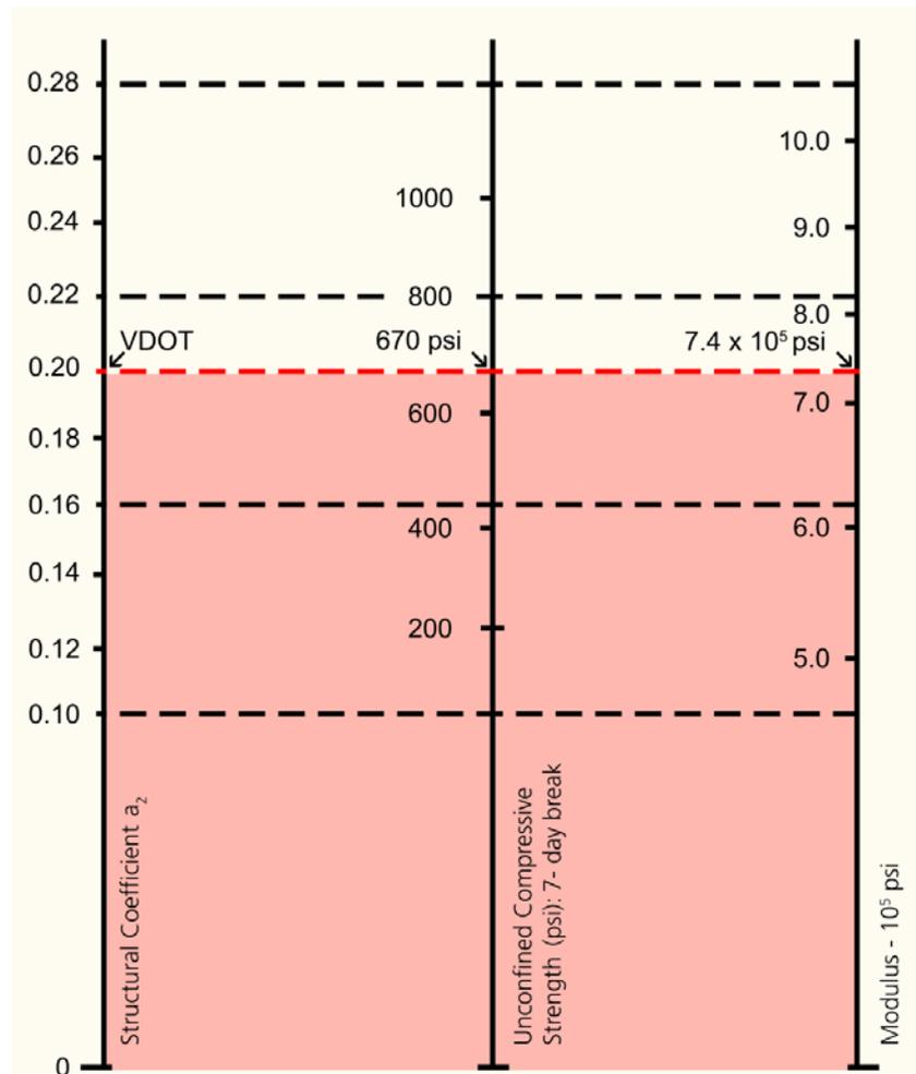
**Figure 16. 7-Day Compressive Strength and Elastic Modulus of CTA Corresponding to Layer Coefficients (AASHTO, 1993). CTA = cement-treated aggregate; VDOT = Virginia Department of Transportation.**
