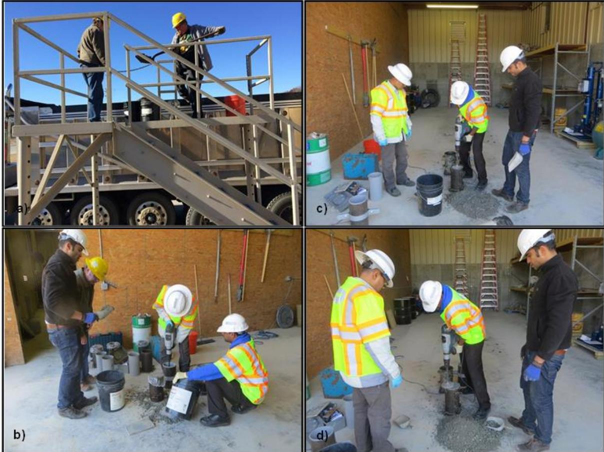
**Figure 4. Preparation of CTA Cylinder Using Vibratory Hammer: (a) sampling from haul truck at plant; (b) compacting cylinder in plastic mold with steel sleeve; (c) sample compaction in steel mold; (d) leveling off samples in mold. CTA = cement-treated aggregate.**
