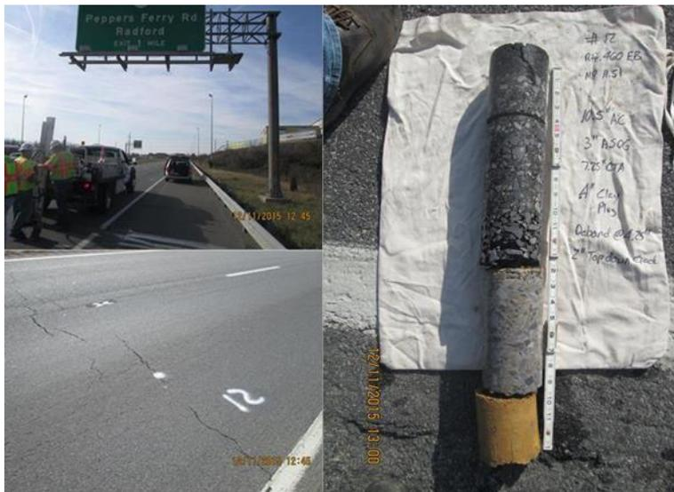
Figure 15. U.S. 460 in Salem, Top-Down Transverse Crack
