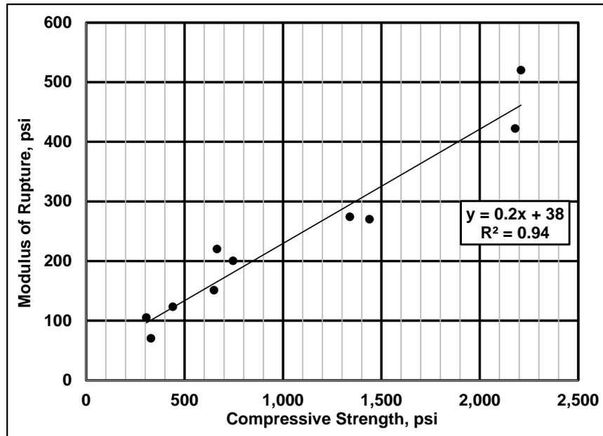
Figure 20. Relationship Between CTA Compressive Strength and Modulus of Rupture. CTA = cement-treated aggregate.
