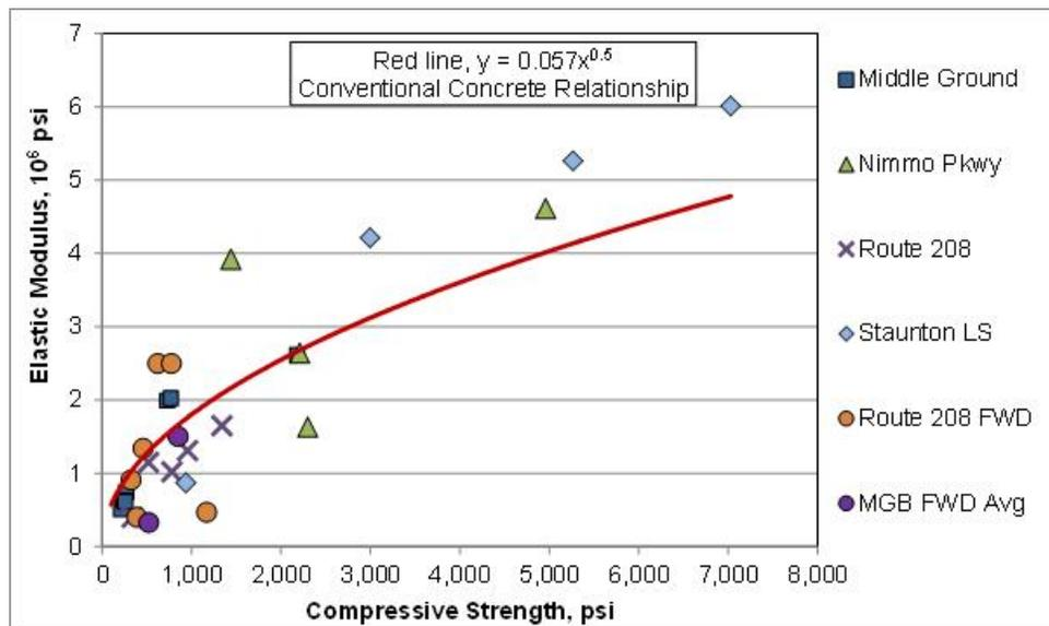
Figure 19. Relationship Between Compressive Strength and Elastic Modulus. Middle Ground = Middle Ground Boulevard; LS = limestone; FWD = falling weight deflectometer.
