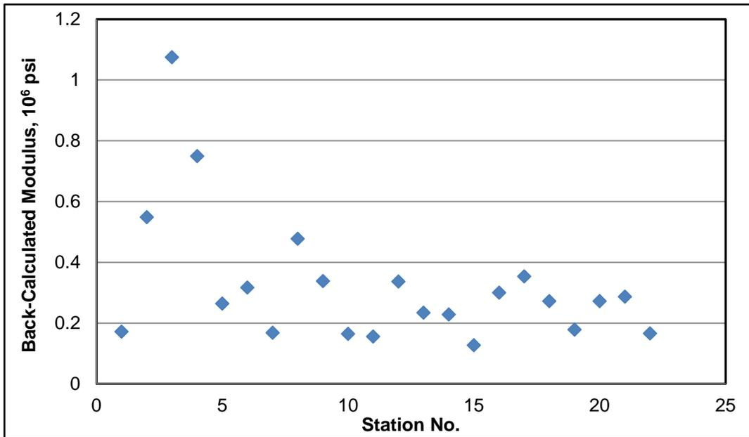
Figure 11. CTA Back-Calculated Layer Modulus at 4 Months After Construction (Middle Ground Boulevard). CTA = cement-treated aggregate.
