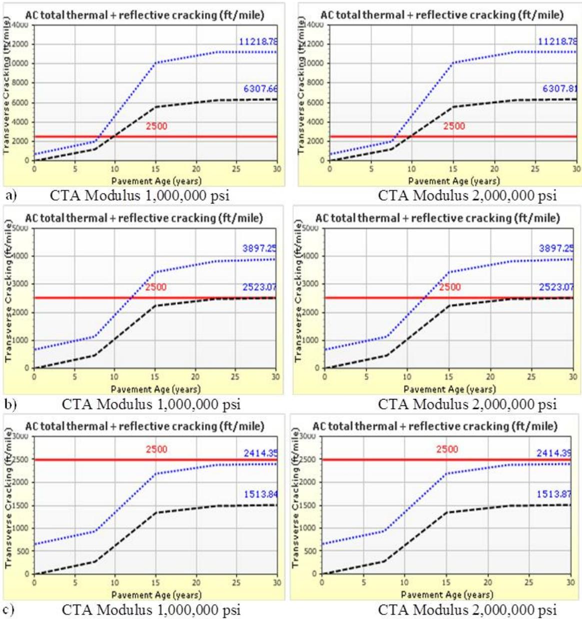
Figure 7. Transverse Crack Reflection at Different Pavement Ages With Seed Crack Spacing: (a) 6 ft; (b) 15 ft; (c) 25 ft. Red line = threshold value; blue line = specified reliability; black line = 50% reliability. CTA = cement-treated aggregate; AC = asphalt concrete; modulus = elastic modulus.
