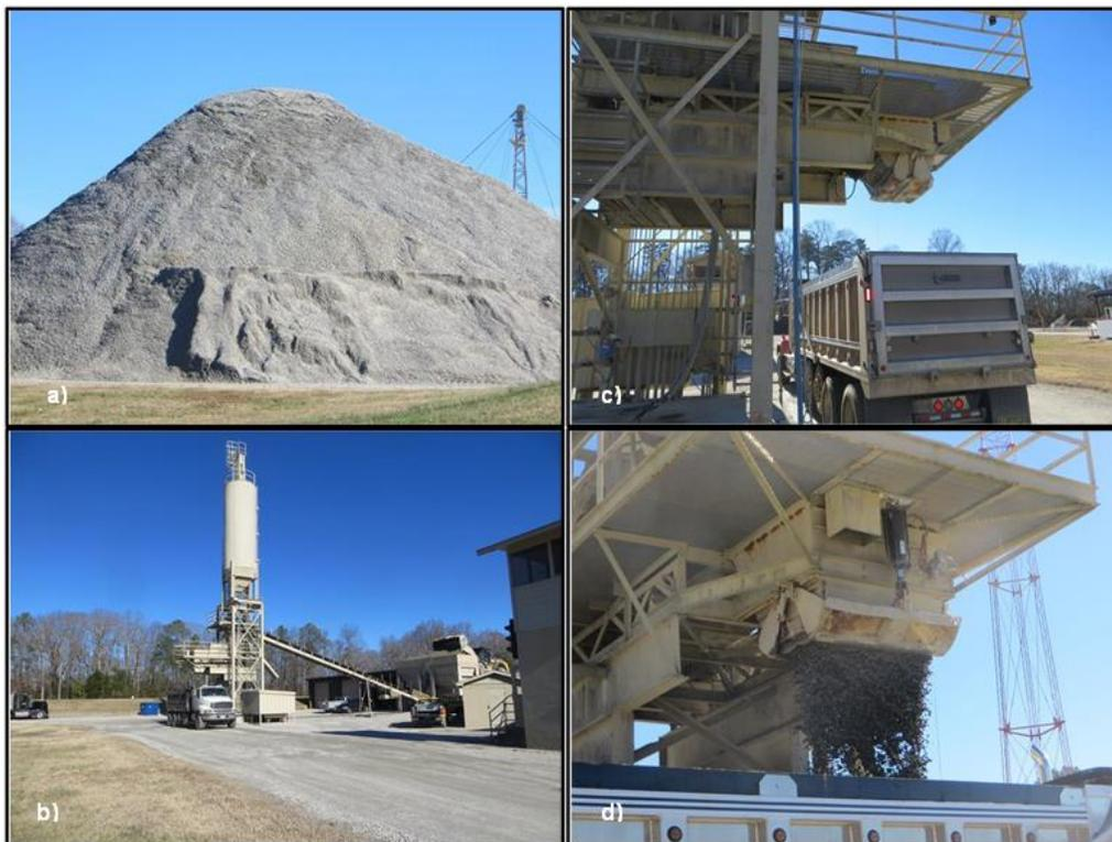
Figure 1. CTA Plant for Middle Ground Boulevard Project: (a) VDOT 21A aggregate pile; (b) pugmill and haul truck; (c) pugmill gate closed; (d) gate open for loading truck. CTA = cement-treated aggregate.
