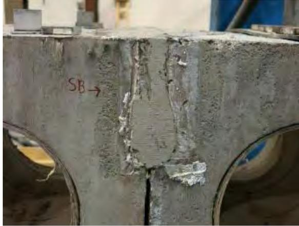
**Figure 13. Hardened Shear Key From First Specimen Tested**
