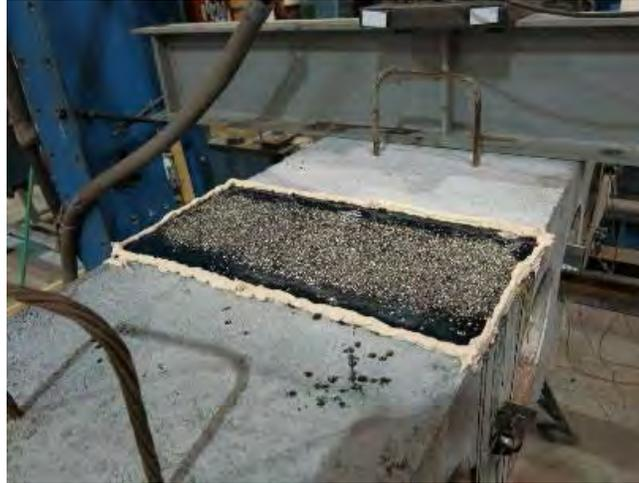
**Figure 14. Photograph of Kevlar-Epoxy Joint With Coarse Sand**
