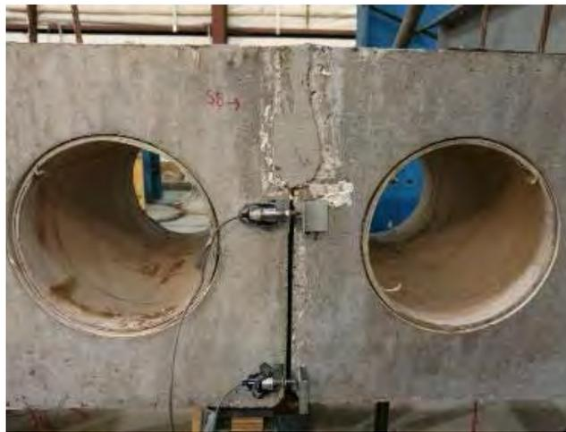
**Figure 24. Photograph Showing Instrumented Joint**
