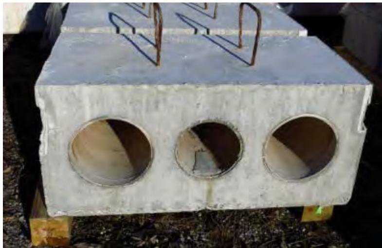
**Figure 12. Finished Voided Slab Specimen**
