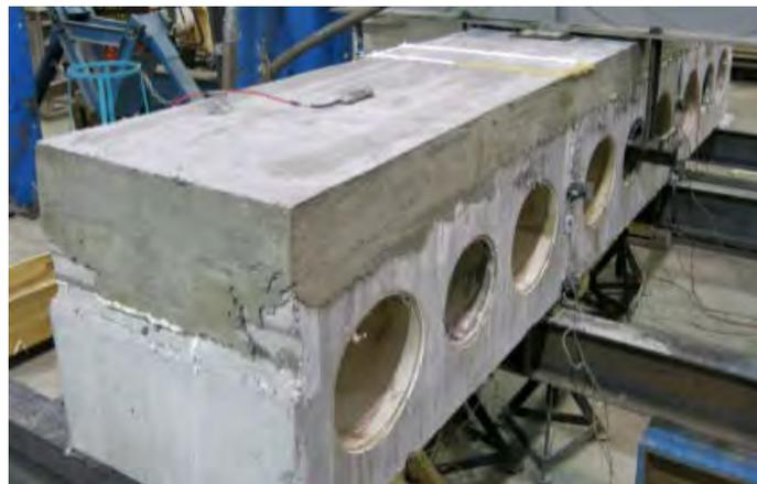
**Figure 19. Concrete Topping on Sub-Assemblage**
