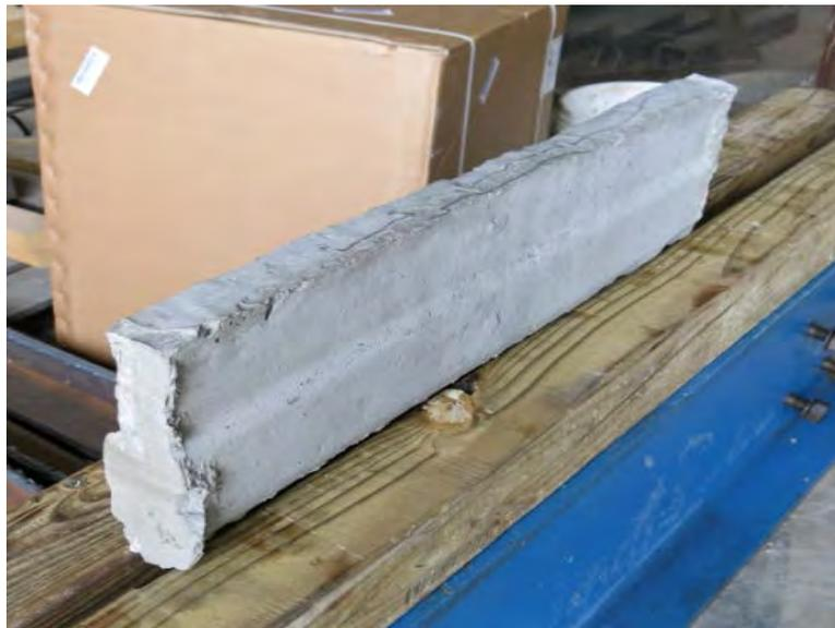
**Figure 28. Intact Shear Key After Failure of Bonded Connection**
