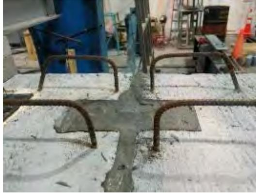
**Figure 16. Photograph of Cured UHPC Joint**
