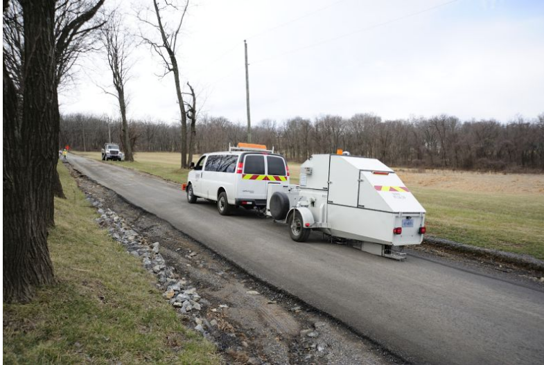
Figure 12. Falling Weight Deflectometer at Test Section
