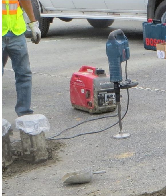
Figure 2. Vibrating Hammer to Prepare RCC Cylinders (Hossain and Ozyildirim, 2015). RCC = roller-compacted concrete.
