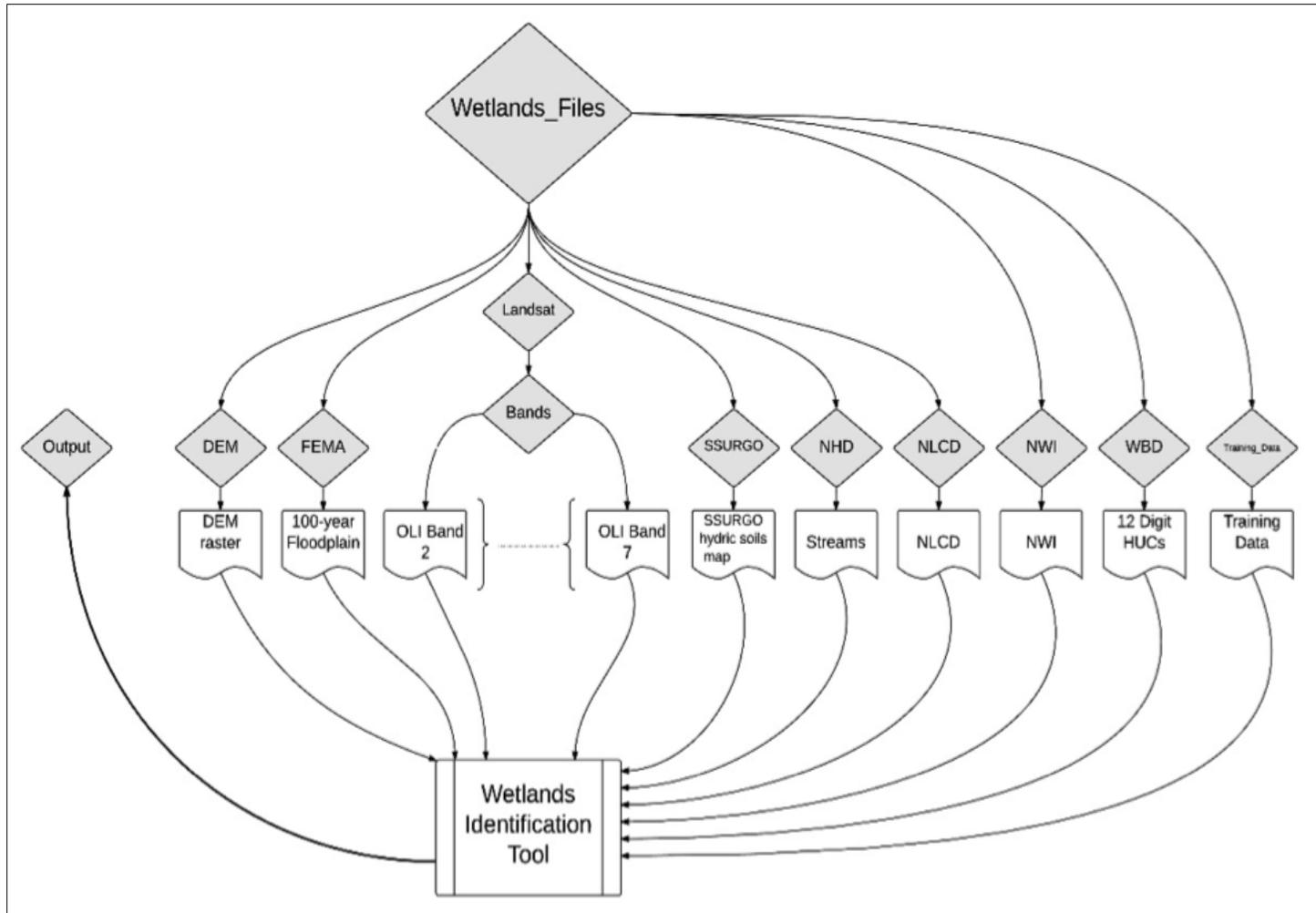
Figure 3. Image of Data Structure Hierarchy Required by Tool
