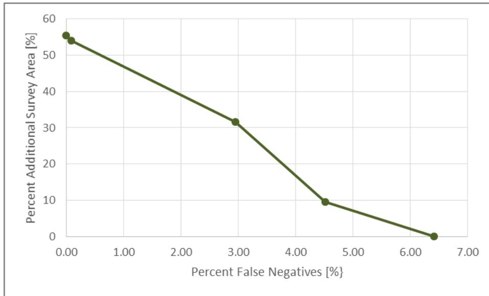
**Figure 13. Relationship Between Level of Certainty in False Negative Predictions and Increased Area That Must Be Investigated Using More Detailed Wetland Identification Procedures**
