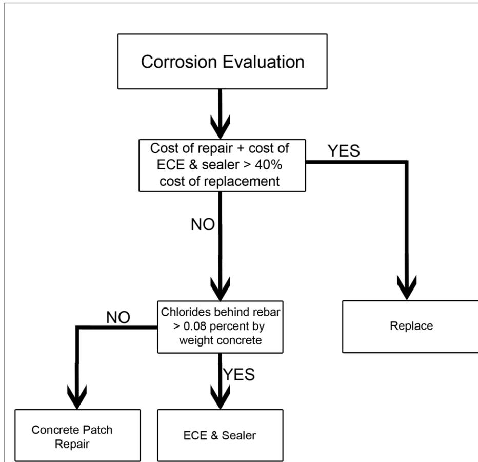
**Figure 20. Repair Method Recommended by VDOT for the Eleven I-95 Bridges in Richmond, Virginia**
