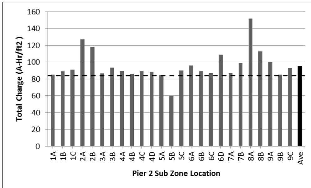
Figure 24. Total Charge Passed During ECE Treatment on Pier 2 of I-95 Bridge Over Hermitage Road. Sub-zones that did not meet the criteria for charge did meet the chloride level requirement. ECE = electrochemical chloride extraction.
