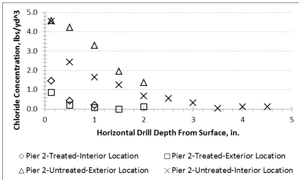
Figure 15. Pier 2 of 5th Street Extended Bridge Showing Chloride Concentrations in Treated and Untreated Columns After 19 Years. Figure 4 shows interior location, indicated by “I,” and exterior location, indicated by “E,” of the pier.
