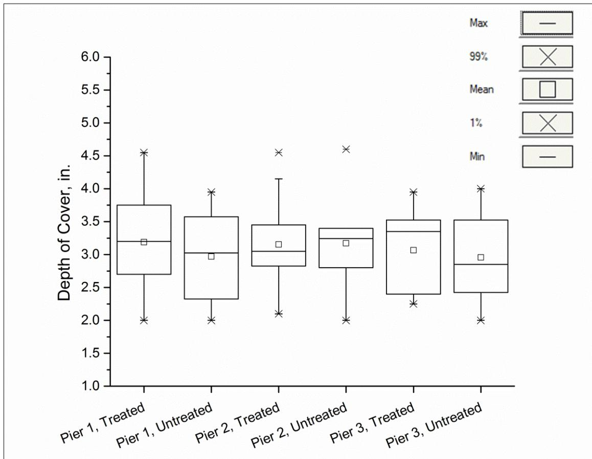
Figure 18. Depth of Cover Measurements on Piers of 5th Street Extended Bridge
