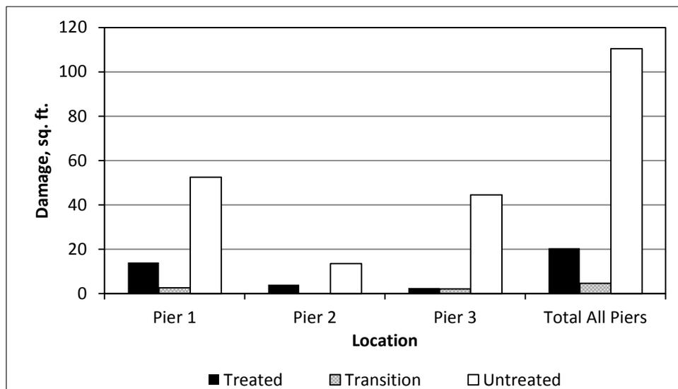
Figure 9. Comparison in Performance for Each Pier and General Performance for All Piers Combined Based on 2012 Evaluation Results for 5th Street Extended Bridge
