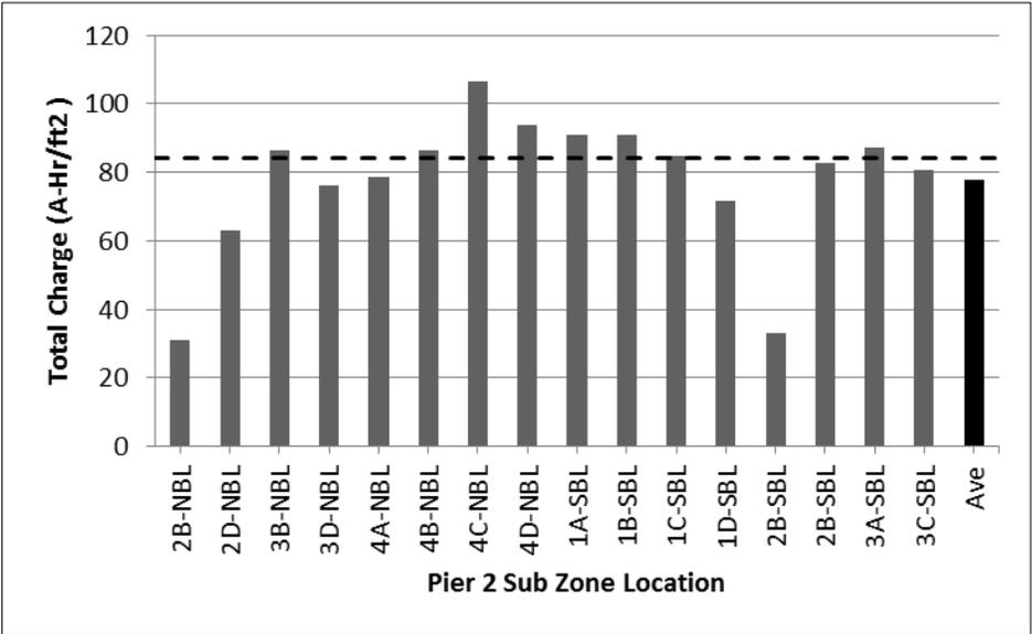
Figure 41. Total Charge Passed During ECE Treatment on Pier 2 Under I-95 Bridge Over Overbrook Road. Sub-zones that did not meet the criteria for charge did meet the chloride level requirement. ECE = electrochemical chloride extraction.
