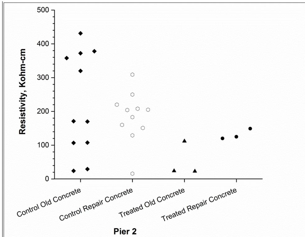
Figure 16. Resistivity Measurements on Cap of Pier 2 of 5th Street Extended Bridge
