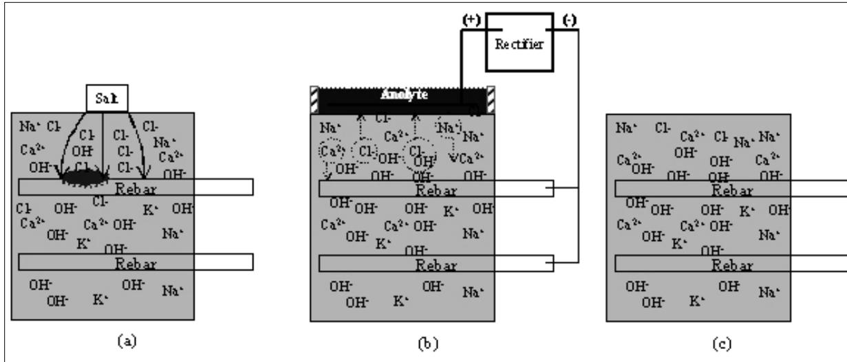
**Figure 1. Illustration of Corrosion Initiation Followed by ECE Treatment on Horizontal Surface. (a) Salt penetrates uncontaminated concrete and chloride threshold is exceeded; corrosion is initiated. (b) A temporary ECE system is constructed, which reduces chloride concentration at the steel while increasing the alkalinity. (c) ECE is complete and equipment is removed. ECE = electrochemical chloride extraction.**
