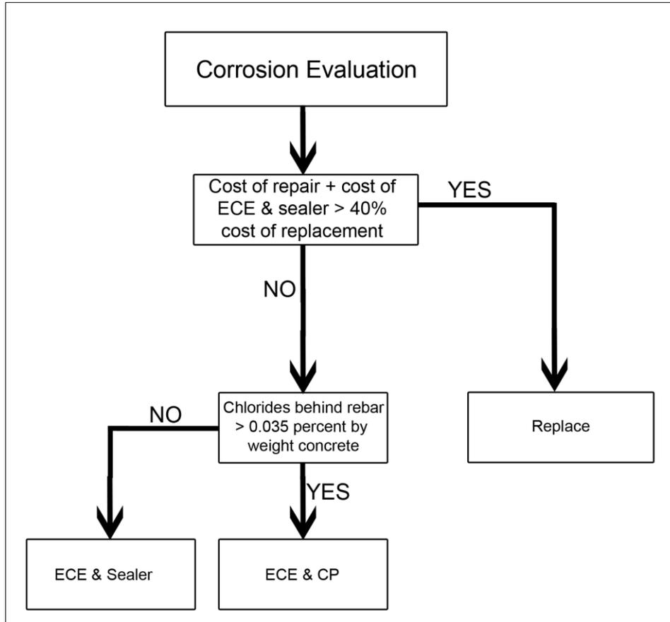
**Figure 19. Repair Method Proposed by Corrosion Services Consultant for the Eleven I-95 Bridges in Richmond, Virginia**
