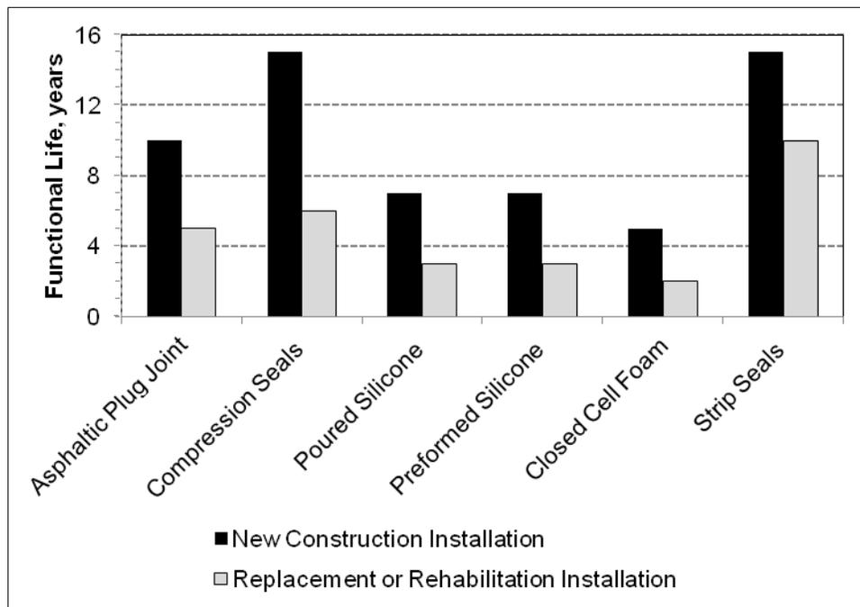
**Figure 5. Comparative Results From the Northeast Bridge Preservation Partnership Study on the Functional Life of Bridge Joints. Based on data from Milner and Shenton (2015).**
