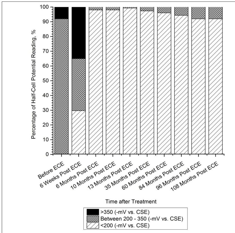
**Figure 6. Percent Change in Average Half-cell Reading Over Time for 1989 ECE-Treated Substructure Faces on Burlington Bay Skyway. Based on data from Pianca et al. (2003). ECE = electrochemical chloride extraction.**
