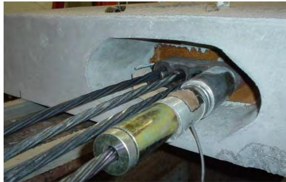
Figure 18. Load Cell on the Dead End of a Strand During Stressing
