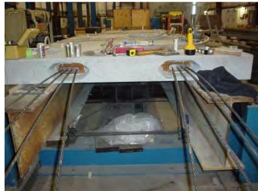
**Figure 36. Four Strands per Duct in the 340 psi Post-Tensioned Connection**
