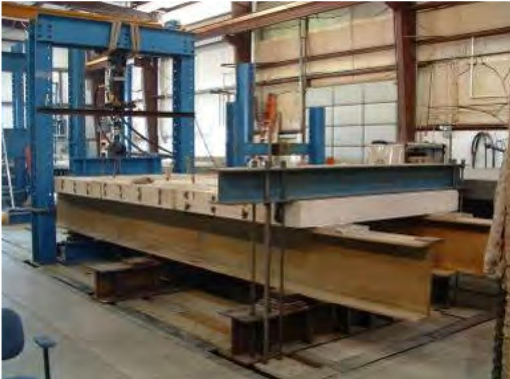
**Figure 9. Panel-to-Panel Connection Test Setup**
