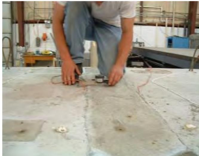
**Figure 21. Taking DEMEC Reading**
