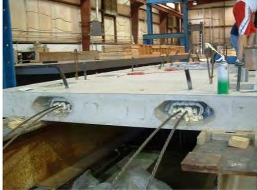
**Figure 35. Two Strands per Duct in the 167 psi Post-Tensioned Connection**
