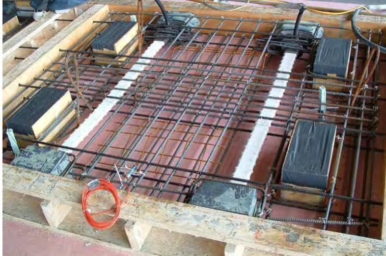
**Figure 12. Installing the Vibrating Wire Gauges in the Panel**
