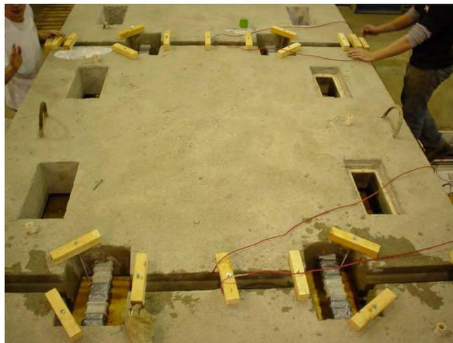
Figure 65. Pocket Layout on the Test Panels
