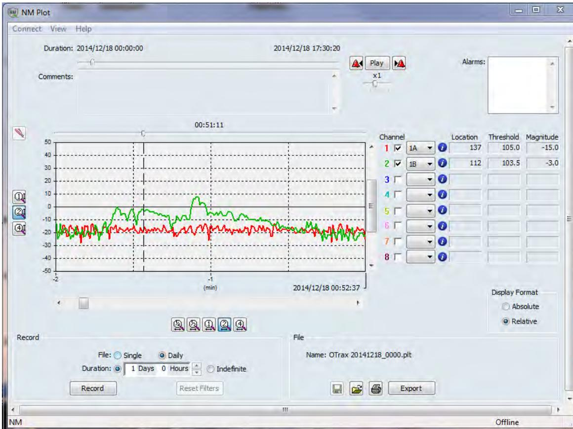
Figure 11. Example of NM Plot Tool Used for Identifying Real-Time Cable Crossing Events. The signal response from both sides of the cable is displayed.
