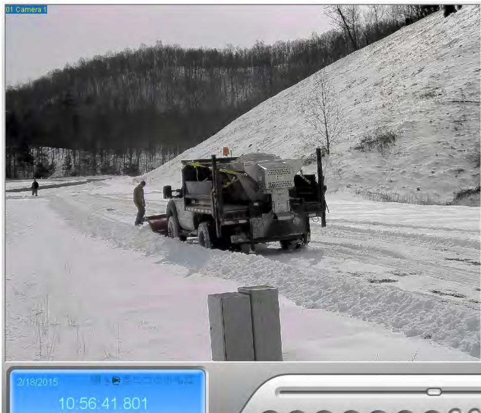
**Figure 23. Maintenance Truck Plowing Snow Over Cable**
