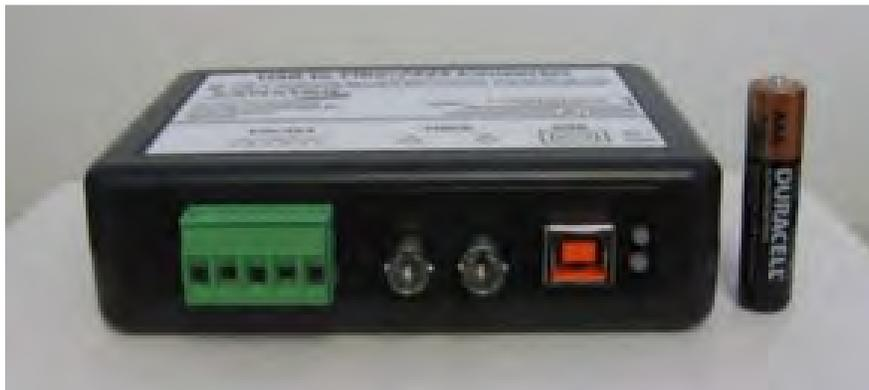
**Figure 9. Network Interface Unit (NIU) Used for Establishing Network Communication**
