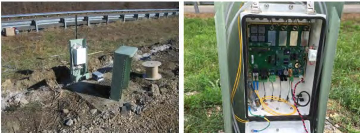
**Figure 7. Weatherproof Processor Enclosure Mounted Inside Telecom Enclosure (*left*) and Processor Board Installed Inside Weatherproof Enclosure (*right*). White tamper switch pictured to the right.**
