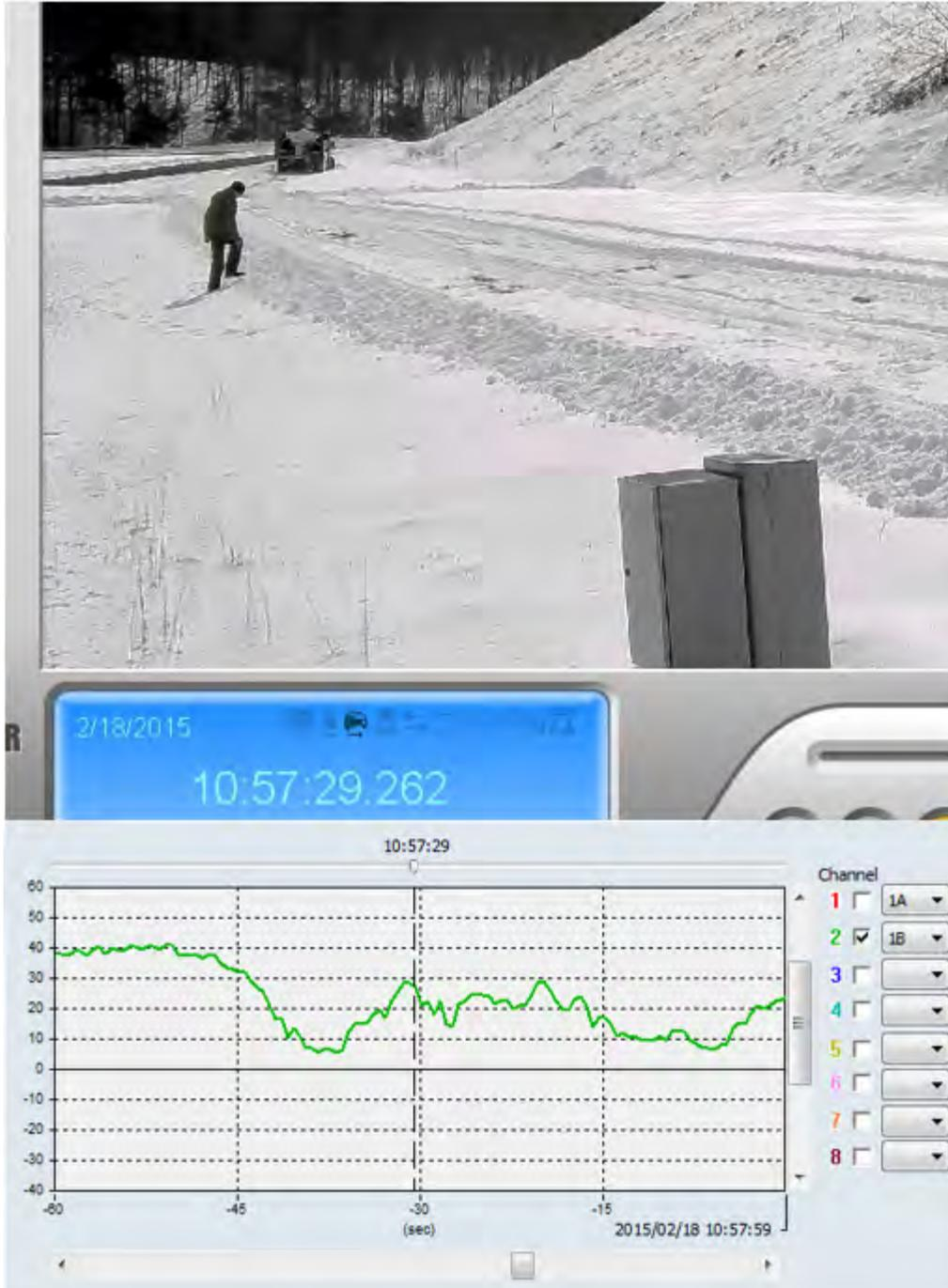
**Figure 24. Crossing Performed Shortly After Additional Snow Was Plowed Over Cable (*top*) and Corresponding Detection Signal (*bottom*).**
