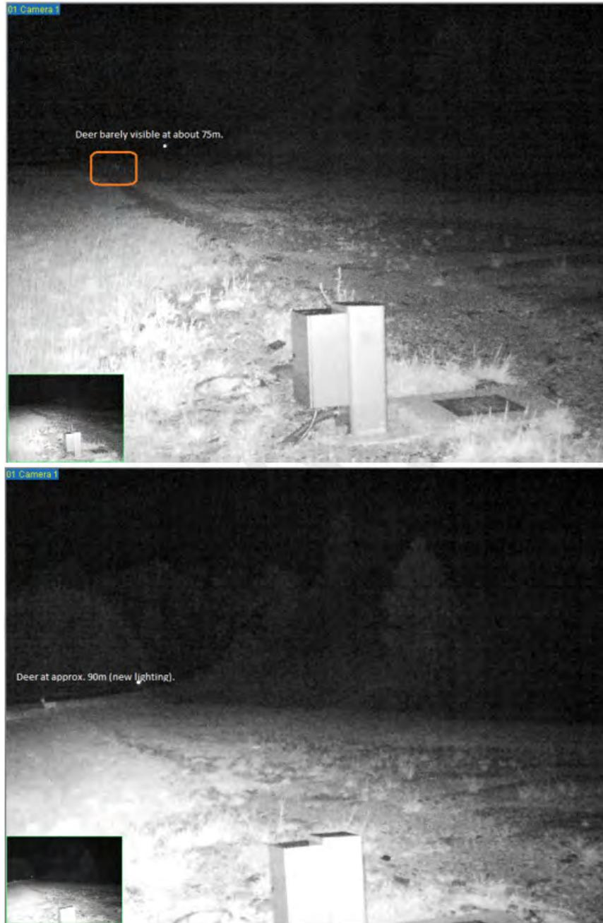
Figure 14. Improved Site Illumination After Installing Additional NIR Illuminators (bottom)
