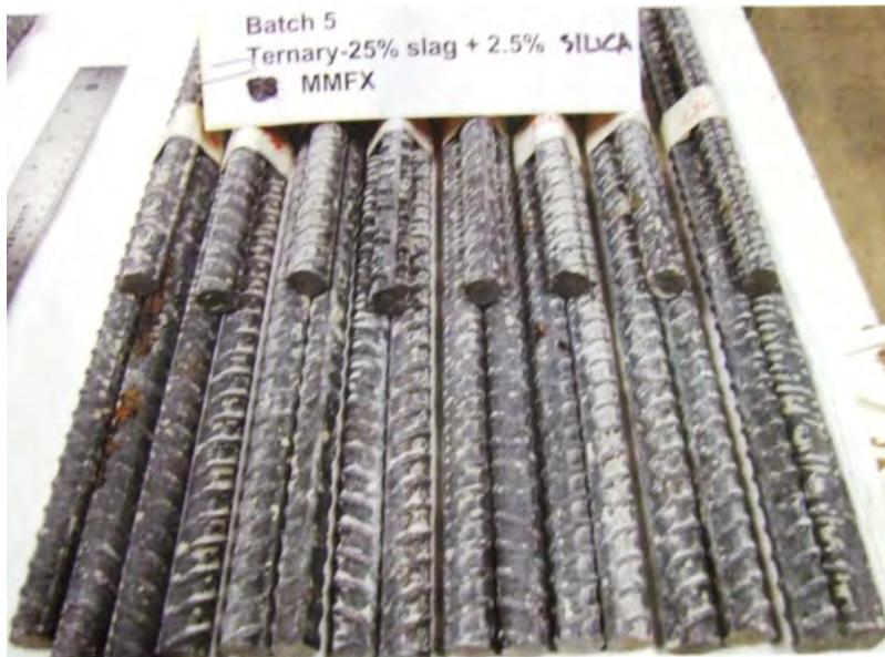
**Figure 7. 72.5% PC + 25% Slag + 2.5% SF Ready-Mixed Batch**
