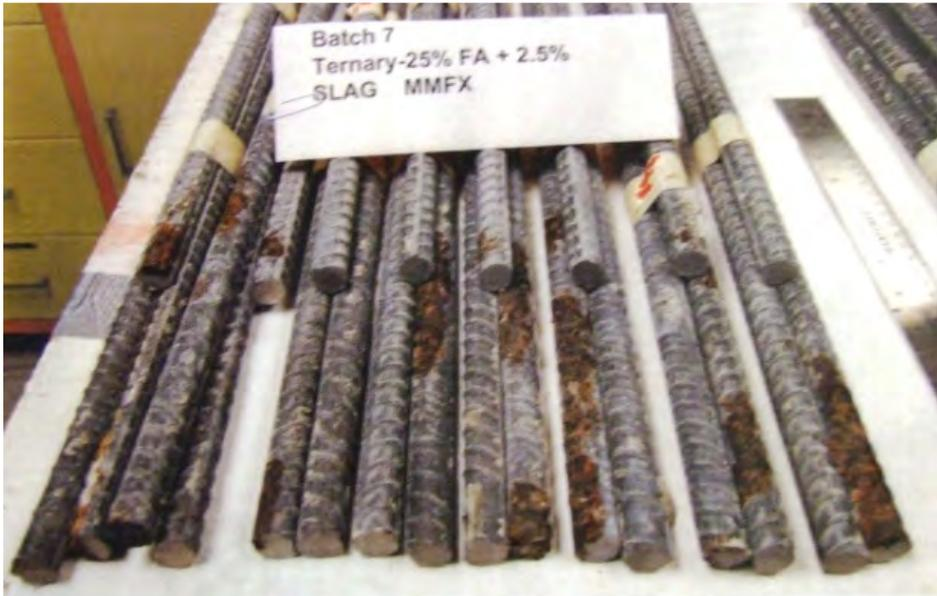
**Figure 9. 50% PC + 25% FA + 25% Slag Ready-Mixed Batch**
