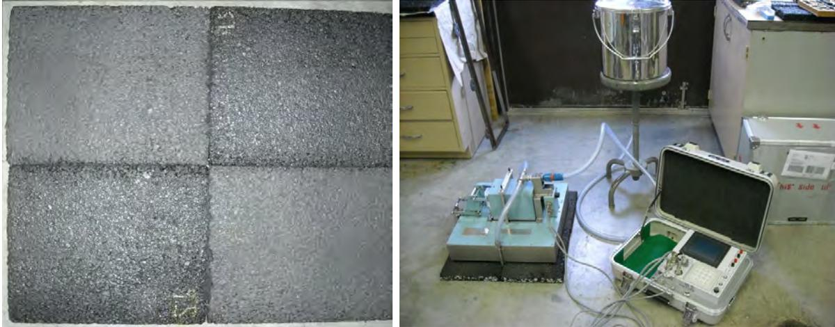
**Figure 3. Dynamic Friction Testing of Asphalt Concrete Slabs in the Laboratory. Left, the slab arrangement for the SM-9.5AL mixture depicting the slabs polished for 100K wheel passes with (upper left / bottom right) and without the epoxy/sand applied to the tires.**
