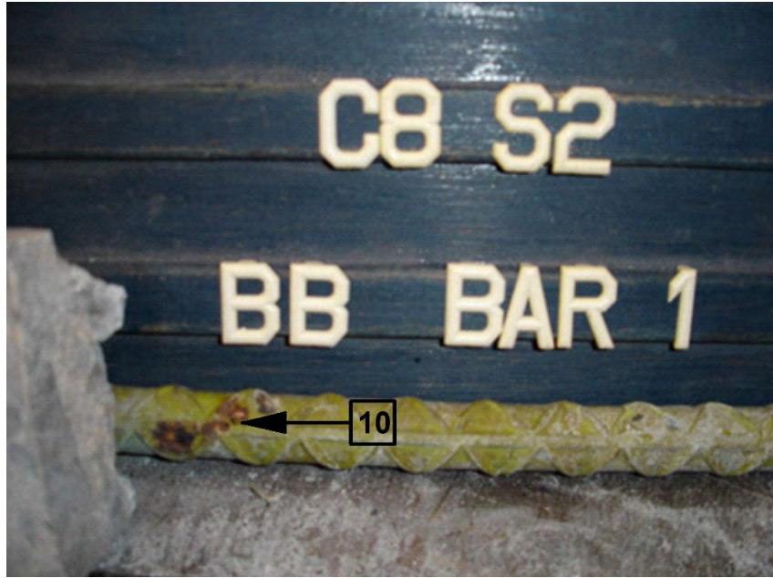
Figure 31. C8-S2 Bottom Bar 1 Without Concrete
