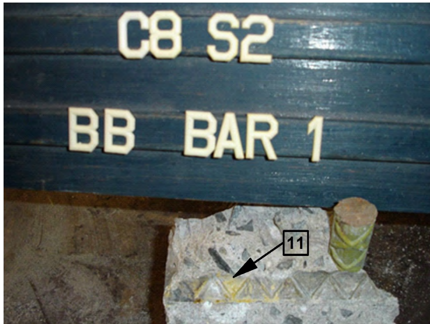
Figure 32. C8-S2 Bottom Bar 1 After Removing Bar
