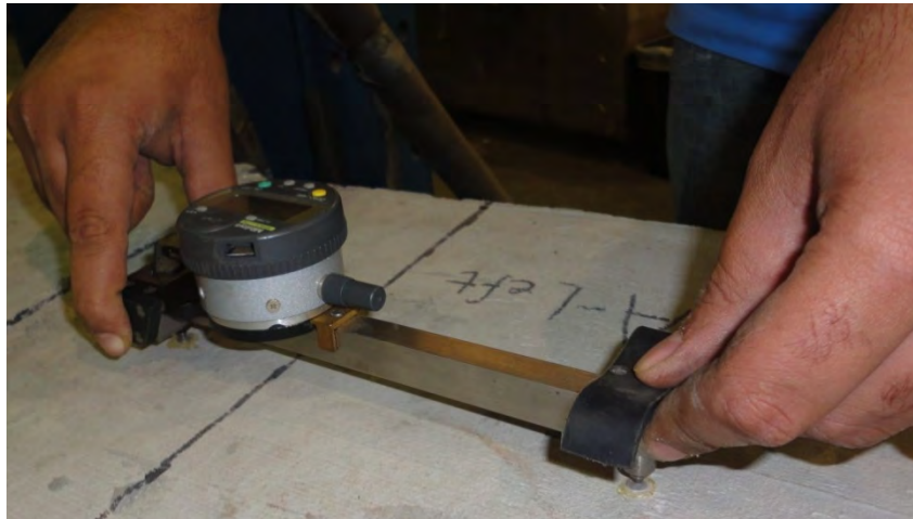
Figure 11. A DEMEC Gage Measuring DEMEC Points
