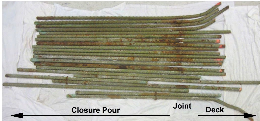
Figure 33. Corrosion Extent of Extracted ECR Bars
