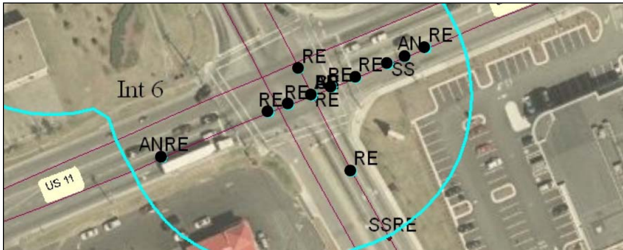
Figure 3. Crashes at Intersection 6 in Roanoke County. RE = rear-end crash; AN = angle crash; SS = sideswipe crash.
