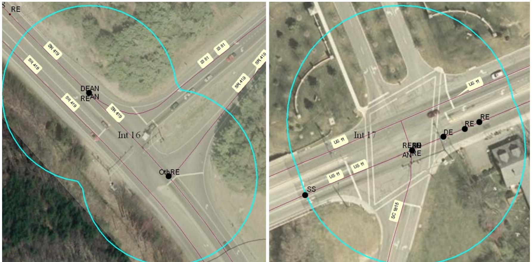
Figure 9. Intersections Necessitating Review of Crash Report (Form FR300). Left: Intersection 16; right: Intersection 17. DE = deer, AN = angle, RE = rear-end, Oth = other, US = U.S. Highway, SR = State Route, SC = Secondary Route.
