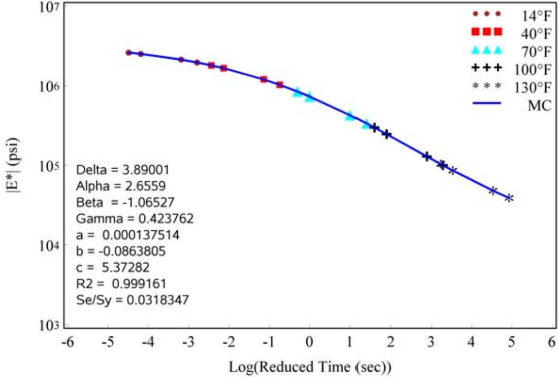
Figure 1. Sample  $|E^*|$  Master Curve Constructed Using MEPDG Software for Mixture 08-1055D
