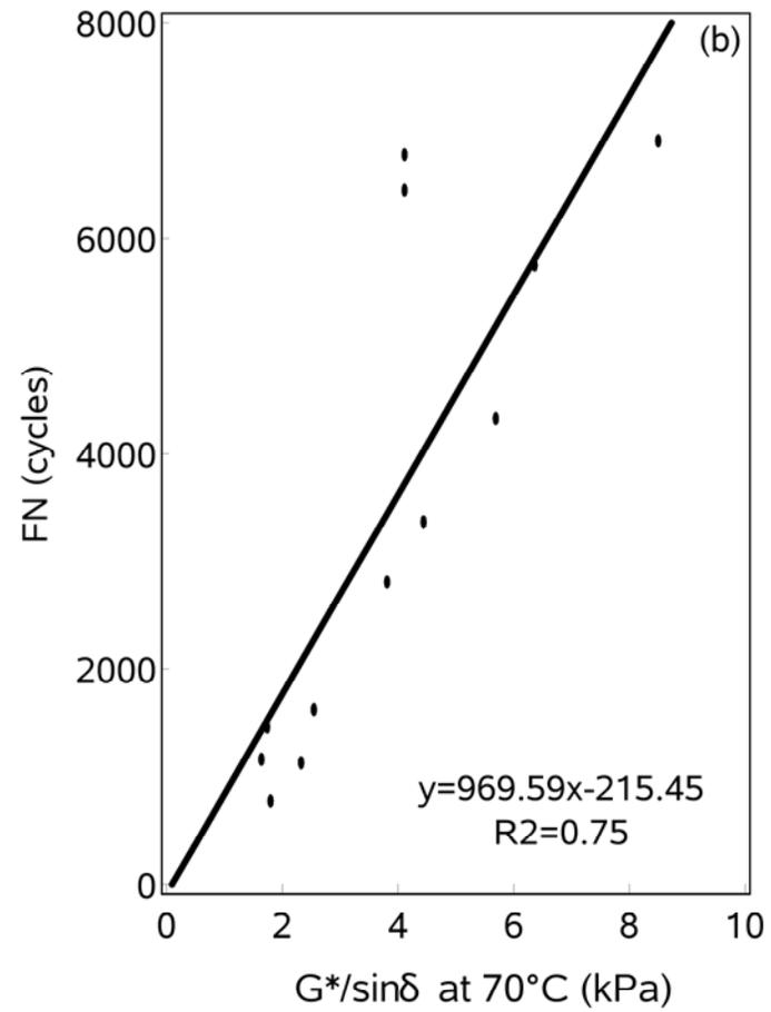
**Figure 10. Relationship Between  $G^*/\sin\delta$  and Rutting.** APA rut depth appears to be insensitive to binder stiffness. Note that  $G^*/\sin\delta$  data were obtained from recovered binders.
