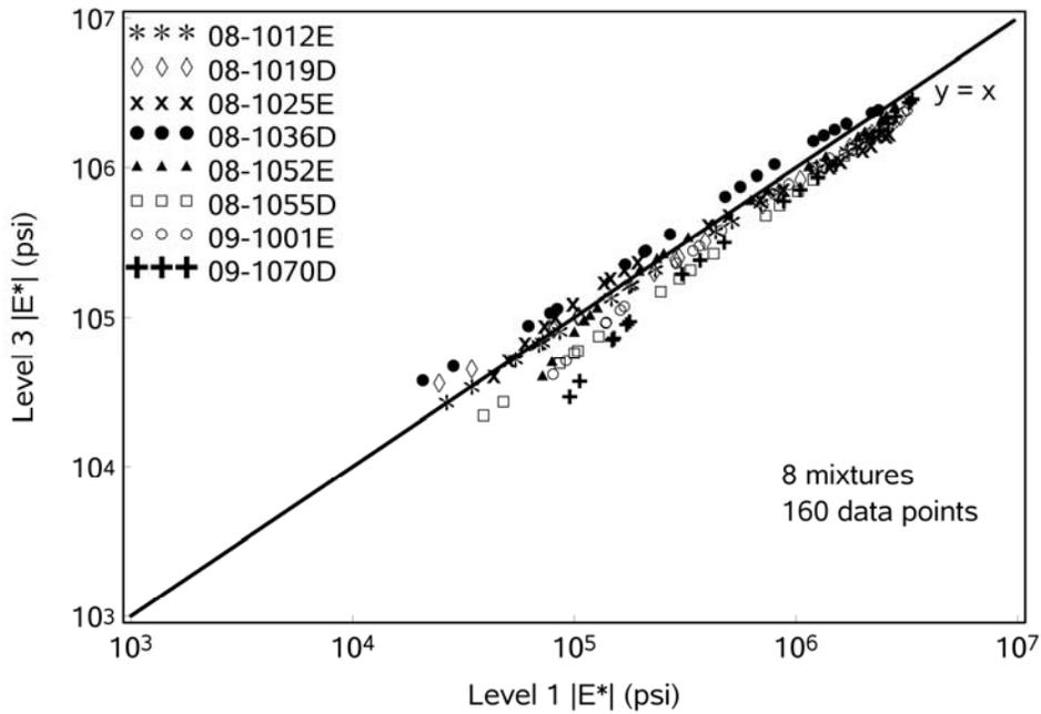
Figure 4. Comparison of Level 1 and Level 3  $|E^*|$  Master Curves for Eight Selected Mixtures
