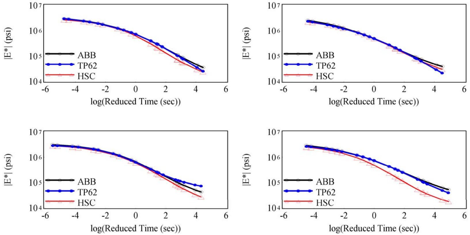
Figure 7. Comparison of ABBREV-Based Master Curve (ABB) with AASHTO TP 62 (TP62) and Hirsch (HSC) Model for Four Selected Mixtures
