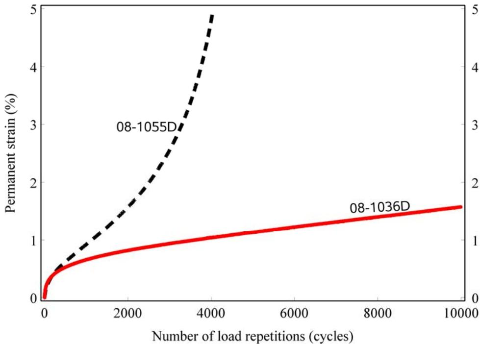
Figure 8. Typical  $\epsilon_p$ -N Results: Two asphalt mixtures with different rutting resistance.
