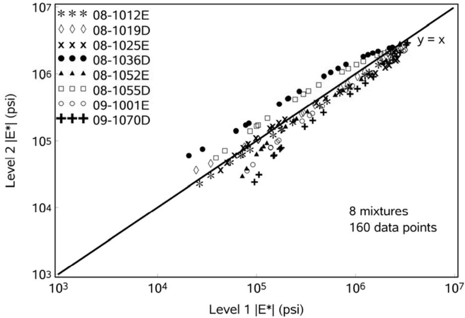
Figure 3. Comparison of Level 1 and Level 2  $|E^*|$  Master Curves for Eight Selected Mixtures
