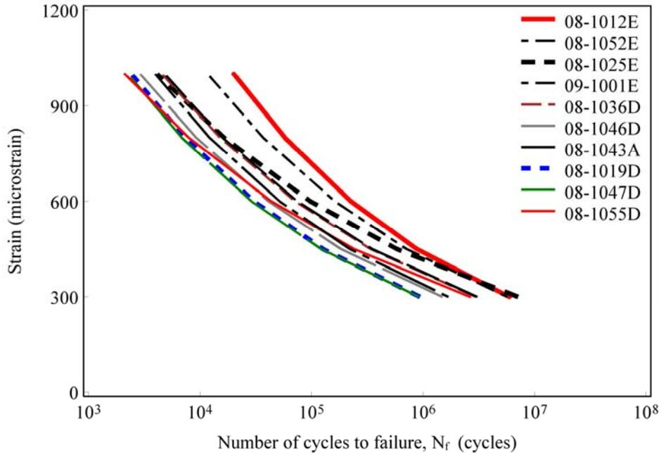
**Figure 11. Fatigue Curves for Virginia Mixtures. Four of the top-performing mixtures in terms of fatigue resistance contained polymer-modified asphalt binders.**
