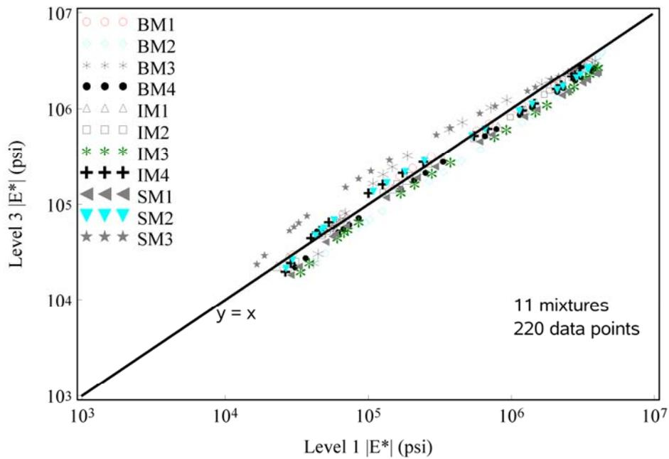
**Figure C2. Comparison of Level 1 and Level 3  $|E^*|$  Master Curves. After Flintsch et al. ( 2007) and Diefenderfer (2010).**
