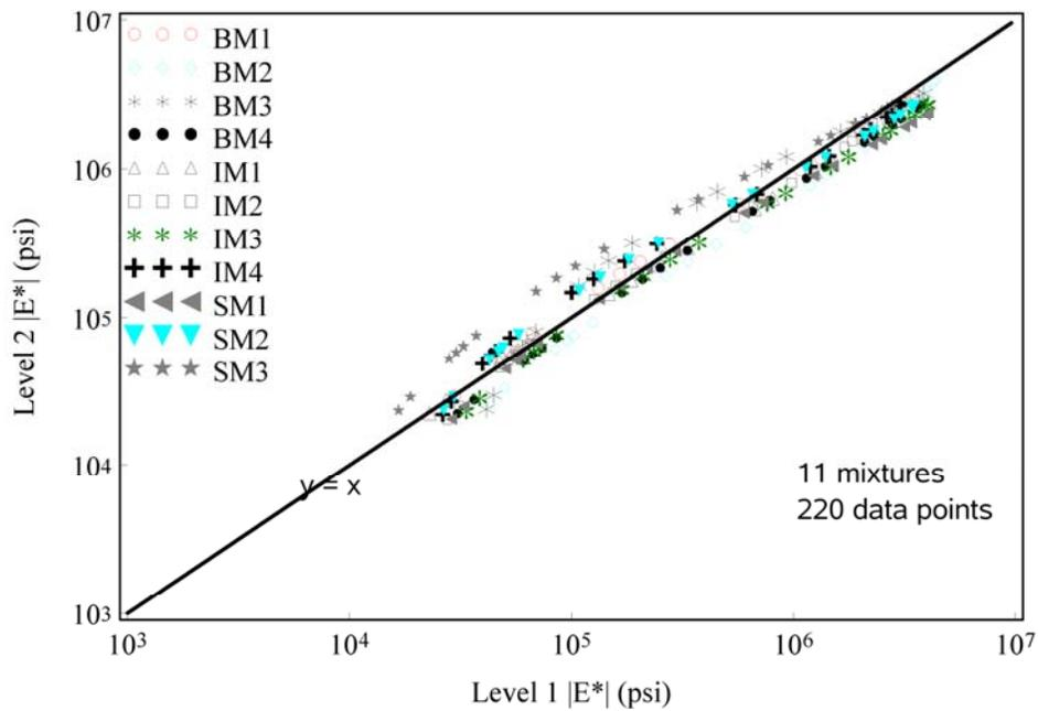
**Figure C1. Comparison of Level 1 and Level 2  $|E^*|$  Master Curves. After Flintsch et al. ( 2007) and Diefenderfer (2010).**
