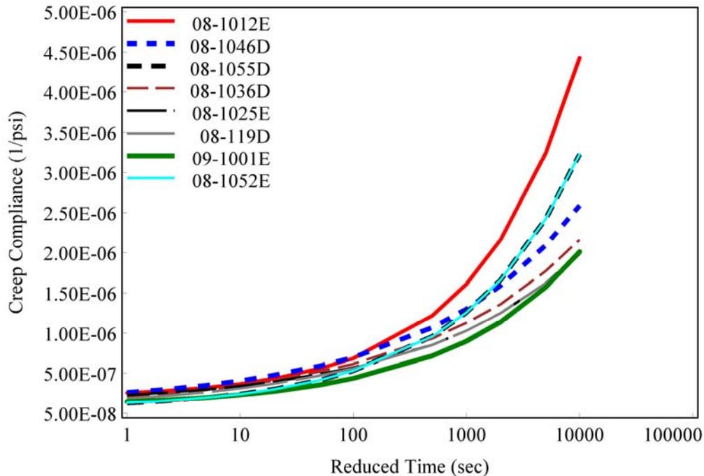
**Figure 9. Creep Compliance Master Curves. Dashed lines = stone-matrix asphalt mixtures, solid lines = surface mixtures.**
