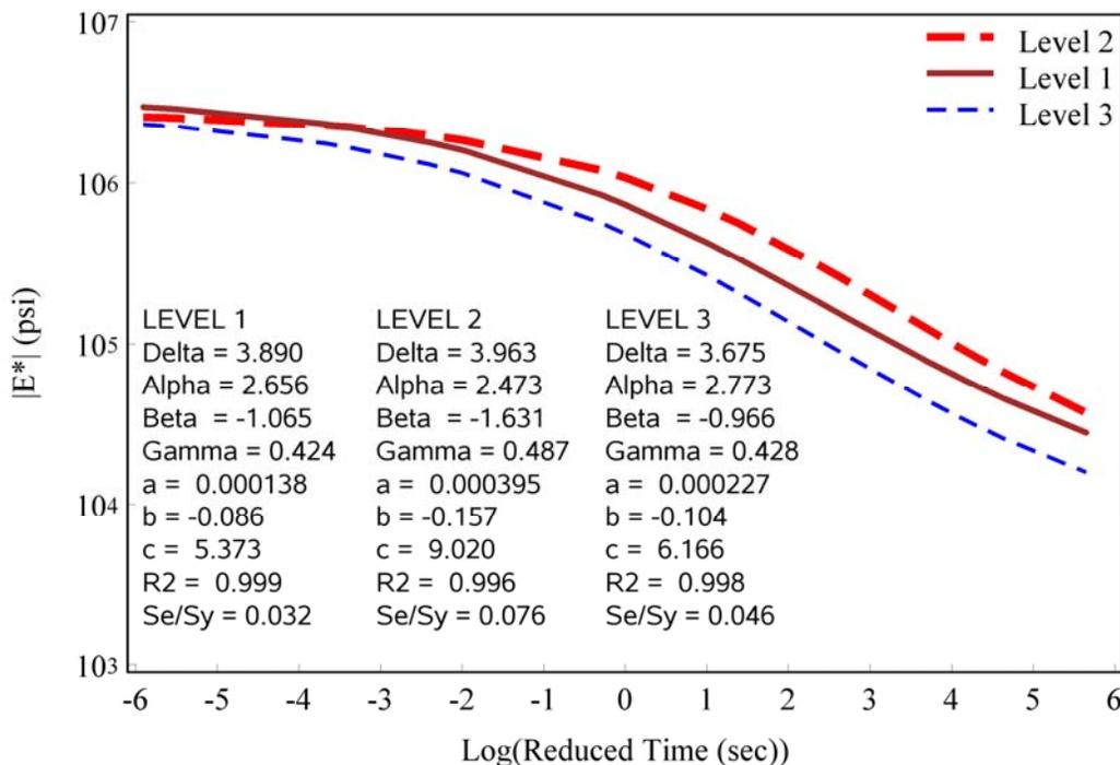
**Figure 2. Comparison of Measured  $|E^*|$  (Level 1) with Predicted  $|E^*|$  at Level 2 and 3 for Mixture 08-1055D.**
