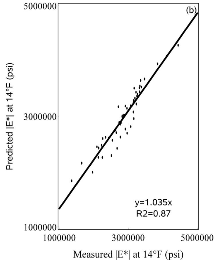
**Figure 6. Comparison of Measured  $|E^*|$  with Predicted  $|E^*|$  Using ABBREV Models for 8 Different Asphalt Mixtures**
