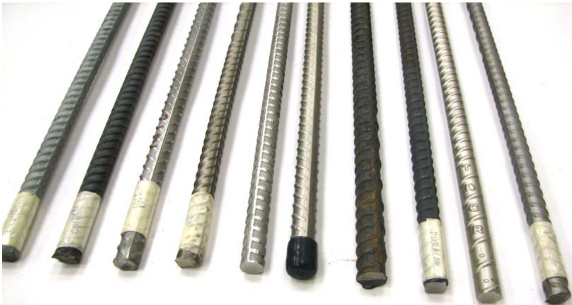
Figure 4. Different types of reinforcing bars that are being offered as being more corrosion resistant than traditional black steel reinforcing bars.
