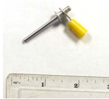
Figure I8. A 3/16" rivet positioned through a ring style solderless connector, which will be used to connect the wires to each rebar specimen
