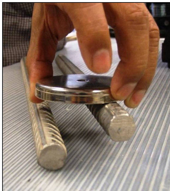
Figure 8. Two bars exposed to magnet: austenitic CRR bar (316LN) on left and duplex CRR bar (2205) on right.
