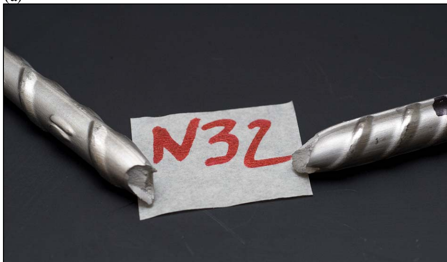
Figure 12. High elongation exhibited by EnduraMet 32. (a) Comparison of untested and tested bar showing stretched rib pattern, and (b) fairly even necking at fracture area.
