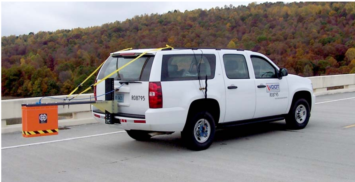
Figure 3. VDOT's Air-Launched GPR System
