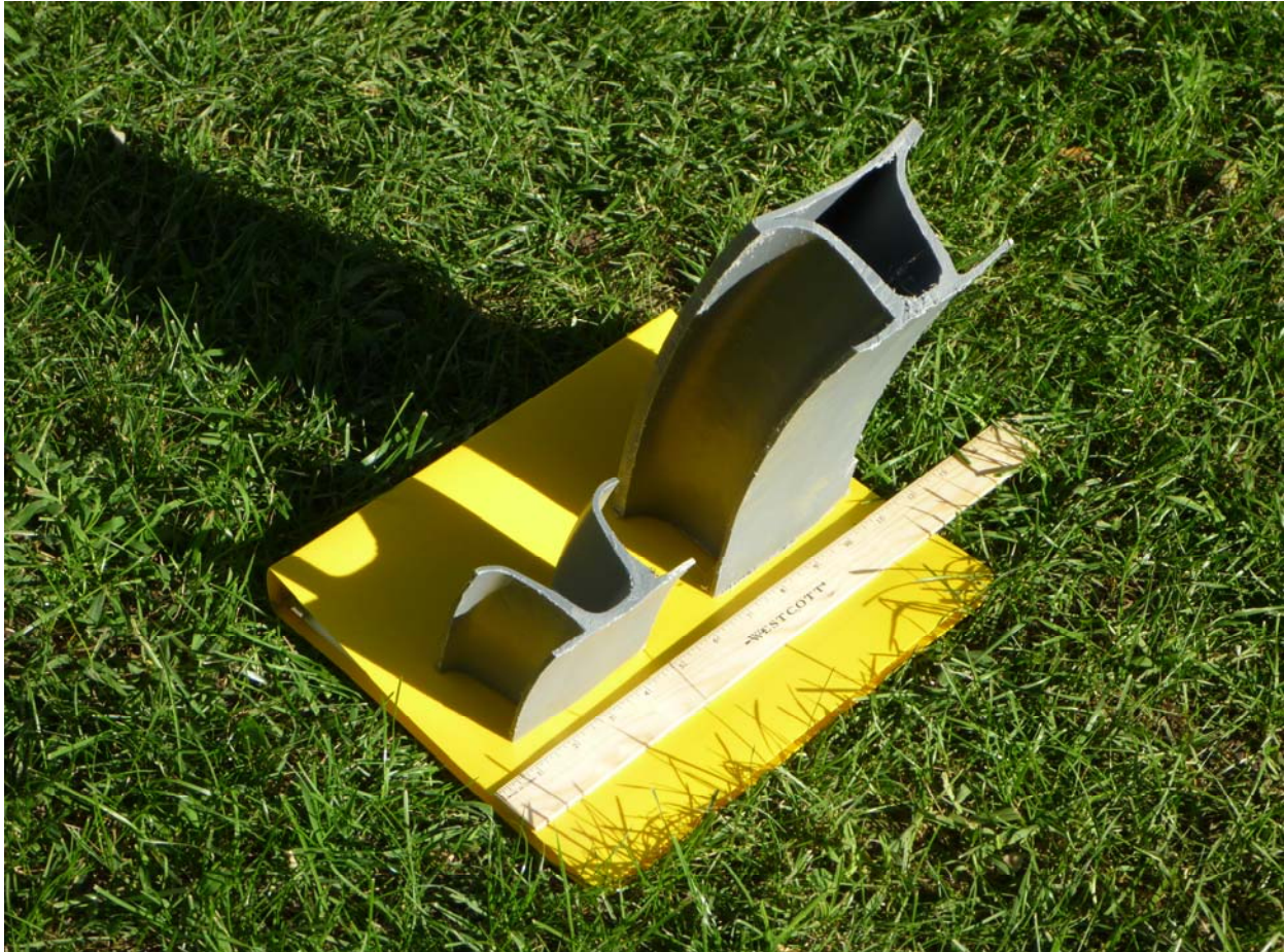
Figure 1. Dual-Wall and Triple-Wall Profiles of ADS Polypropylene Pipes
