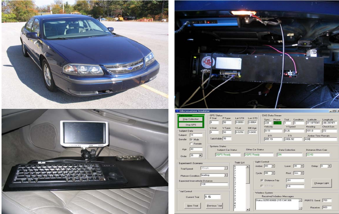
Figure 3. DAS and communication interface in the subject car.
