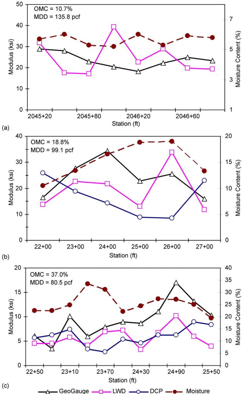
Figure 10. Effect of Moisture on Stiffness Modulus for Subgrade Soil: (a) Route 3, (b) Route 644, (c) Route 743
