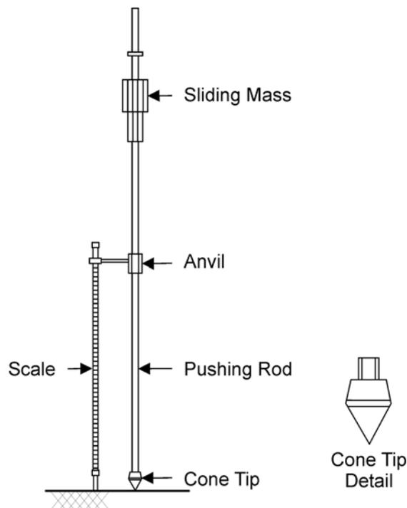
Figure 4. Schematic of Dynamic Cone Penetrometer (after Schmidt, 2008)
