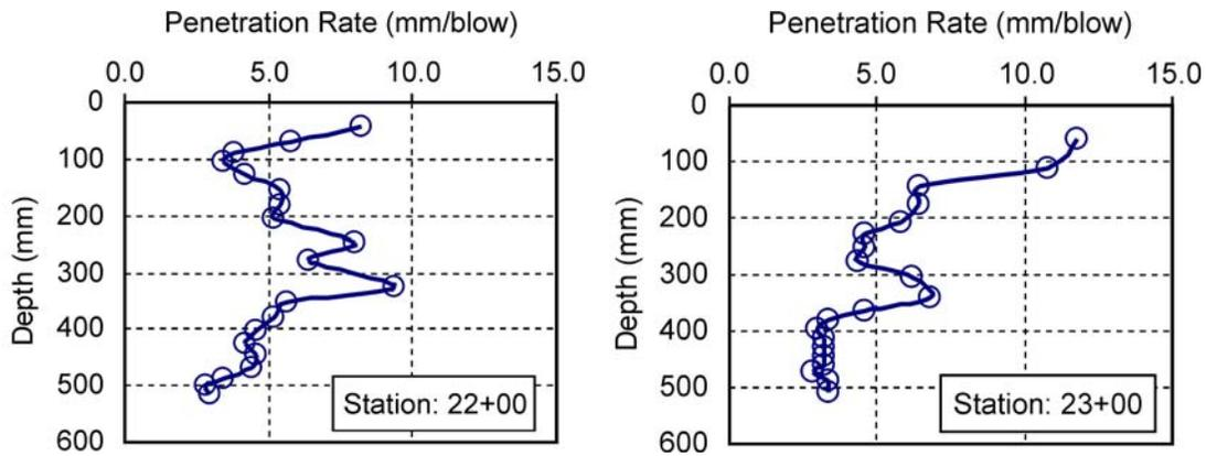
Figure 6. Typical DCP Penetration Rate Versus Depth (Example: Gravel Road on Route 644)
