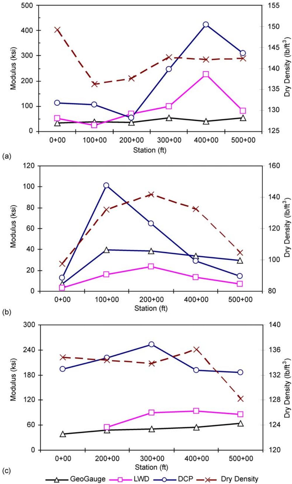
**Figure 8. Comparison of Stiffness Modulus with Dry Density for Gravel Roads: (a) Route 782, (b) Route 785 (c) Route 797**
