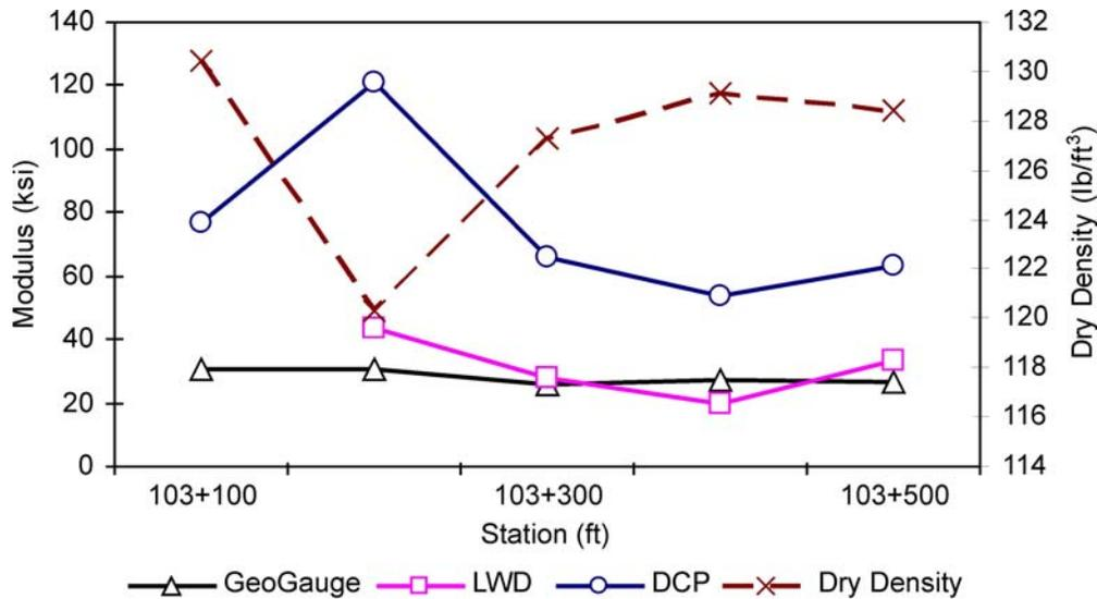
Figure 9. Comparison of Stiffness Modulus with Dry Density for Base Layer on Route 15
