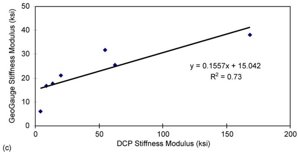
**Figure 13. Comparison of 85th Percentile Stiffness Modulus**
