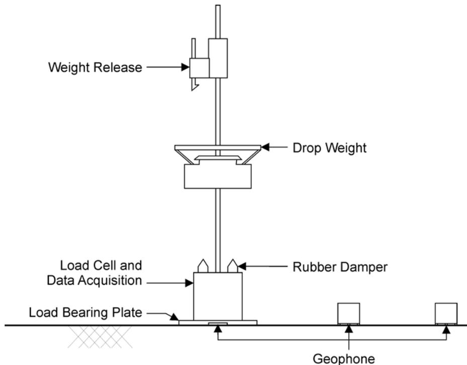
Figure 3. Lightweight Deflectometer
