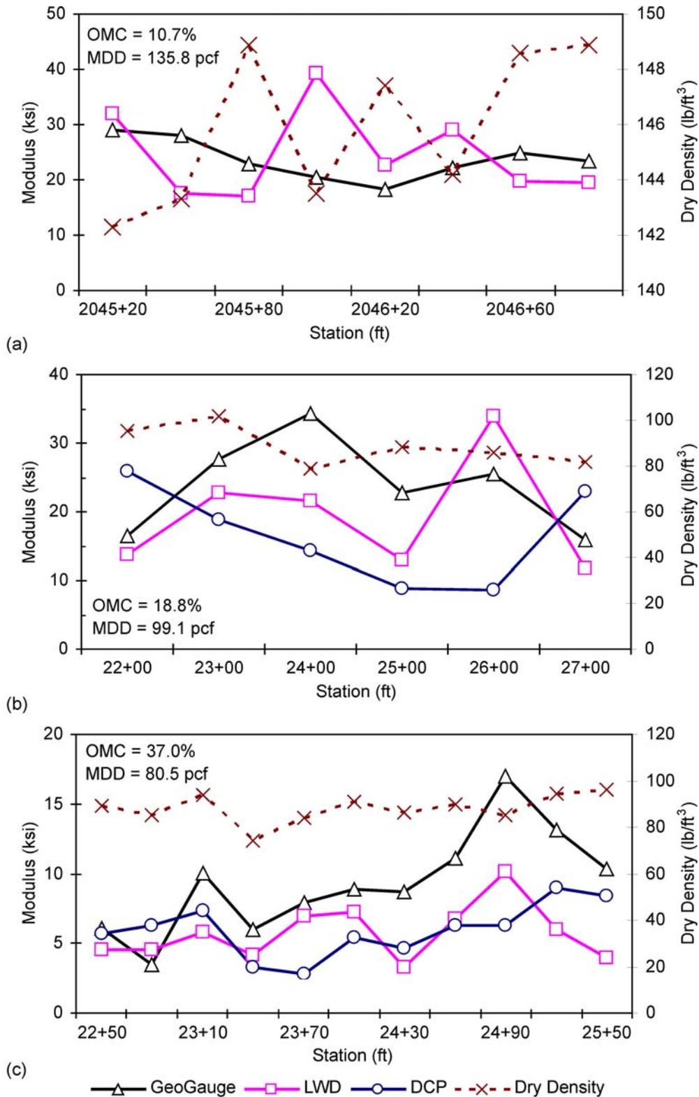
Figure 7. Comparison of Stiffness Modulus with Dry Density for Subgrade Soil: (a) Route 3, (b) Route 644 (c) Route 743
