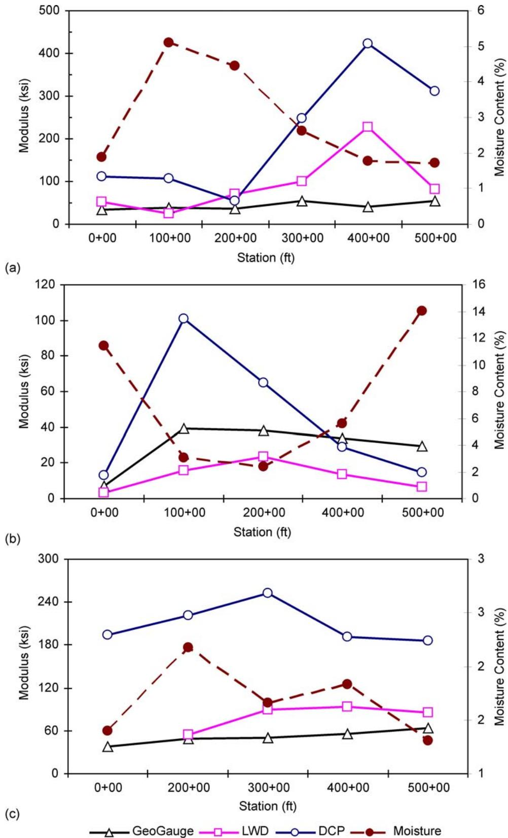
Figure 11. Effect of Moisture on Stiffness Modulus for Gravel Roads: (a) Route 782, (b) Route 785, (c) Route 797
