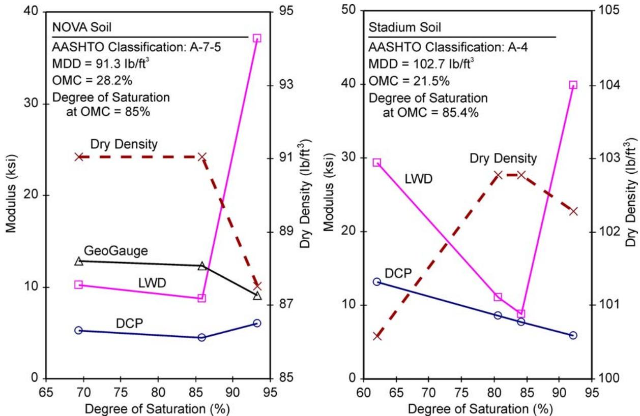
**Figure 14. Effect of Moisture (Degree of Saturation) on Soil Stiffness Modulus in a Laboratory Setup.** NOVA = Northern Virginia; AASHTO = American Association of State Highway and Transportation Officials; MDD = maximum dry density; OMC = optimum moisture content; LWD = lightweight deflectometer; DCP = dynamic core penetrometer.
