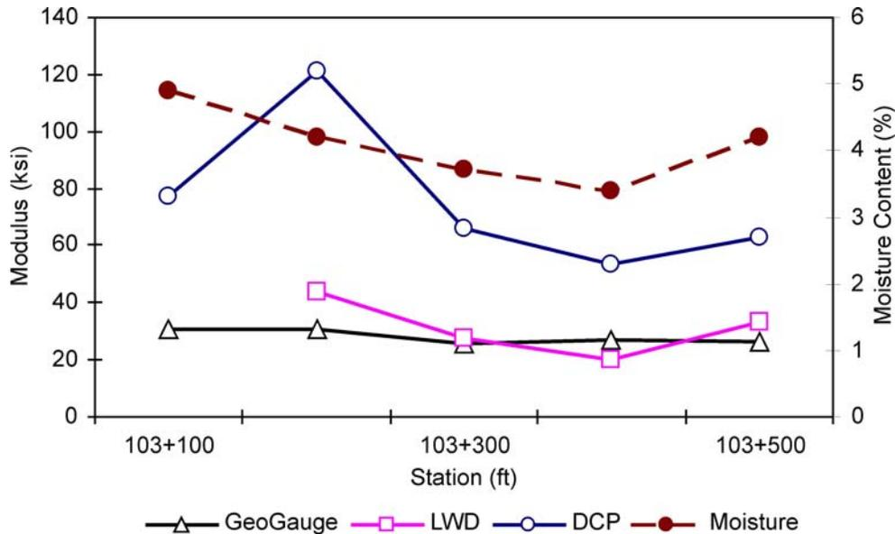
Figure 12. Effect of Moisture on Stiffness Modulus for Base Layer on Route 15
