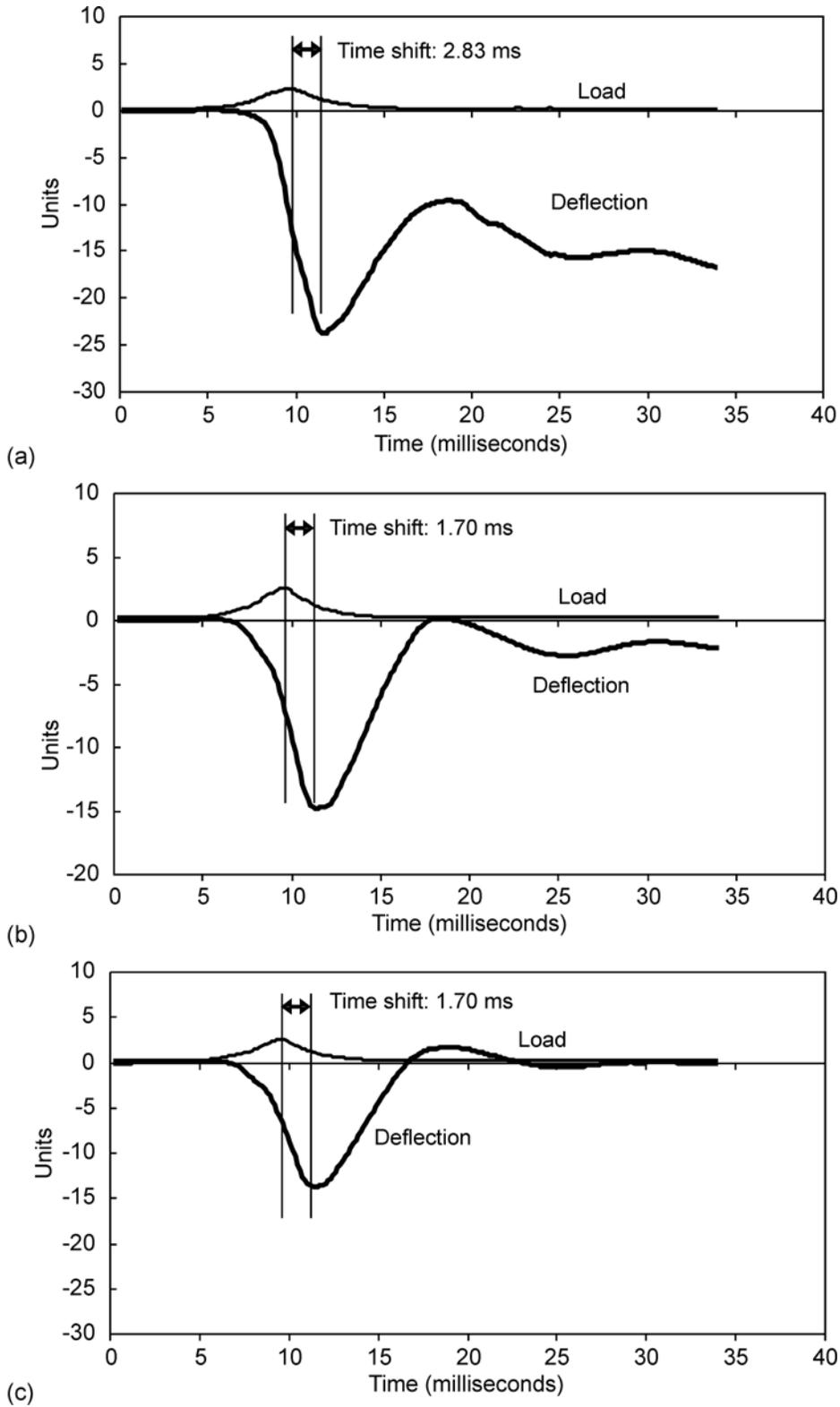
**Figure 5. LWD Output Showing Time Lag Between Load and Deflection Pulses During Consecutive Load Drops: (a) first drop, (b) second drop, (c) third drop**
