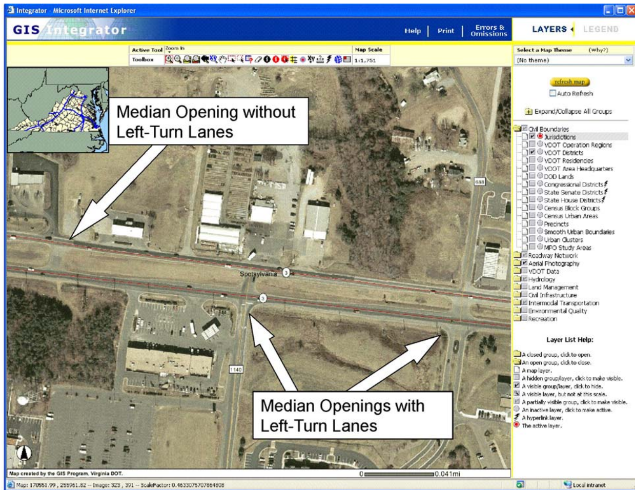
Figure A12. GIS Integrator Aerial Photograph Showing Three Median Openings. The eastern two openings have turn lanes, but the western-most opening does not. The roadway photograph of the western median opening is shown in Figure A13.
