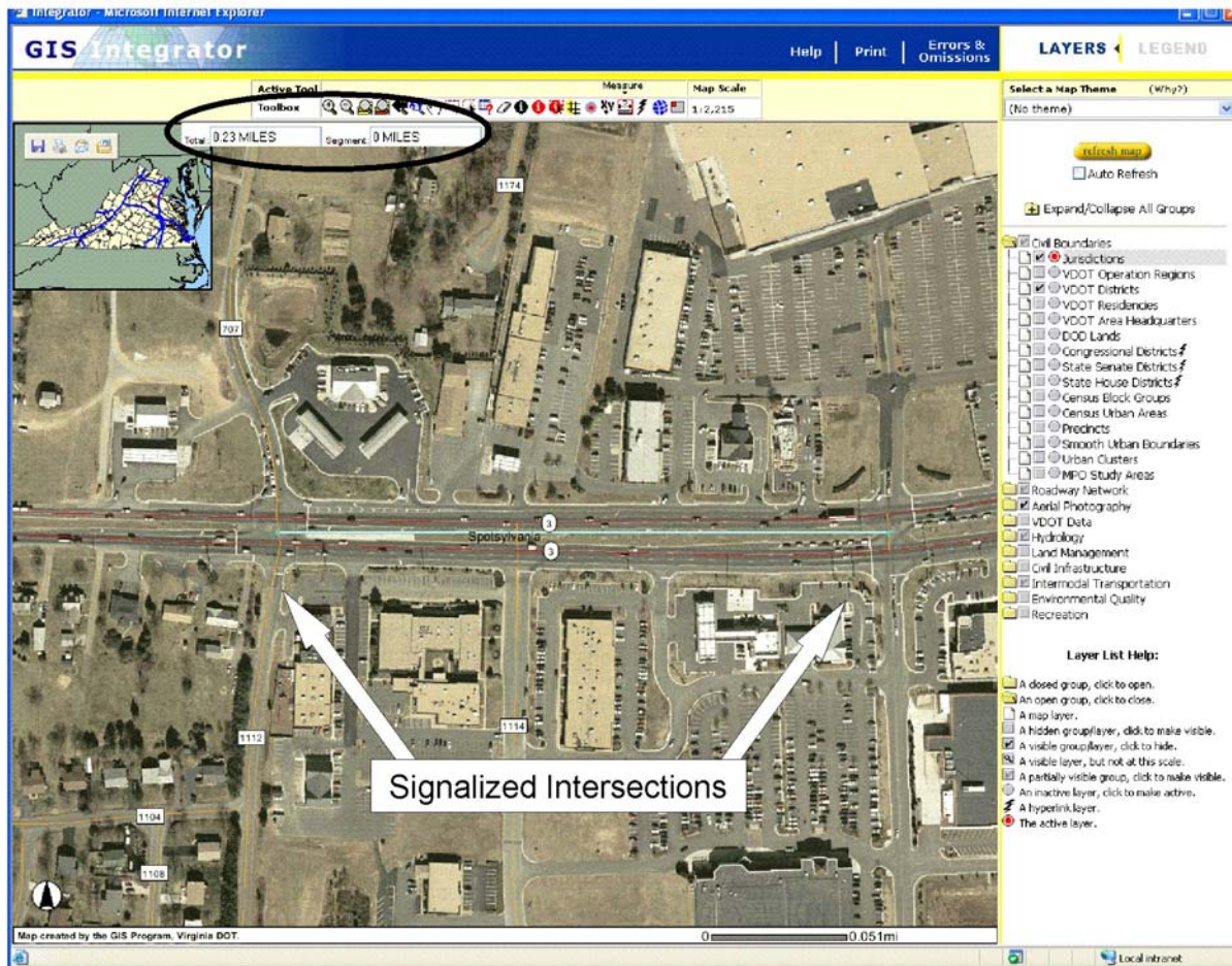
Figure A9. GIS Integrator Aerial Photograph Showing Two Signals. The “Measure” tool was used to determine that the distance between the centerlines of the two signalized intersections is 0.23 mile.
