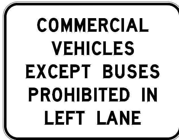
Figure 1. Truck Restriction Sign Used on Interstates with Three or More Directional Lanes
