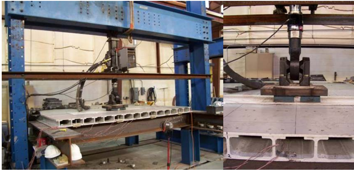
Figure 11. Fatigue test setup at joint 2
