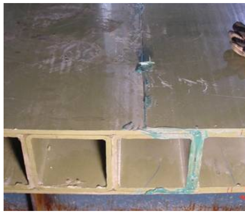
Figure 3. End view of the Strongwell FRP deck
