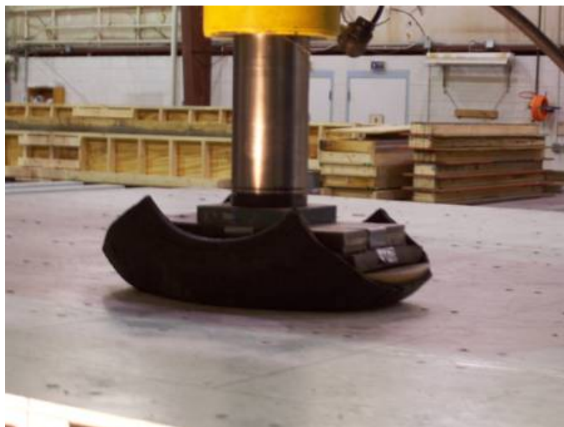
Figure 9. FRP deck loading system
