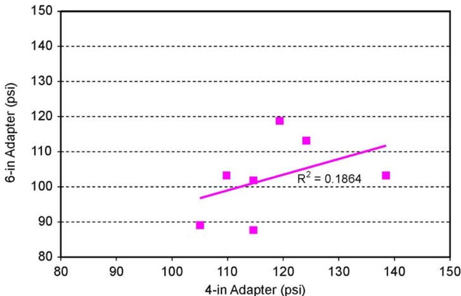
Figure 17. Comparison of Torque-Shear Strength as Measured with the Four-inch and Six-inch Adapters
