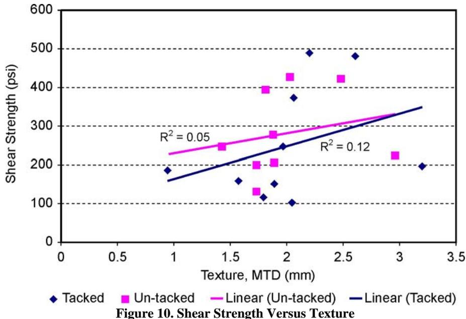
Figure 10. Shear Strength Versus Texture
