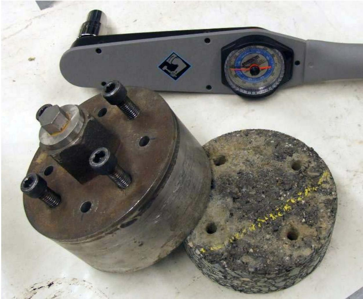
**Figure 7. Torque Wrench, Modified Core Barrel, and Core**
