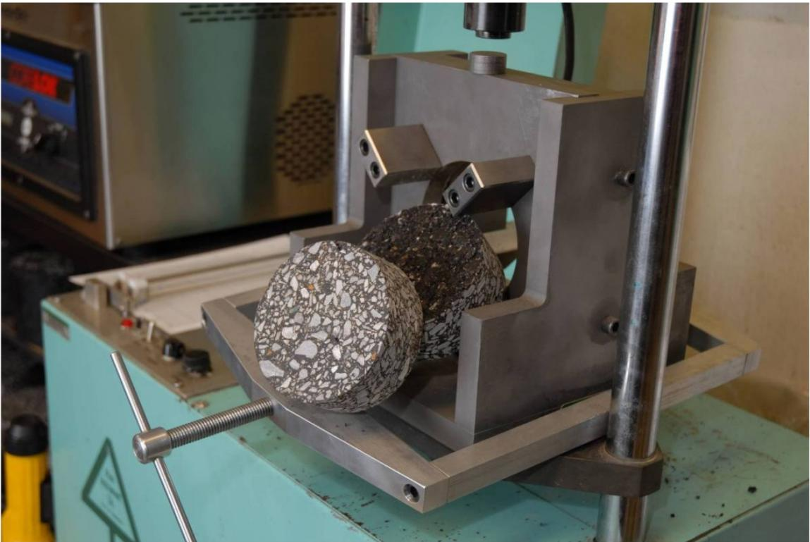
**Figure 3. Guillotine-Style Shear-Testing Adapter for Marshall Device**
