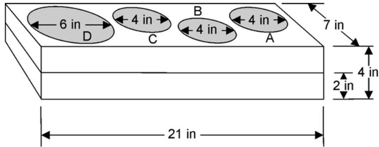
A - Pull Test      C - 4 in Torque Test
