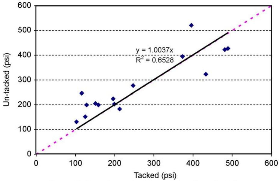
**Figure 13. Shear Strength of Cores Taken From Field Projects**
