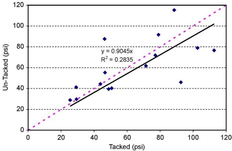
**Figure 14. Tensile Strength of Cores Taken From Field Projects**
