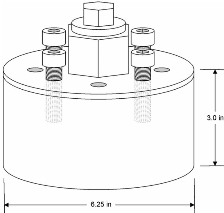
**Figure 6. Six-inch Torque Adapter (Component 1) of the Torque-Shear Device**
