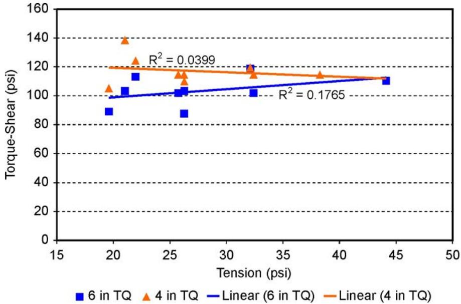
Figure 15. Comparison of Results of Tests with Torque-Shear Device and Simple Tensile Strength Tests
