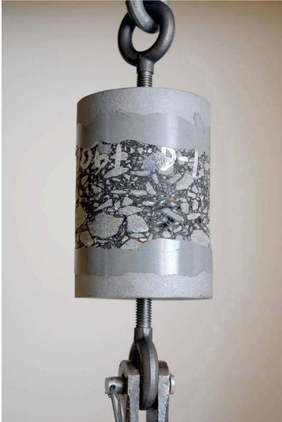
**Figure 4. Specimen Ready for Tension Test**
