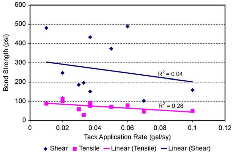
Figure 12. Bond Strength Versus Tack Application Rate
