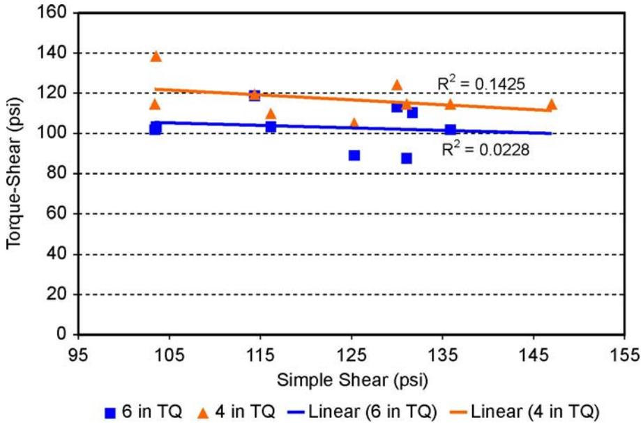
Figure 16. Comparison of Results of Tests with Torque-Shear Device and Simple Shear Strength Tests
