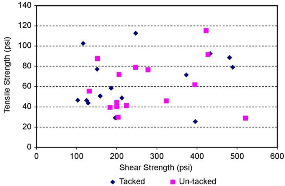
Figure 9. Shear Versus Tensile Strength for Field Cores
