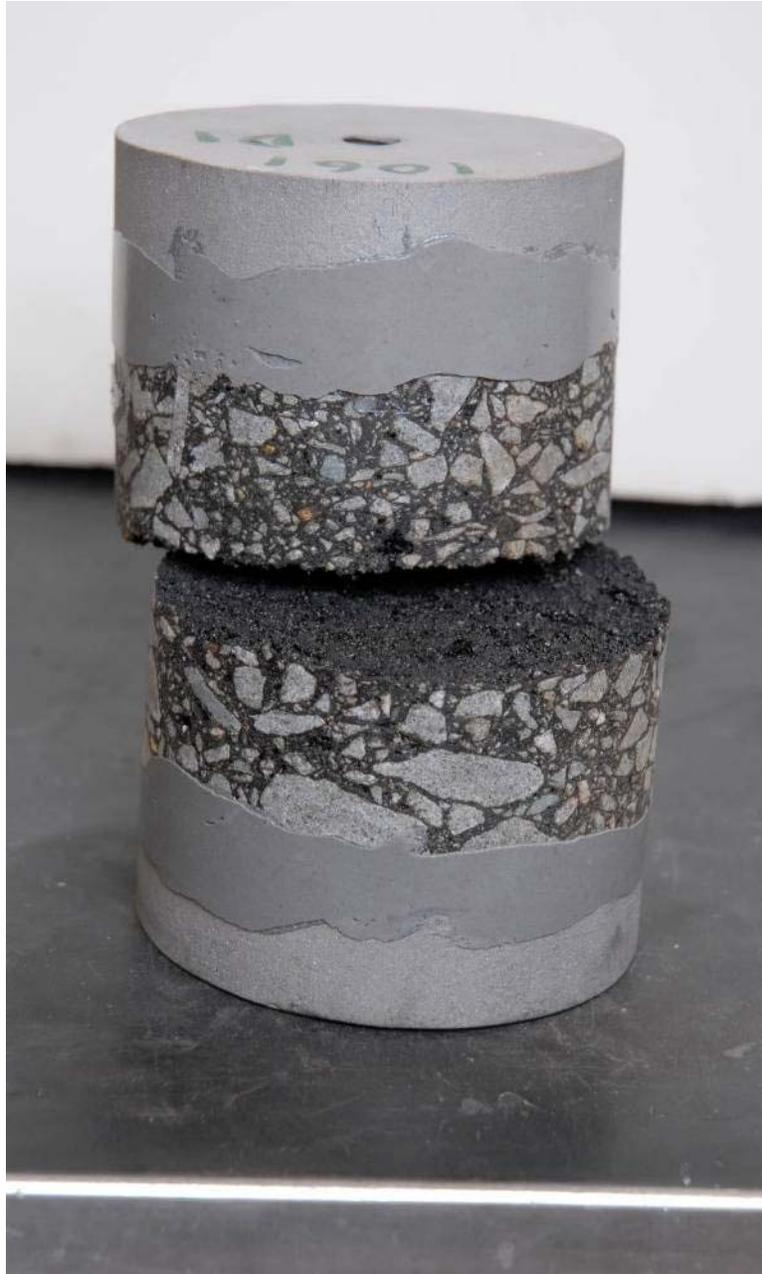
**Figure 5. Specimen After Tension Test**
