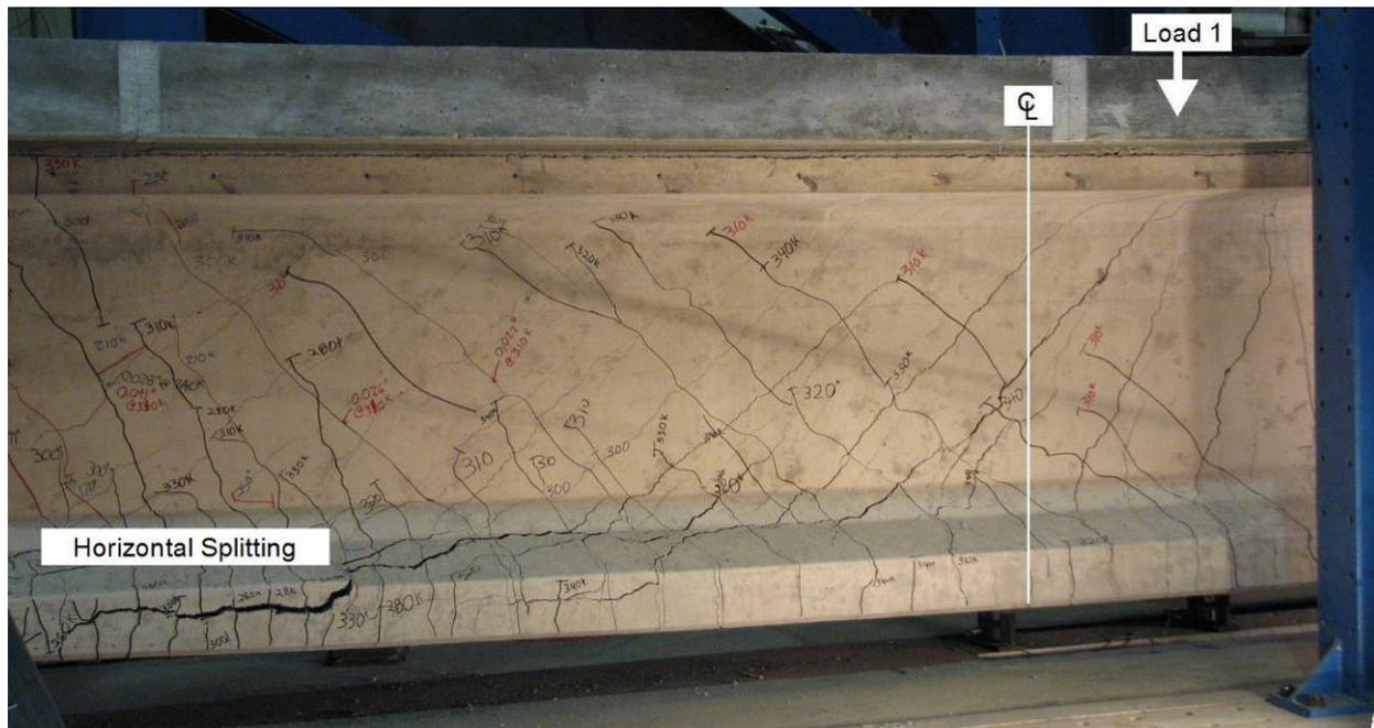
**Figure 51. Horizontal bottom flange splitting failure**
