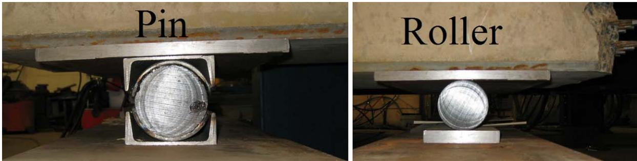
Figure 13. Beam end support conditions
