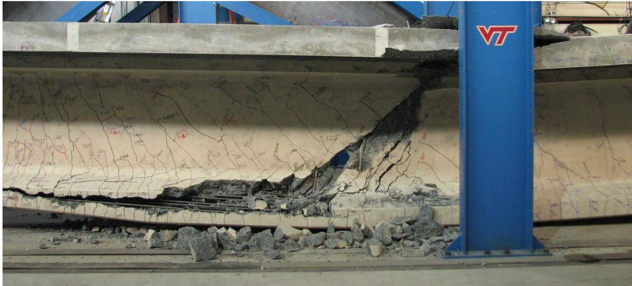
**Figure 55. Ultimate failure of the PCBT-53**
