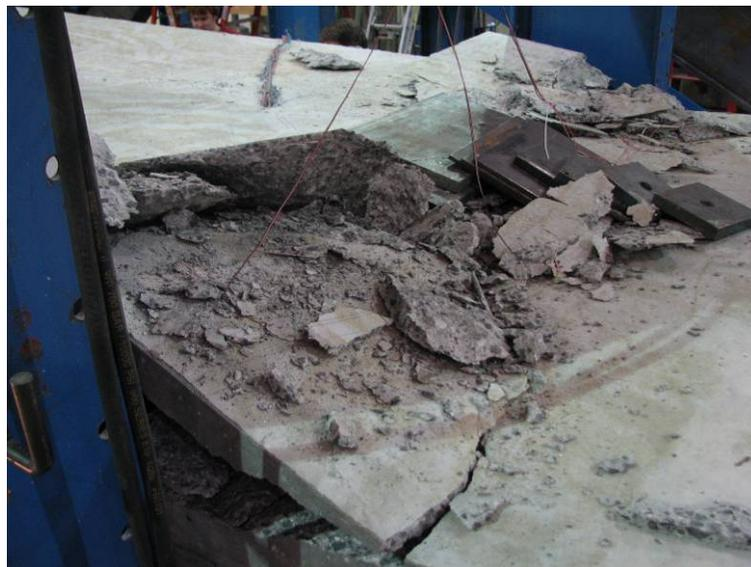
**Figure 56. Crushing in the top of the deck**
